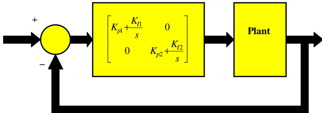
Figure 7.4: Structure of the liquid level control system showing the two-input two-output diagonal form of proportional plus integral controller.
