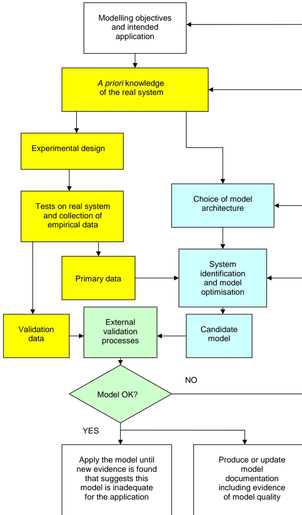
Figure 9.1: Block diagram of iterative processes of model development showing from formulation of modelling objectives to external validation and testing of model adequacy.
