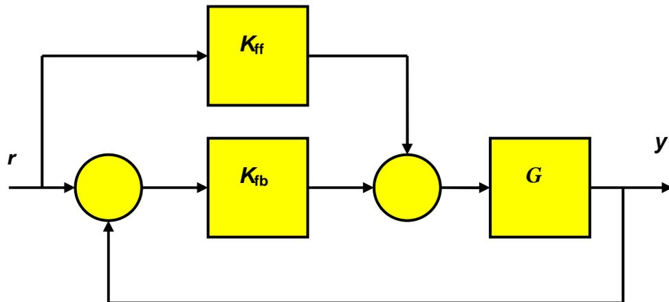
Figure 6.1: Block diagram of model-following control system based on the two degrees-of-freedom approach involving a feed-forward controller  $K_{ff}$  and a feedback controller  $K_{fb}$ .
