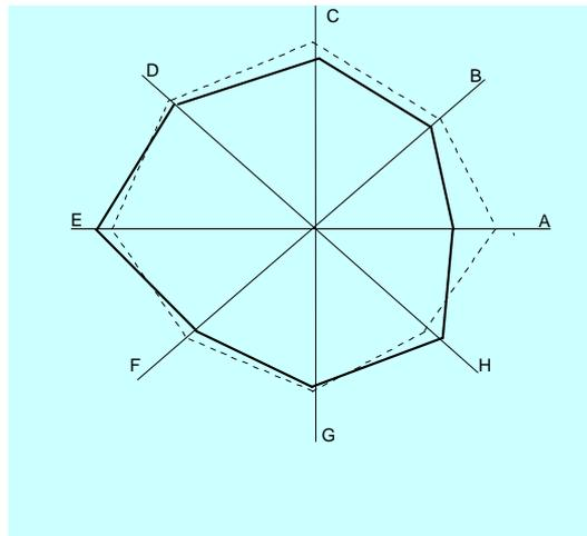
Figure 4.1. Example of polygon representation for model validation results. Here solid lines represent modelled results for eight different quantities while the dashed lines indicate the corresponding measured values. (Adapted from diagram in (Smith, Murray-Smith & Hickman, 2007b - **submitted paper, [67]**).
