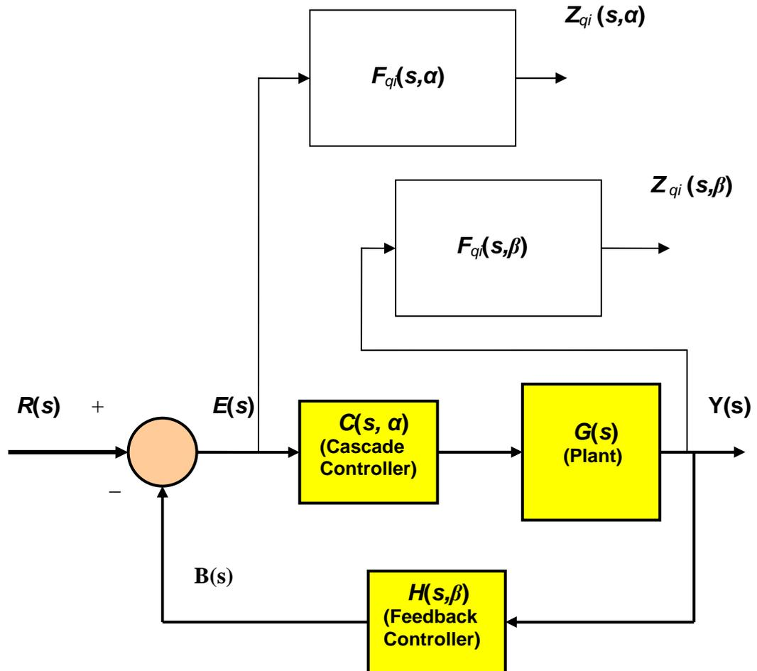
Figure 7.2: Block diagram for single-input single-output case showing method of generation of the sensitivity signals for one parameter of the cascade controller and one parameter of the feedback controller. Additional parameters can be handled by introducing extra sensitivity filters in parallel with each of the two sensitivity filters shown in this diagram.
