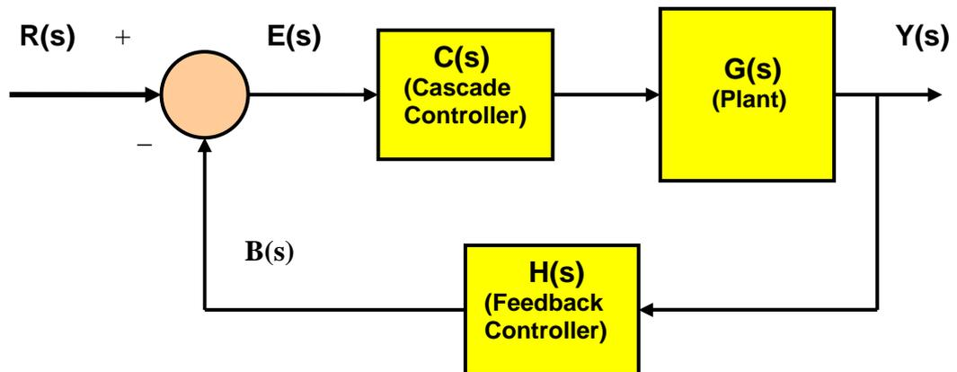
Figure 7.1: Block diagram of single-input single-output system with cascade and feedback controllers, where  $R(s)$  represents the Laplace transform of the reference input  $r(t)$  and  $Y(s)$  represents the Laplace transform of the system output  $y(t)$ . The variables  $e(t)$  and  $b(t)$  correspond to the transformed variables  $E(s)$  and  $B(s)$  shown on the diagram.
