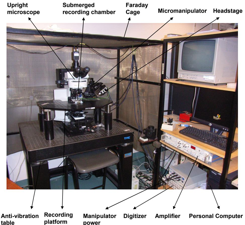
**Figure 2-2** Photograph showing the actual setup used in patch-clamp experiments.
