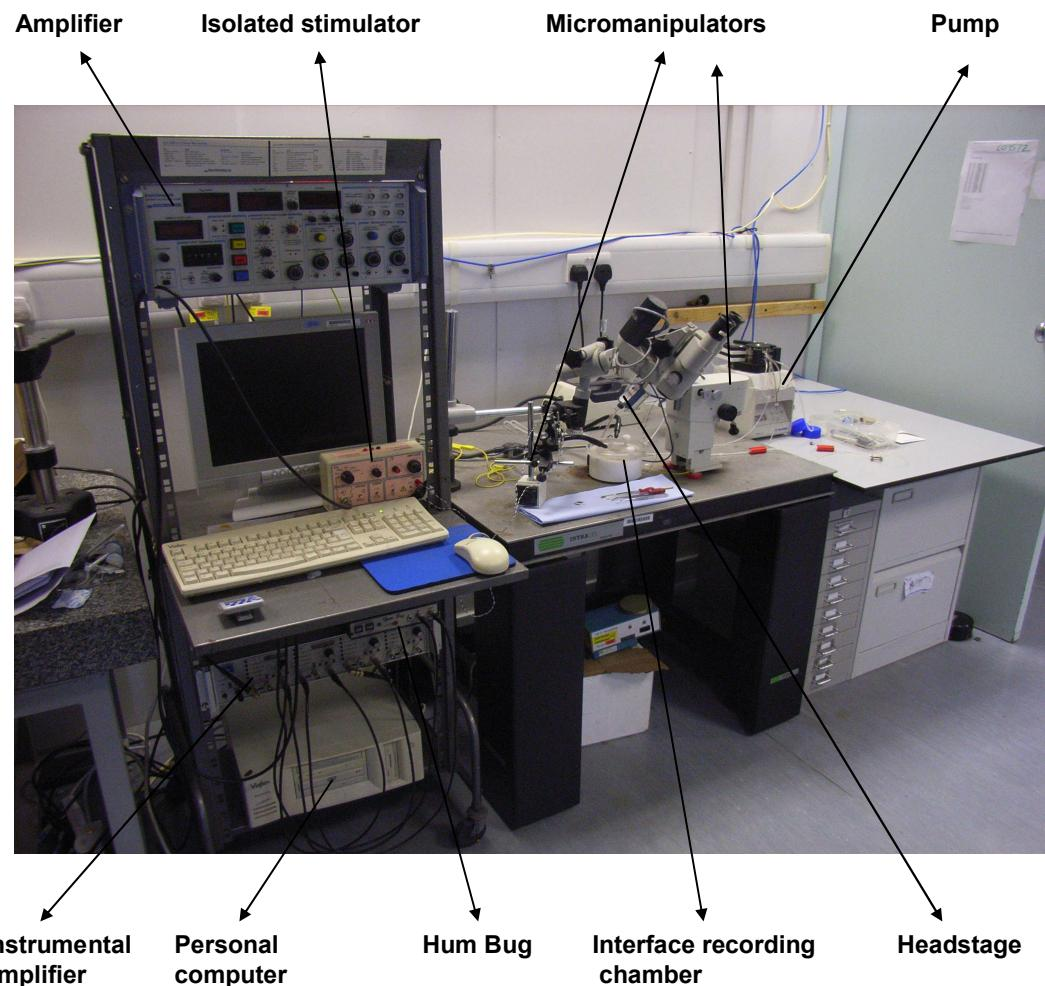
**Figure 2-4** Photograph showing the actual setup used in extracellular recording experiments.
