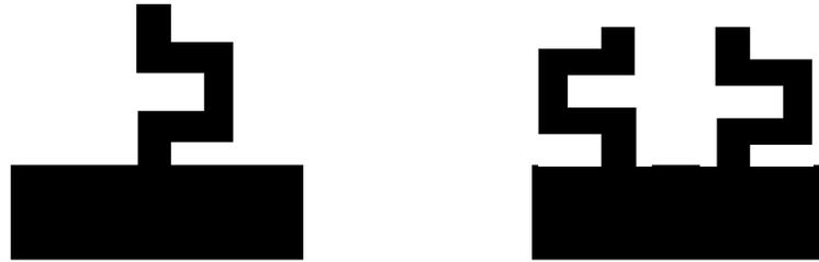
b) Cantilever beam with meandered suspensions
