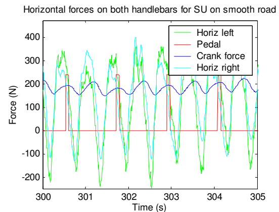
Figure 5-45: Horizontal force on the both handlebars for the fully suspended bike on the rolling road rig on a smooth surface.
