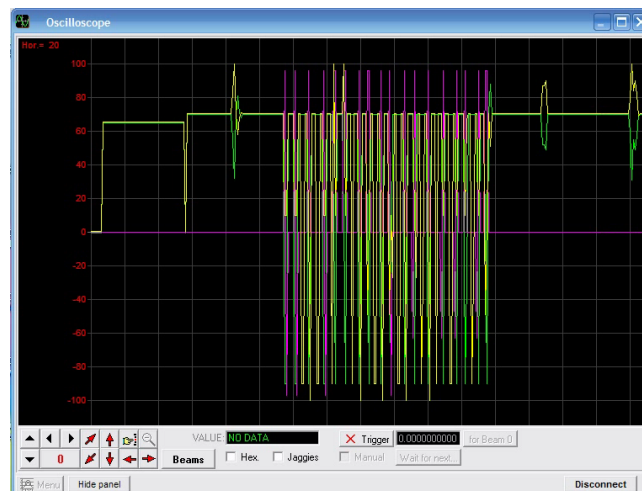
Figure 5.25: The bluetooth logger developed for windows. It has an interface similar to an oscilloscope. It logs the signal of interest. In this case the energy and the motor outputs.
