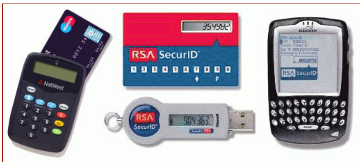
Figure 2-5: Different types of tokens used to generate one-time pin (OTP) numbers
