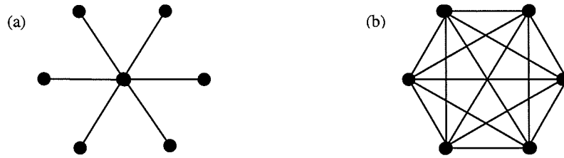
Figure A.4a and A.4b The number of necessary links with (b) and without (a) a common switching point.
