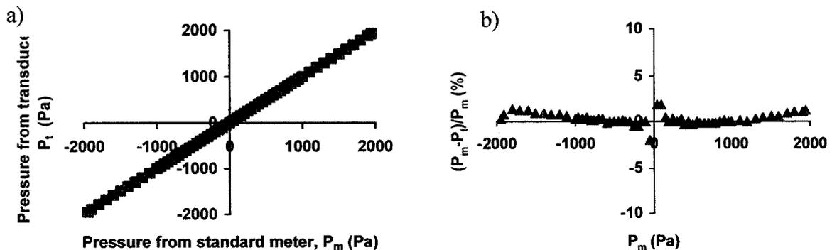
**Figure A1.2. Plot demonstrating linearity of the pneumotachograph used to measure flow in the FOT device.**
