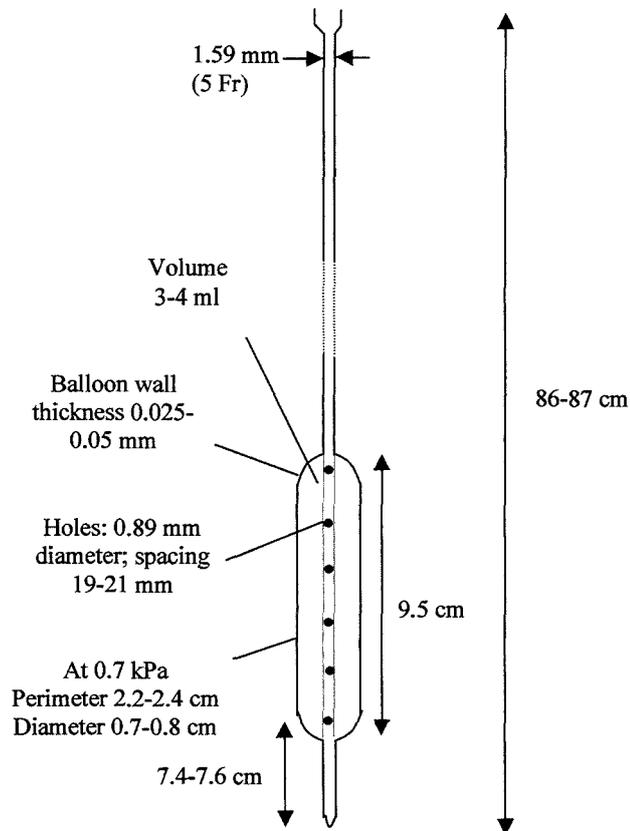
**Figure 1.3.3. Working volume of the oesophageal balloon catheter.**
