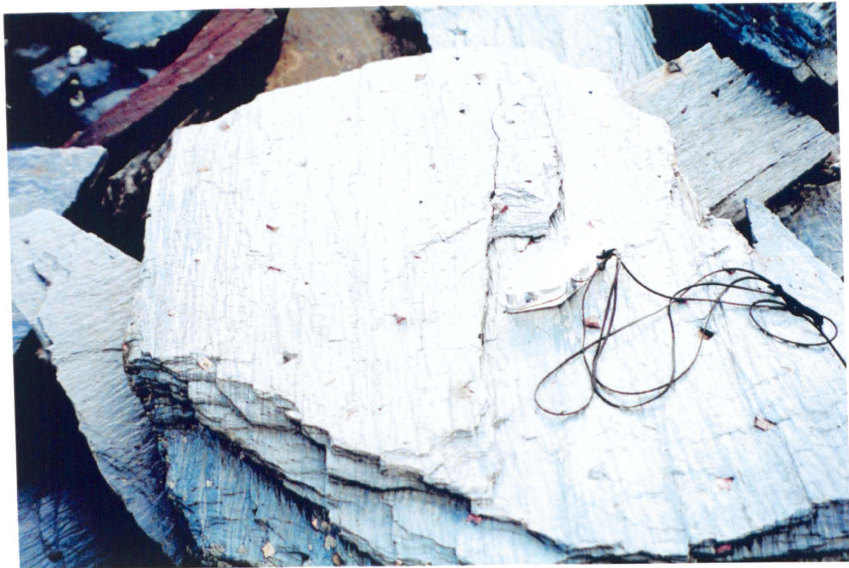
Plate 15 Easdale slate showing the crenulation cleavage. Pyrites show little deterioration after more than 50 years of weathering.
