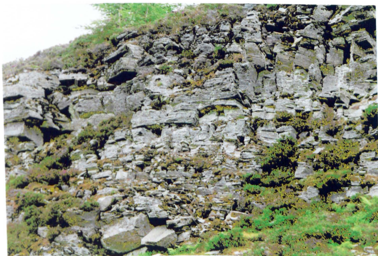
Plate 40 Kirkney Quarry near Huntly. The overhanging face has collapsed with time along the pillaring line. (NJ 503317 to 510320)
