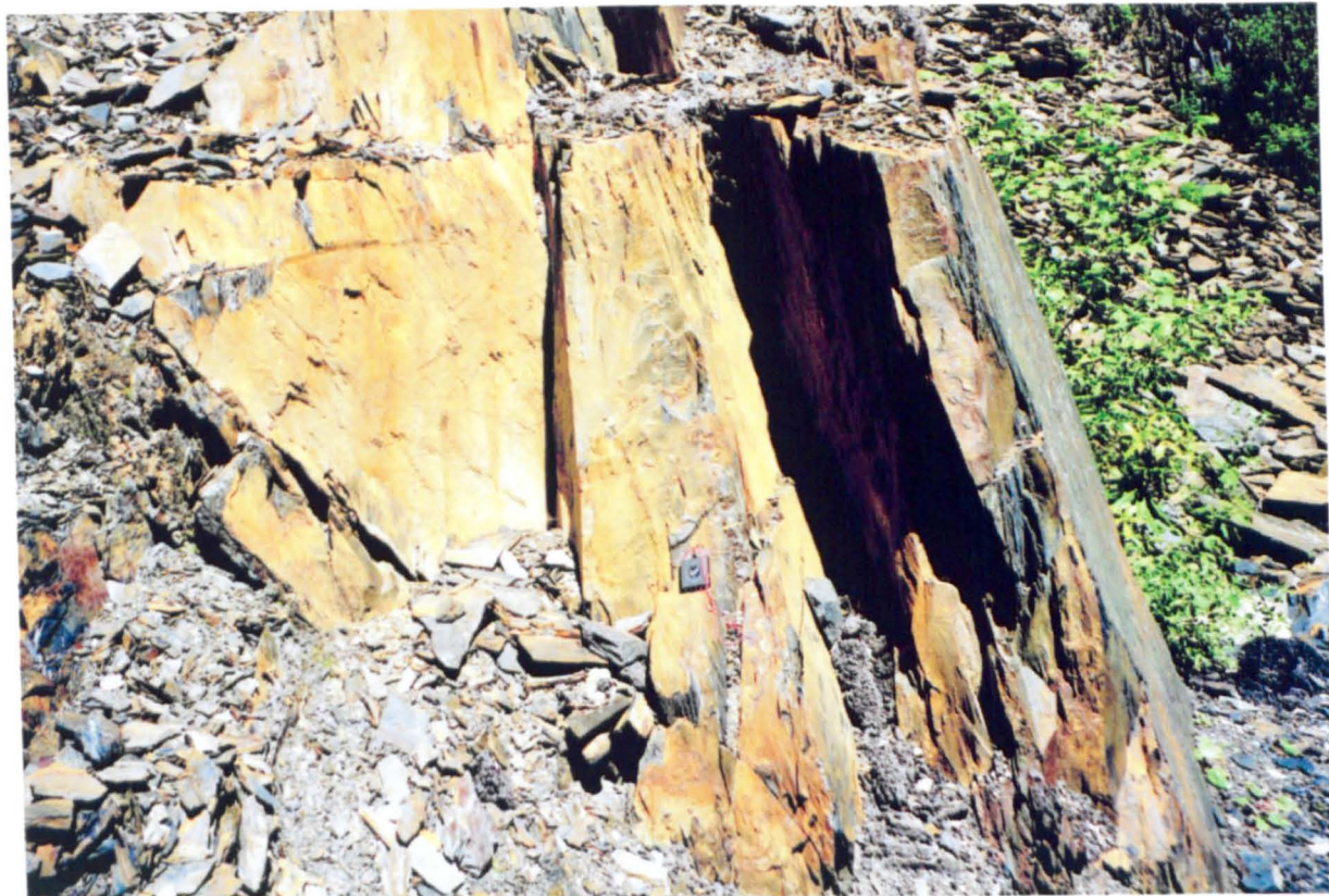
Plate 9 North Ballachulish - West Quarry showing the intense weathering of the pyrrhotites.
