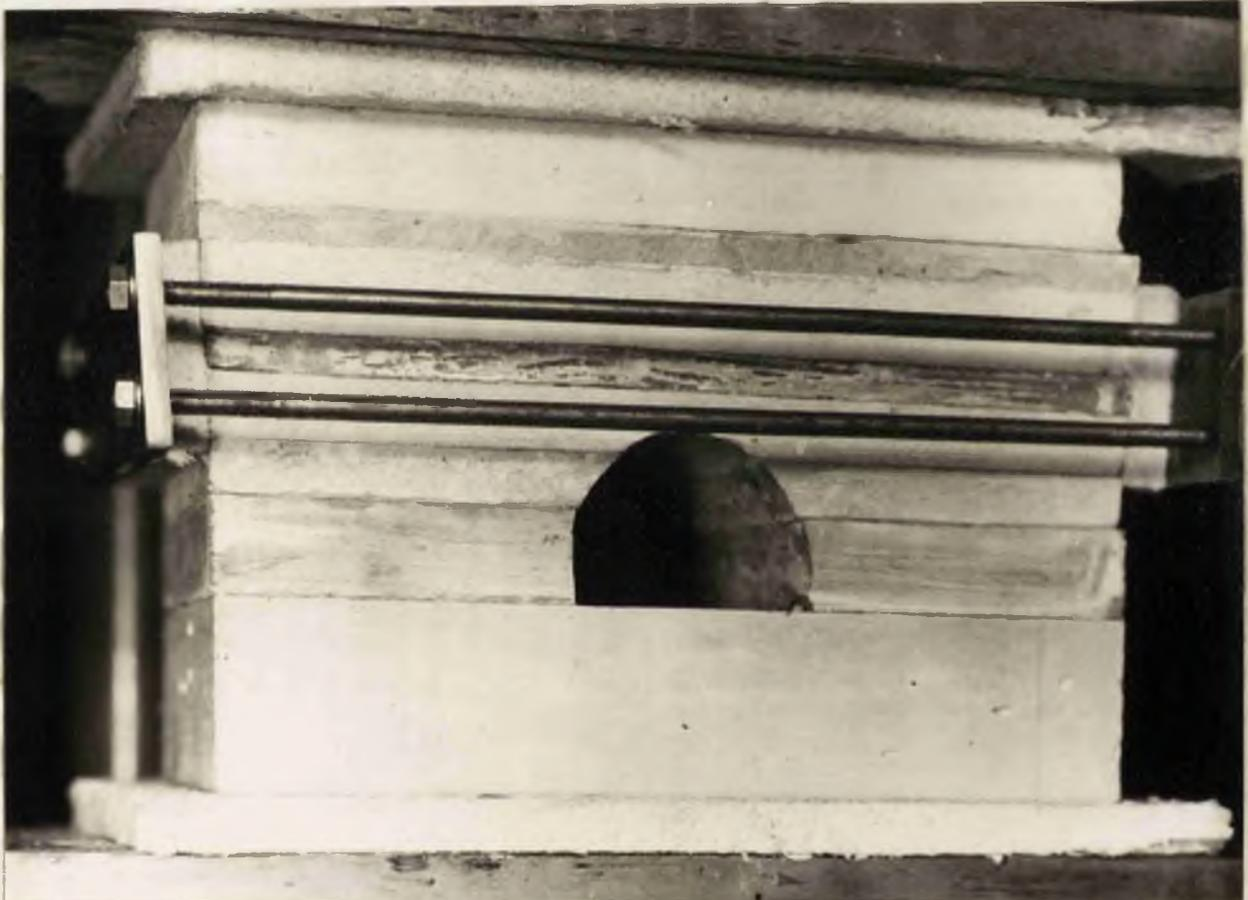
The model fitted with the horizontal retaining frame prior to applying the vertical load. The various thicknesses of strata are clearly seen as well as the fibre boarding between the model and the machine platens to prevent localised regions of high stress.
