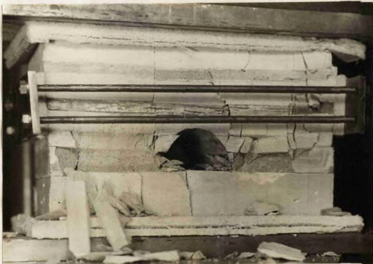
Applied load 485 lb./in.<sup>2</sup>. The roadsides have now failed completely and deformation of the model continued without further increase in the applied load.
