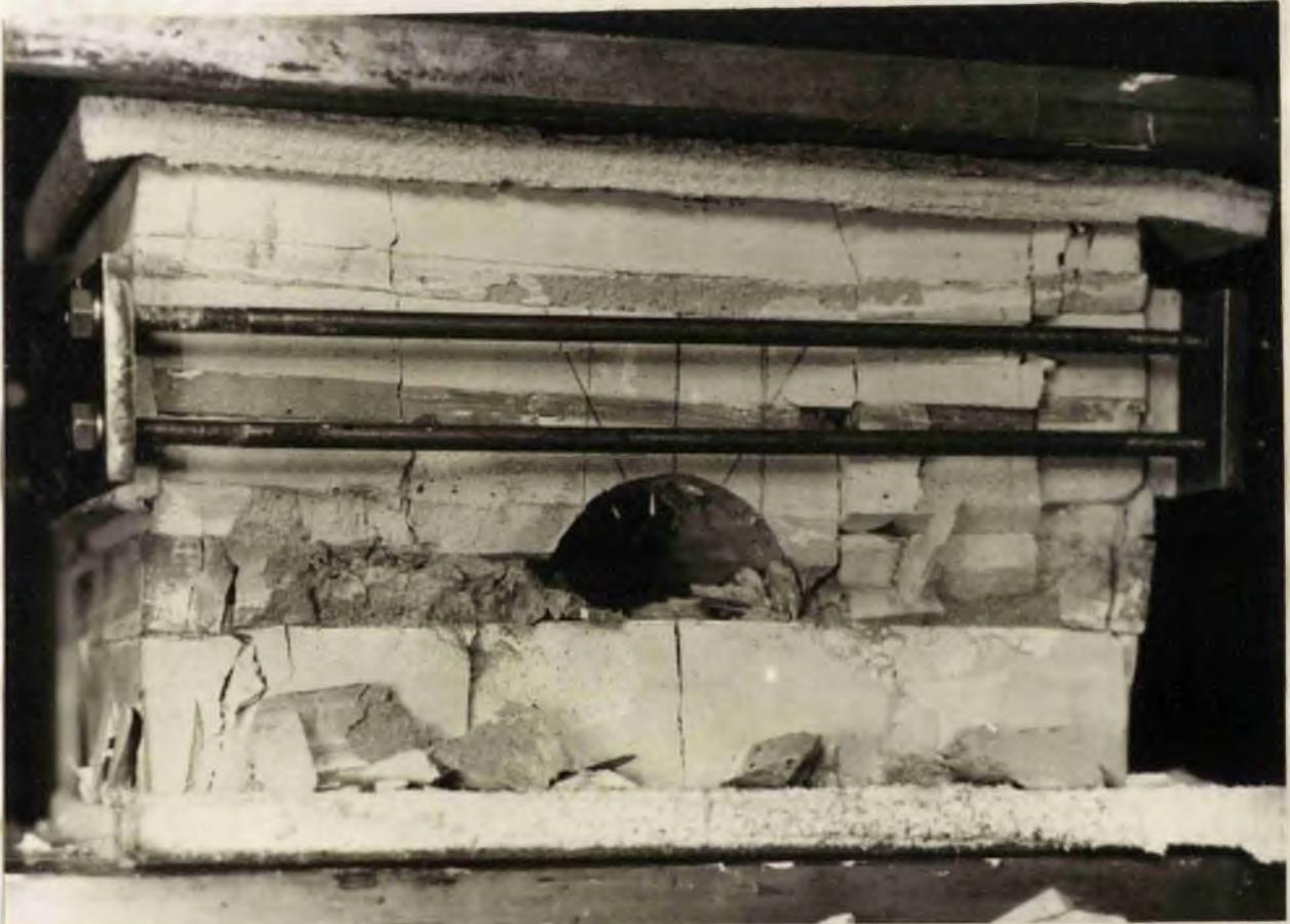
Applied load 425 lb./in.<sup>2</sup>. The roadside packs disintegrated completely but no bed separation or collapse of the bolted strata became visible.
