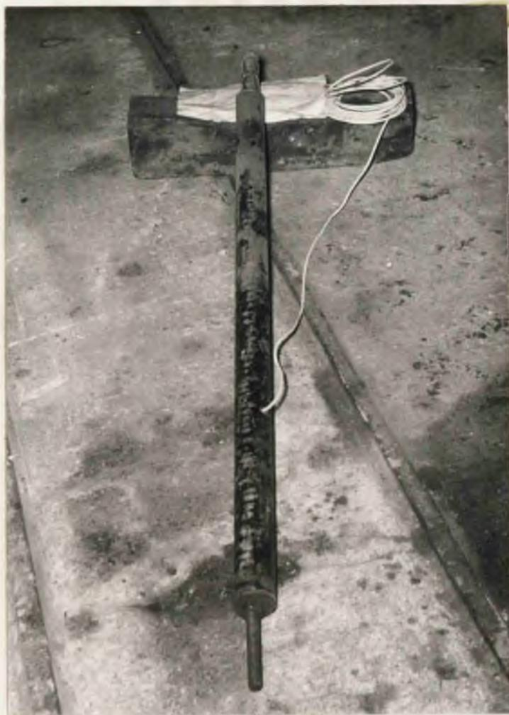
Control Bolt to Check Drift of Gauges
