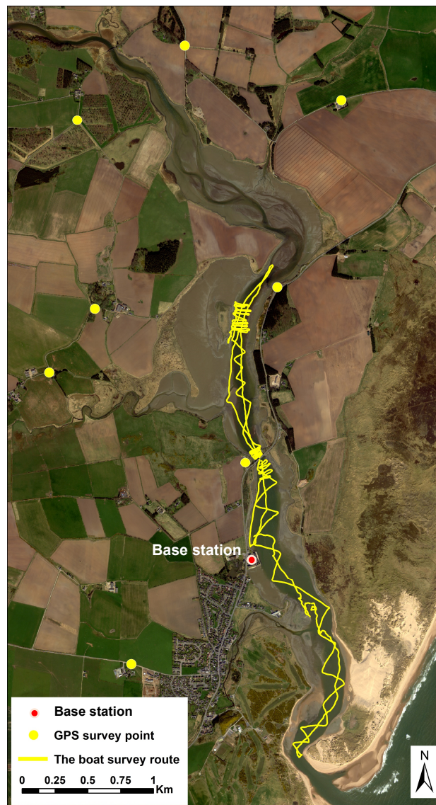
Figure 2-11: The bathymetric survey routes in the main channel of the estuary conducted on 10/09/2015, and GPS validation point locations.
