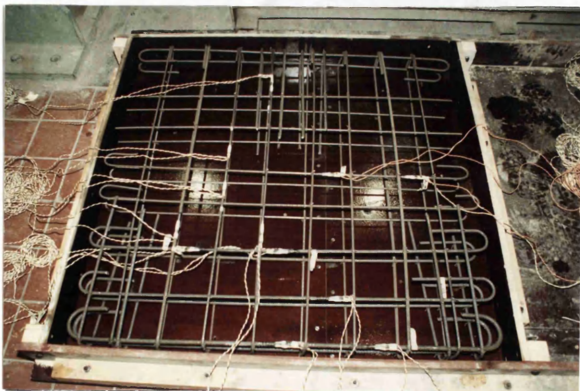
Fig. 6.9b Steel Layout - Beam Model
