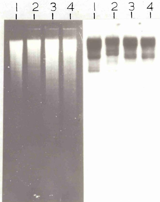
Figure 8.6. Southern blot analysis of A.nidulans and A.niger DNA using a v-ras probe.
