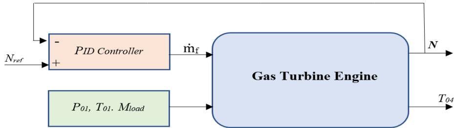
Figure 4.3: Schematic diagram of gas turbine control system
