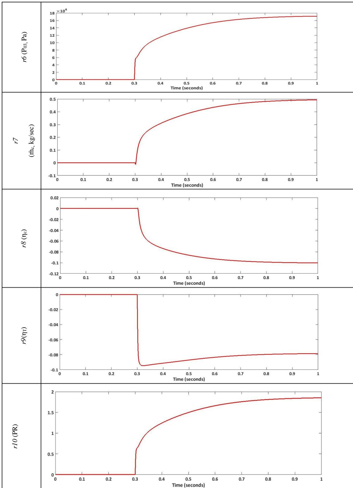
Figure 5.8(b): Residual plots ( $r6$  to  $r10$ ) in case of  $f2b$  (+50% in  $\dot{m}_f$ )
