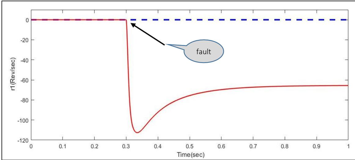
Figure 5.5: Fault detection through residual plot of  $r_1$ (spool speed) in case of  $f_{2a}$  (-78.13% in  $\dot{m}_f$ )
