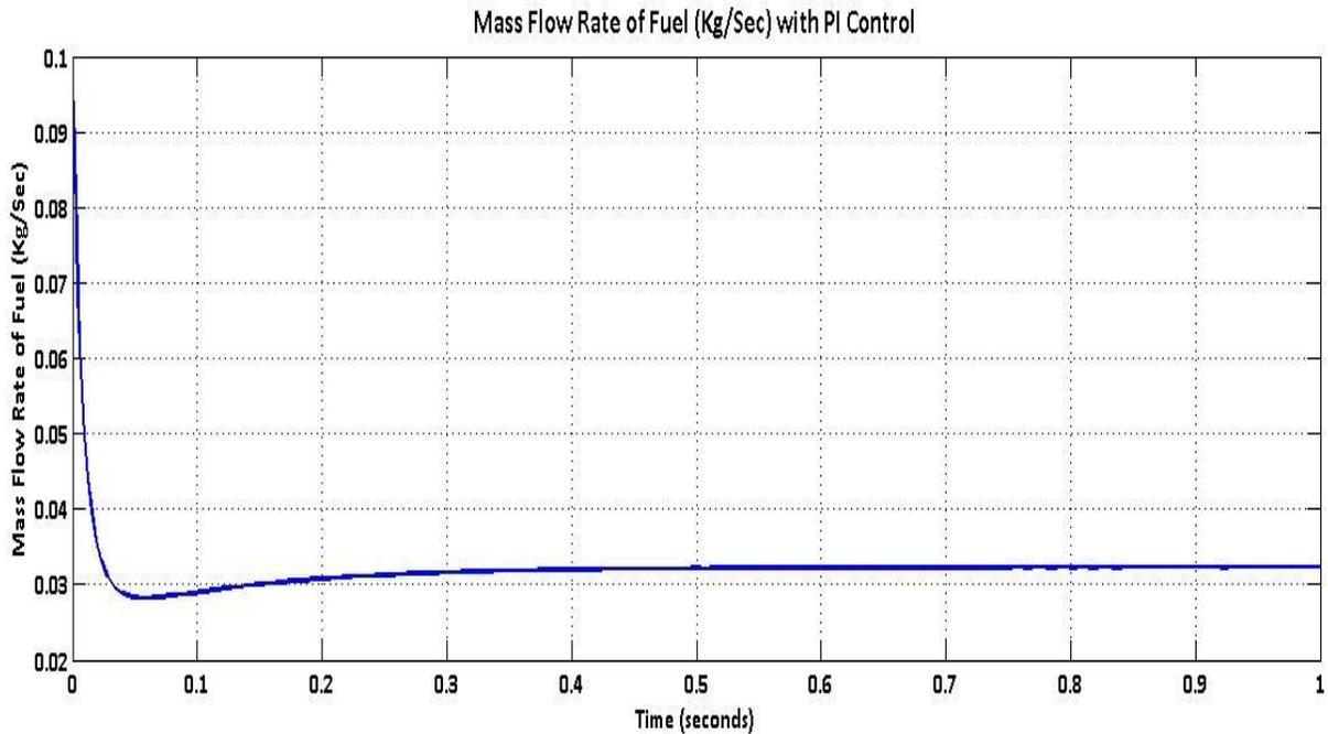
Figure 4.7: Plot showing Fuel Flow rate vs time with PI Controller
