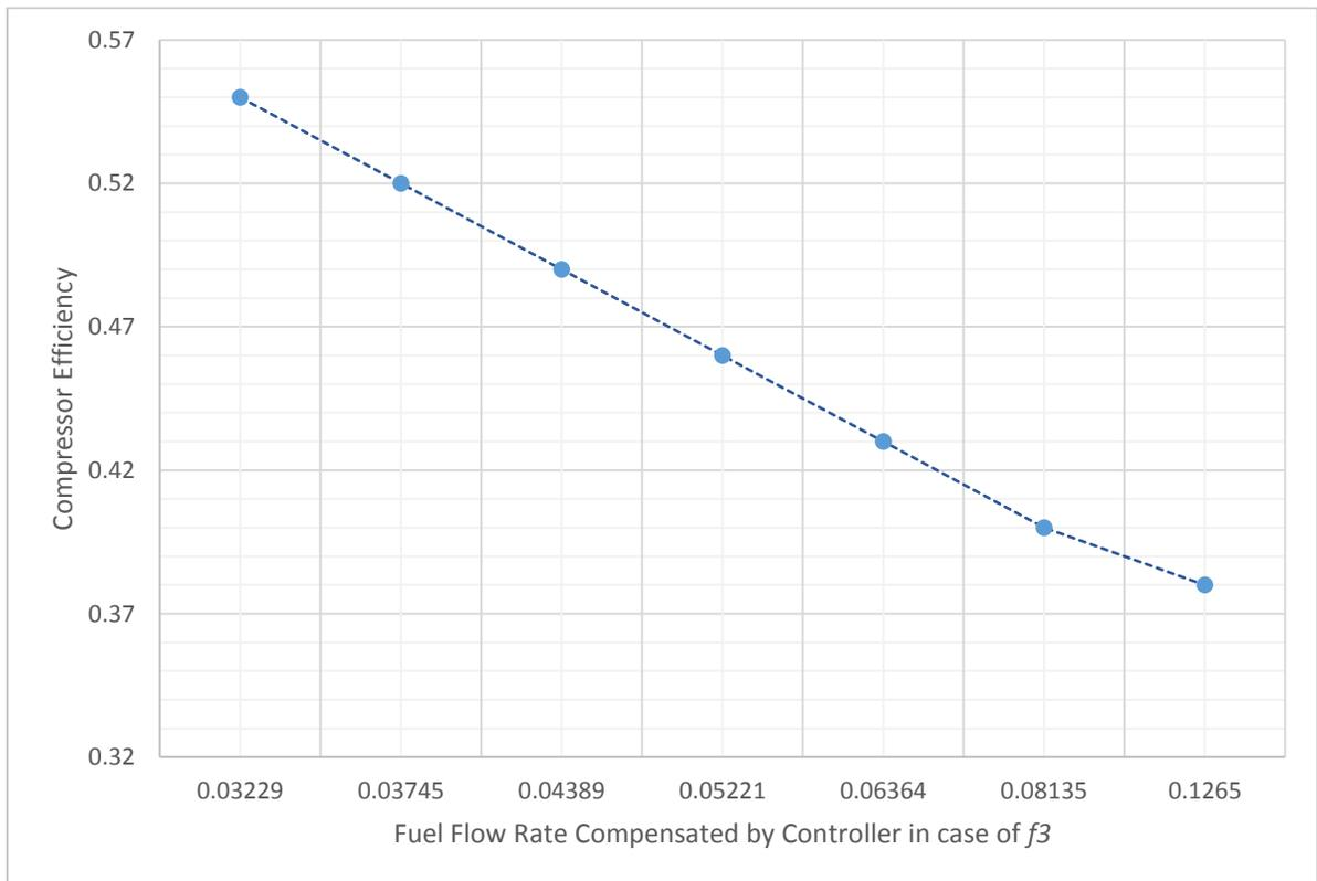
Figure 5.11: Comparison of efficiency loss and fuel flow rate
