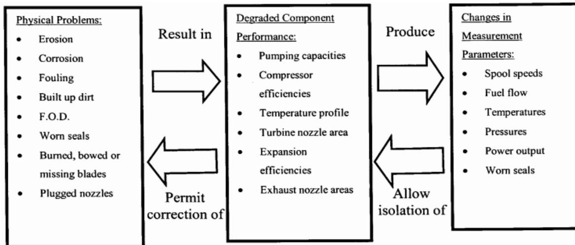
Figure 2.4: Gas Turbine Fault Diagnosis Approach (Urban, 1975)
