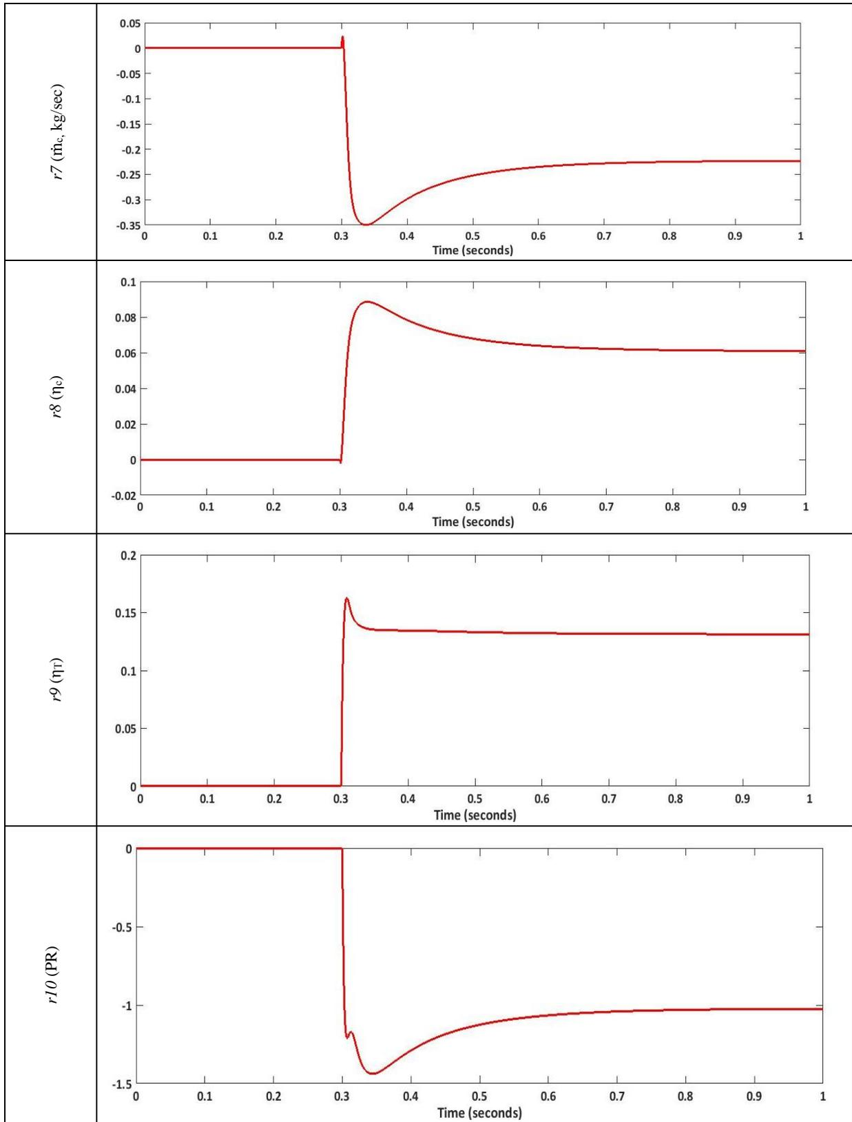
Figure 5.6(b): Residual plots (r7 to r10) in case of f2a (-78.13% in  $\dot{m}_f$ )
