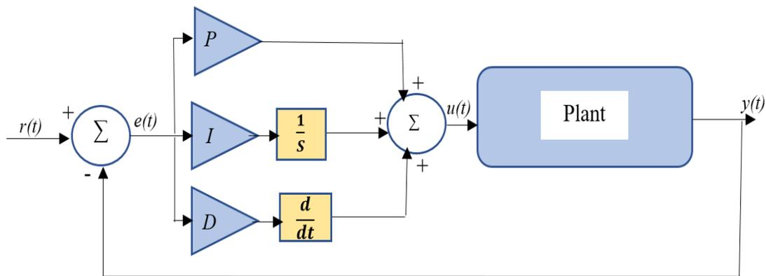
Figure 4.2: PID control structure
