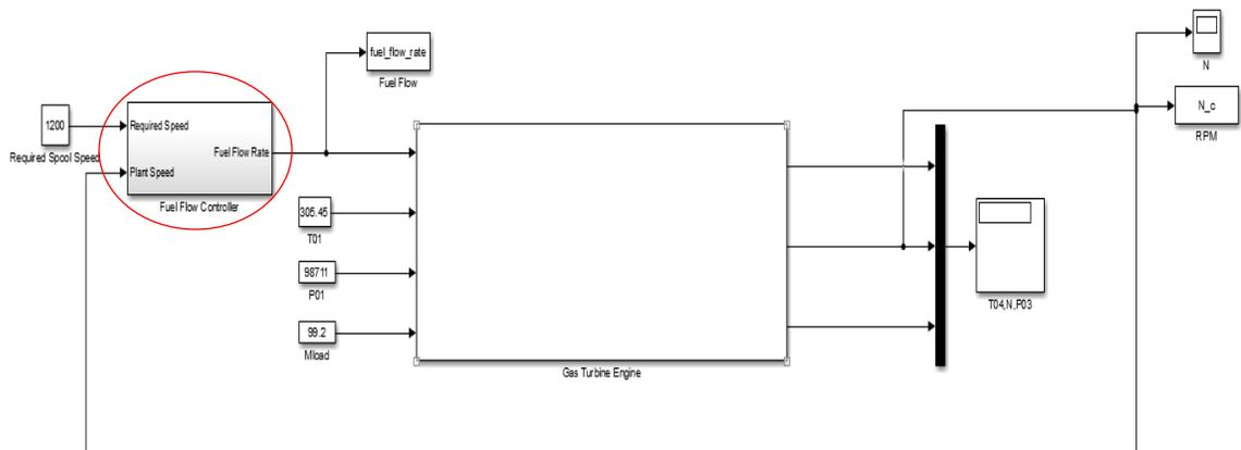
Figure 4.4: Simulink model of PI Control structure for gas turbine fuel management system
