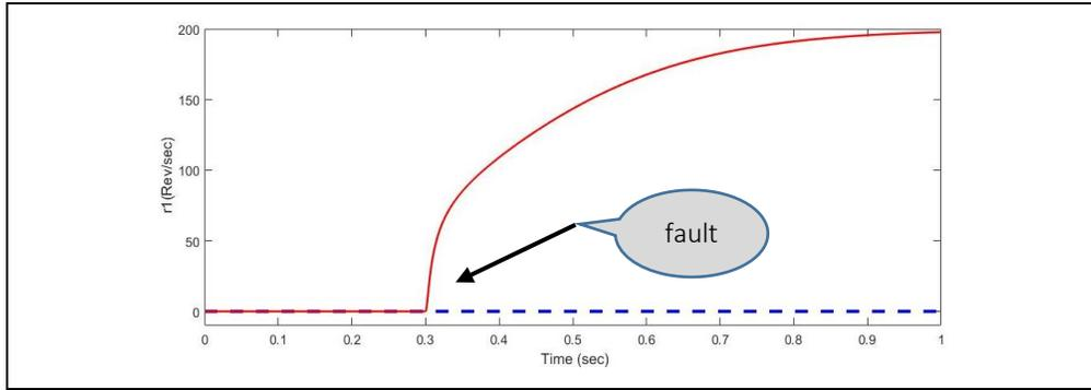
Figure 5.7: Residual plot of  $r1$  (spool speed) in case of  $f2b$  (+50% in  $\dot{m}f$ )
