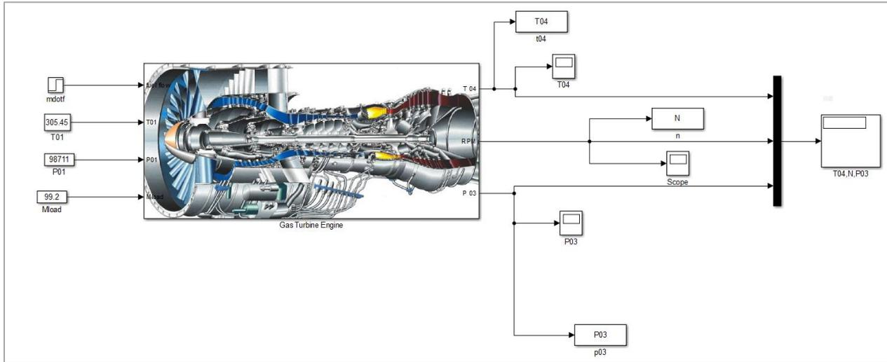
Figure 3.2: Simulink Model of Gas Turbine Engine
