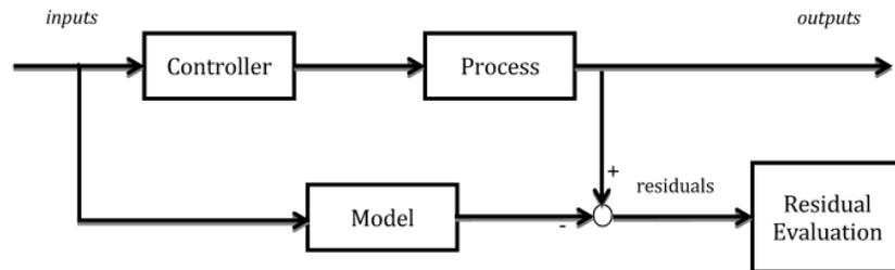
Figure 5.2: The output error residual in model based Fault Diagnosis (Avram, 2012)
