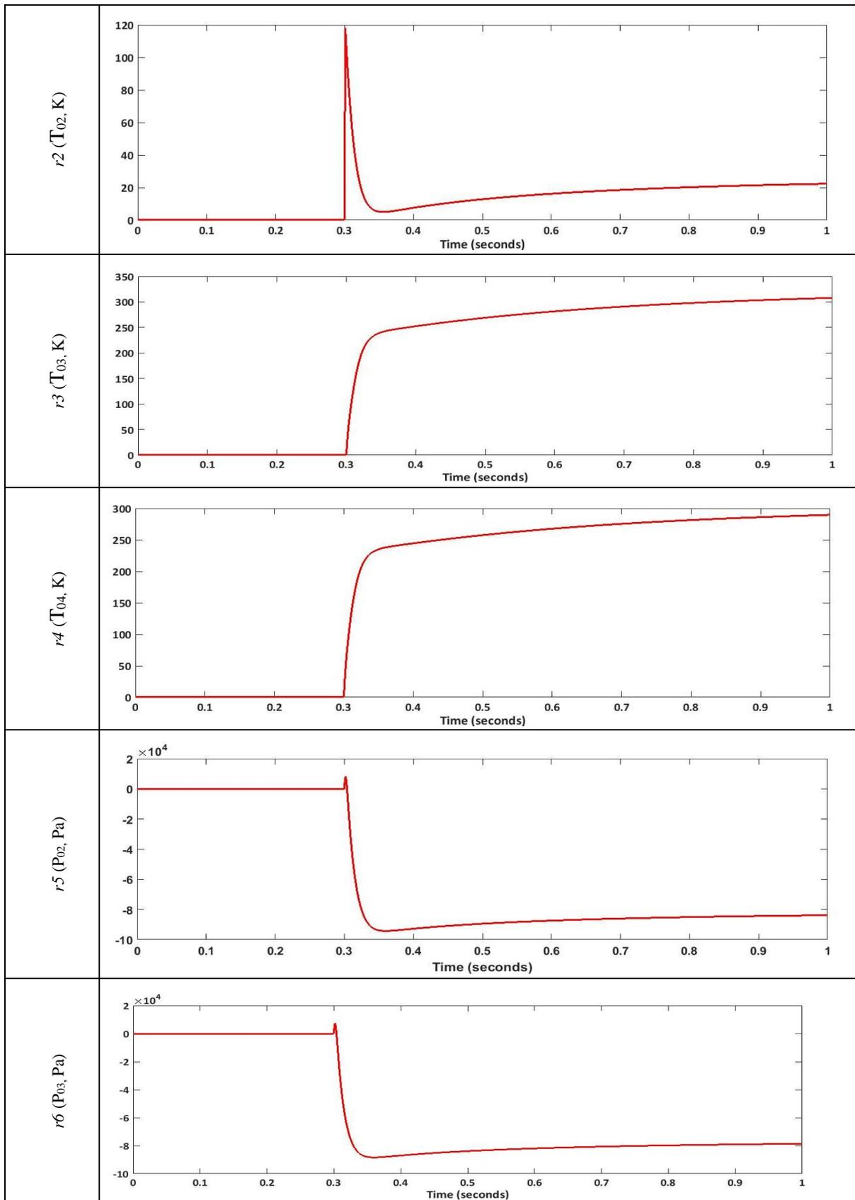
Figure 5.10(a): Results of residual plots ( $r_2$  to  $r_6$ ) in case of  $f_3$  (-26.9% in  $\eta_c$ )
