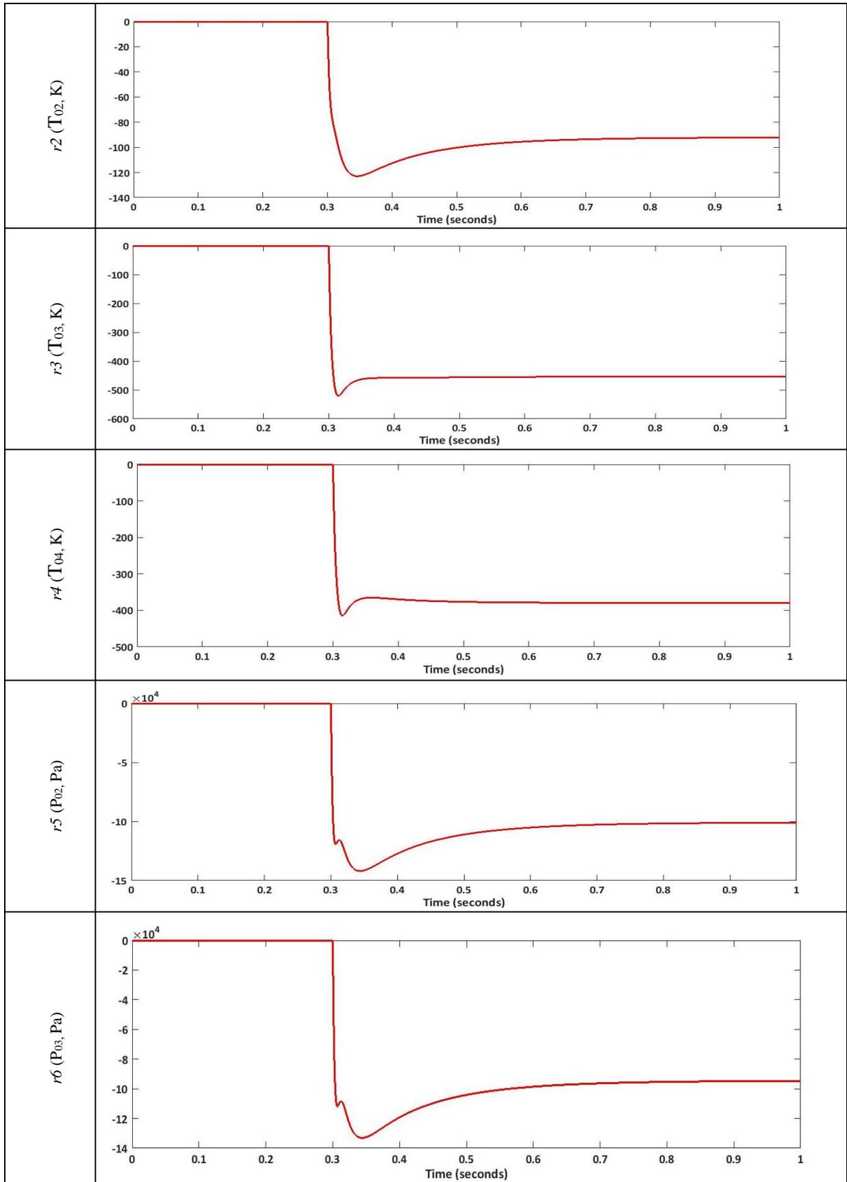
Figure 5.6(a): Residual plots ( $r_2$  to  $r_6$ ) in case of  $f_{2a}$  (-78.13% in  $\dot{m}_f$ )
