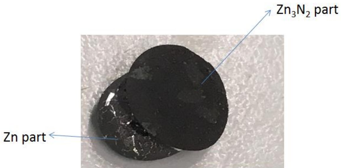
Figure 3. 7 : Image of the final product of the oil bath “quenching” reaction (sample 12).
