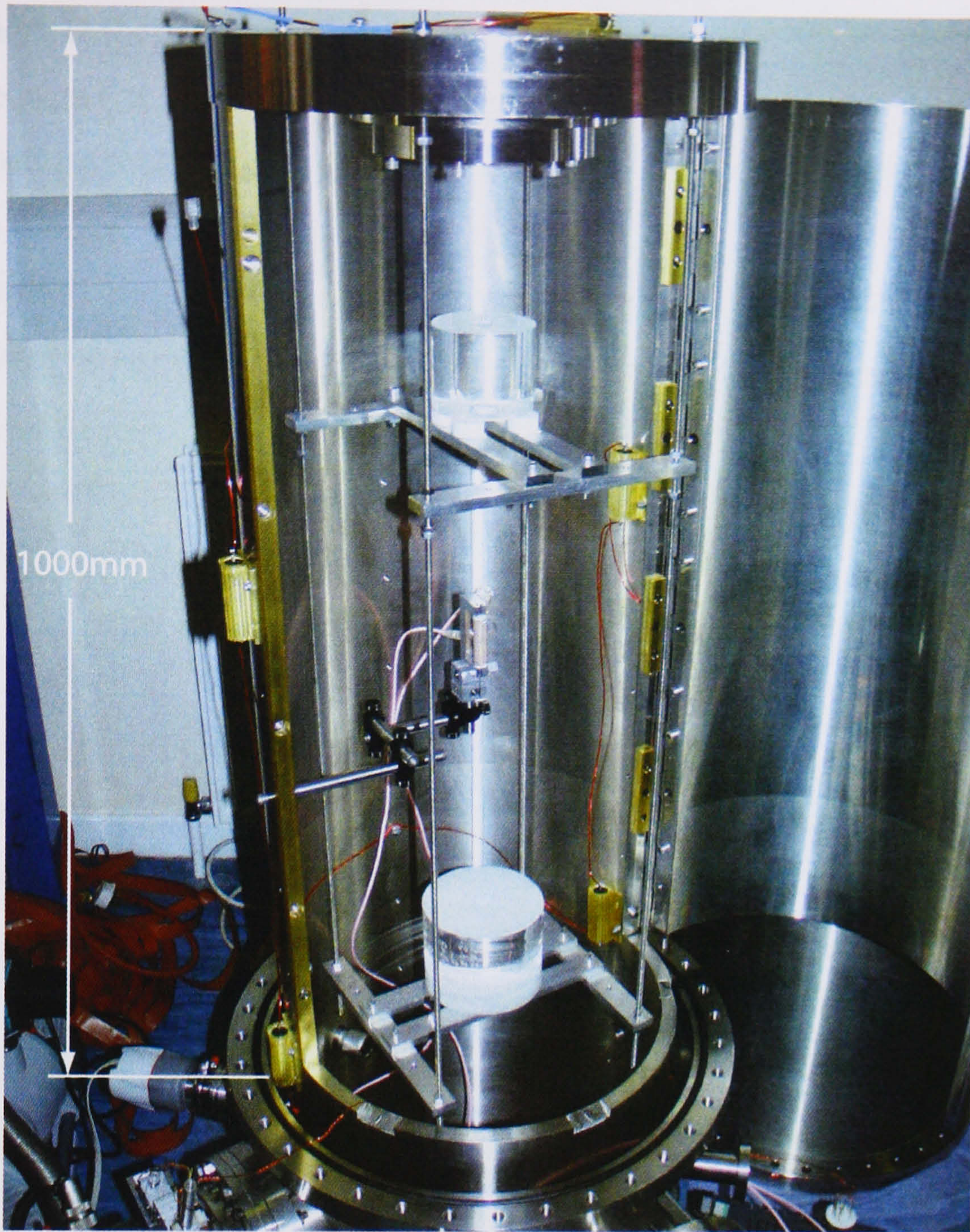
Figure 33: Completed suspension mounted in the support frame on the vacuum tank base. The catcher frame has been lowered and sits close to the underneath of the masses.
