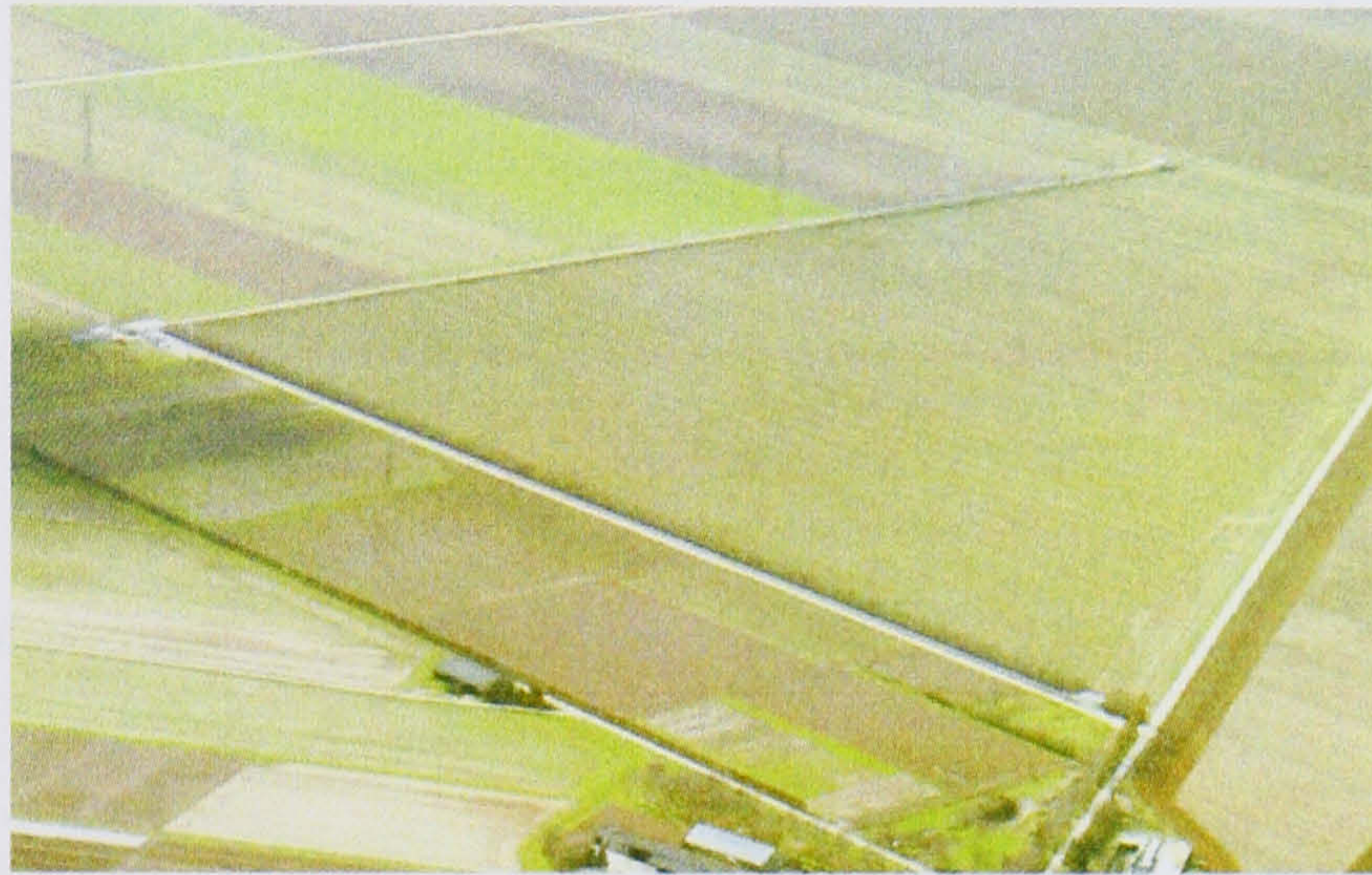
Figure 8: Aerial photo of GEO600 detector near Hannover in Germany showing the two 600m vacuum tube arms and buildings.
