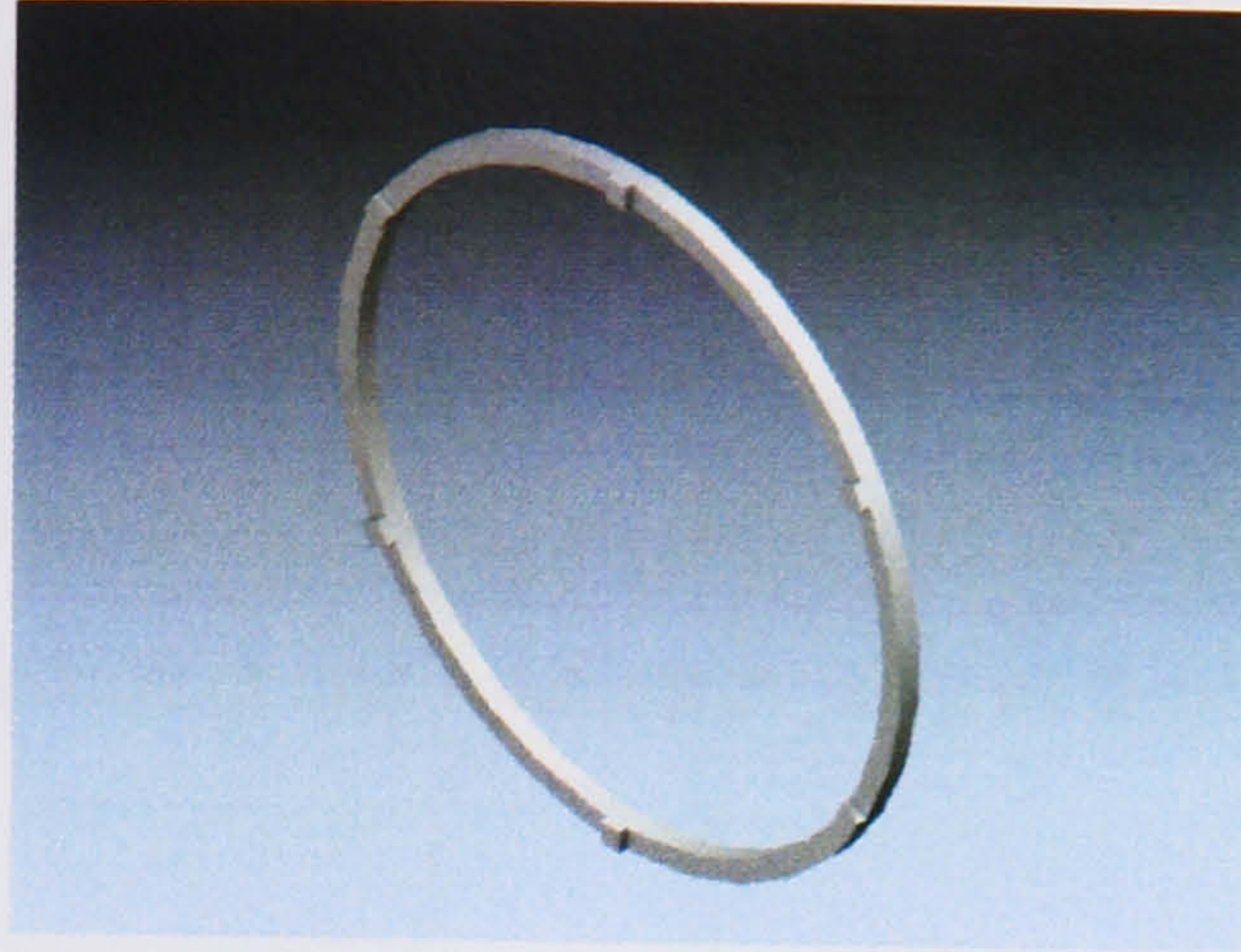
Figure 96: Solidworks rendering of the clamping ring. The six small rectangular feet used to clamp the glass can be seen.
