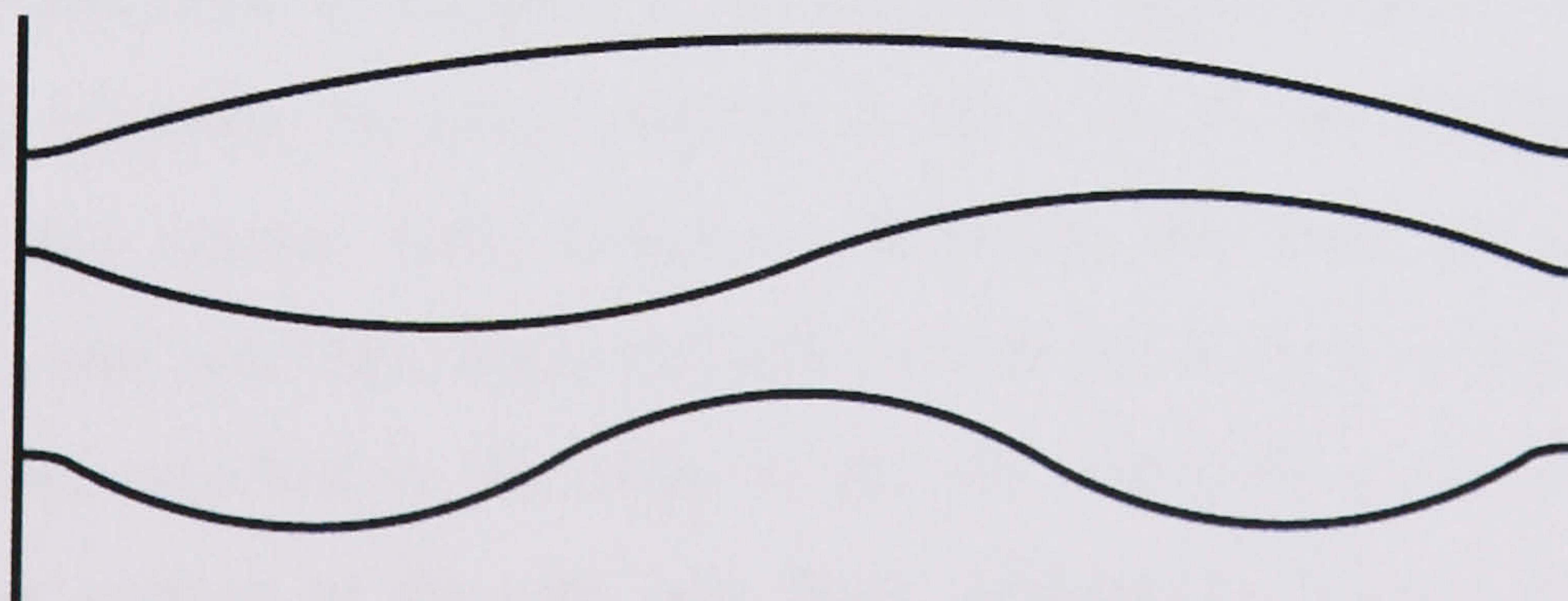
Figure 29: Violin modes of a fibre held at both ends. From top to bottom the first three modes of oscillation are shown.
