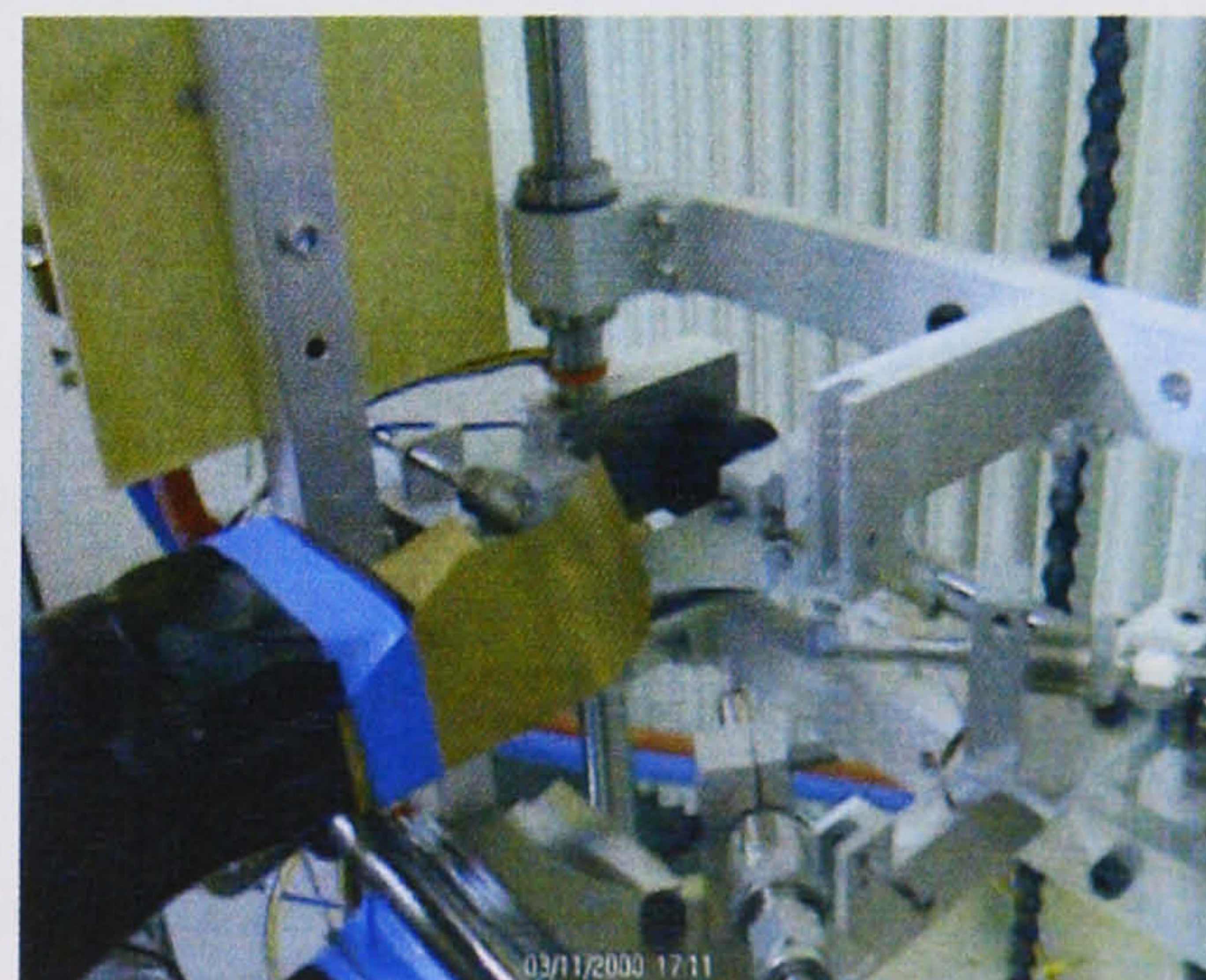
Figure 23: Close-up of burner platform showing five burners arranged in a ring. Fan shown is used to cool upper clamp.
