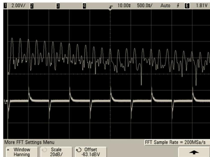
Figure 5.11: Measured time domain transmitted signal and its spectrum in the frequency domain. Hanning window with 200 MSa/s sample rate was used to capture the input signal.
