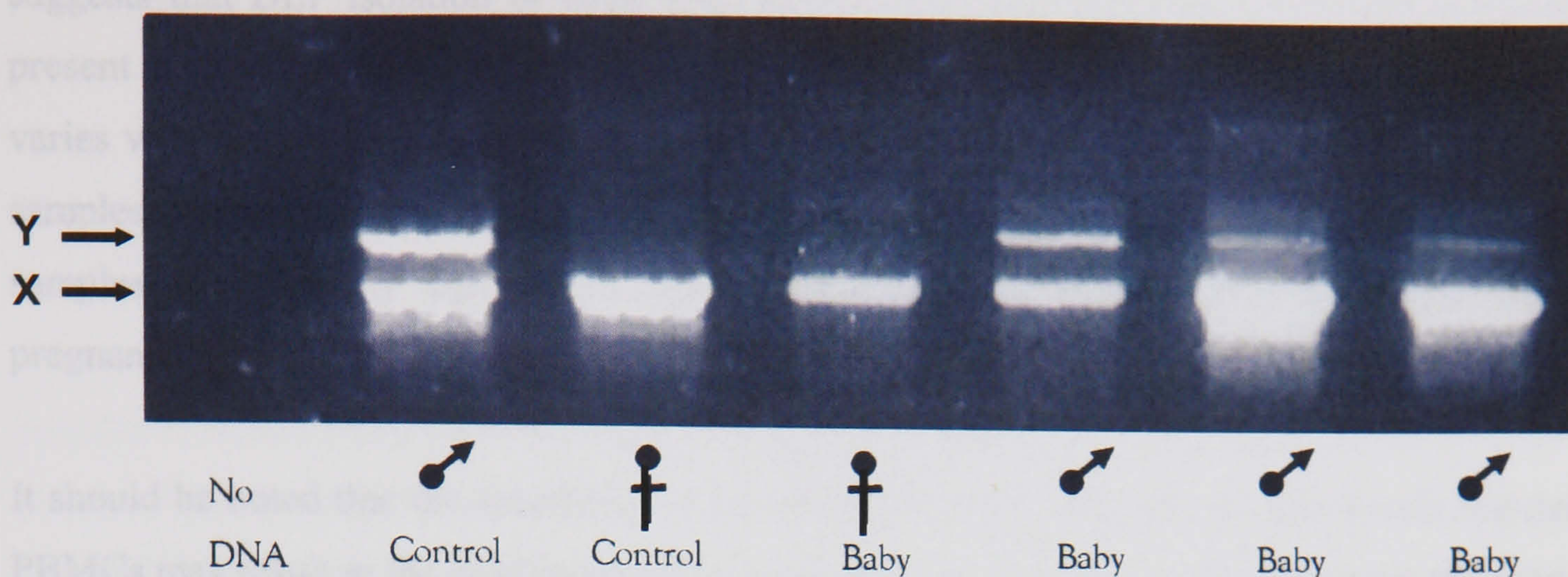
Figure 8-2. PCR results from maternal blood samples passed through an earlier DEP separation system.
