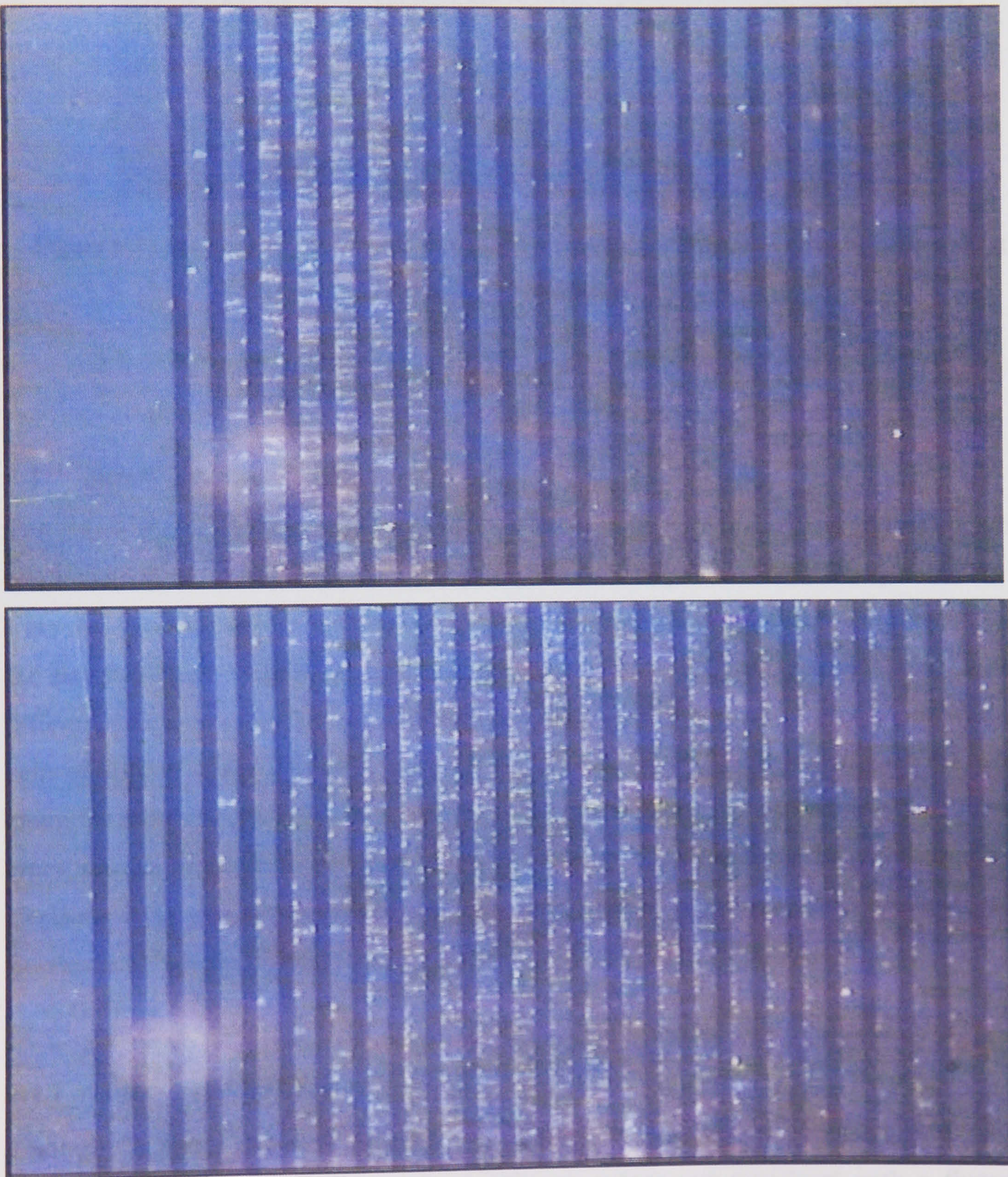
Figure 6-10. Banding of THP-1 cells showing the capture of particles at defined positions along the length of the 40 \mu m electrode array, at flow rates of (a) 0.5mlhr -1 and (b) 1.0mlhr -1 .
