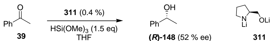
Scheme 3.8. Organocatalytic Enantioselective Reduction of Acetophenone.
