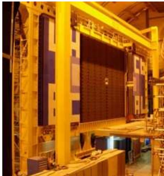
**Figure 2.19:** Schematic diagram of scintillator-absorber layout for the HCAL (left), and photograph of the completed HCAL detector (right). Both figures reproduced from [70].
