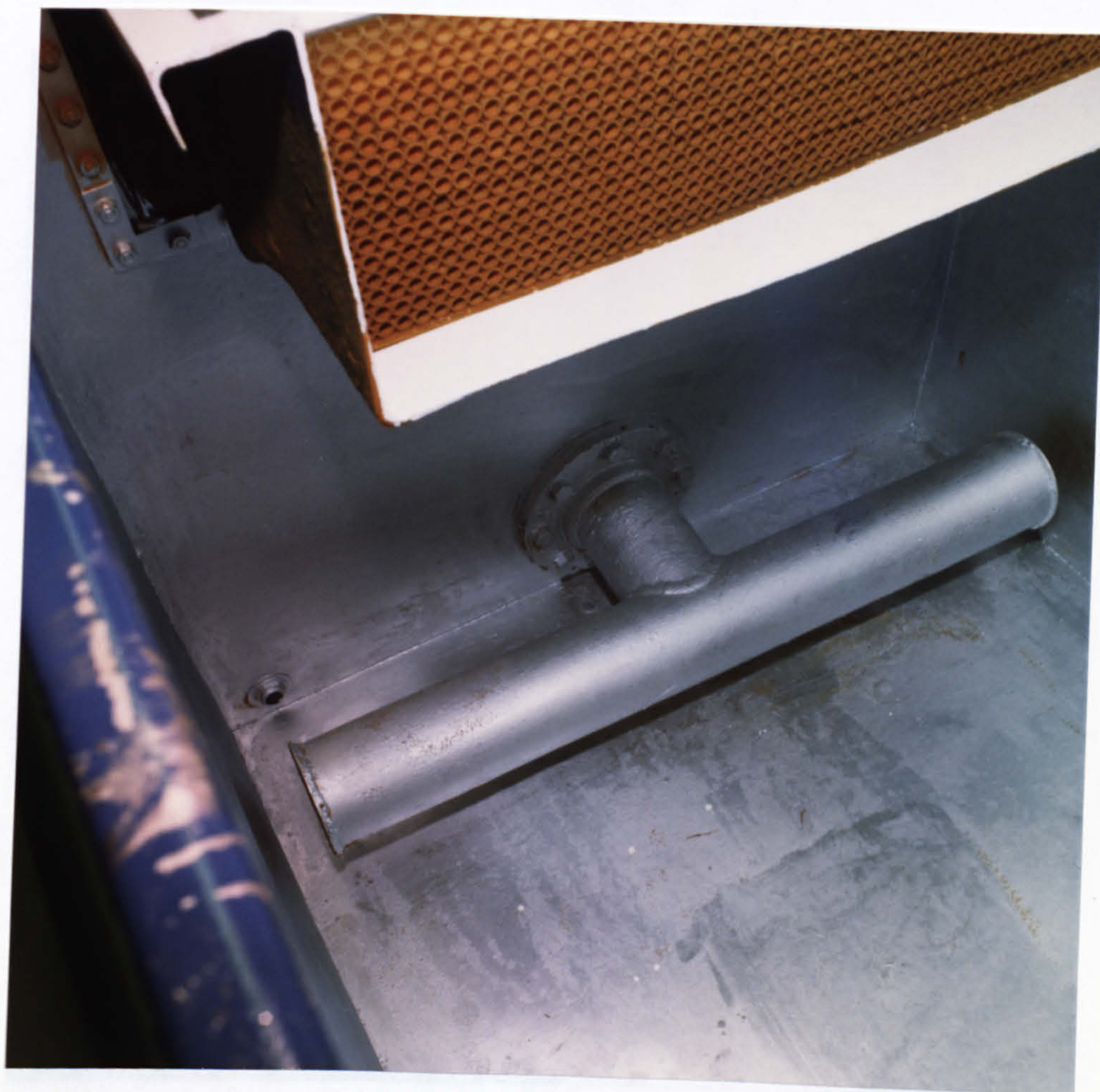
FIG 3.12 T- PIECE SECTION IN THE INLET TANK (HONEYCOMB FLOW STRAIGHTENER ALSO SHOWN).
