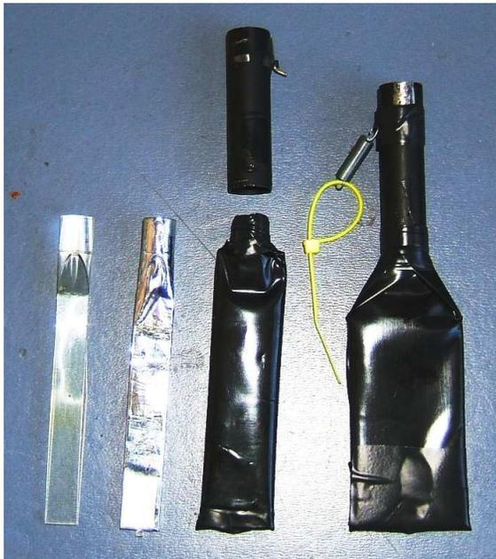
Figure 3.8: Various widths of scintillator through the stages of wrapping: unwrapped (far left), in mylar (second from left), in black tape and below a  $\mu$ -metal tube (second from right) and with  $\mu$ -metal tube attached (far right).
