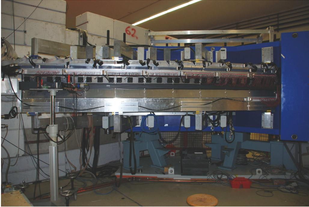
Figure 3.18: The completed Glasgow-Mainz Photon Tagging Spectrometer.
