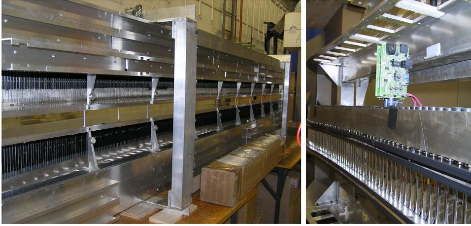
Figure 3.15: Left: The focal plane detector frame. Right: Scintillators mounted therein.
