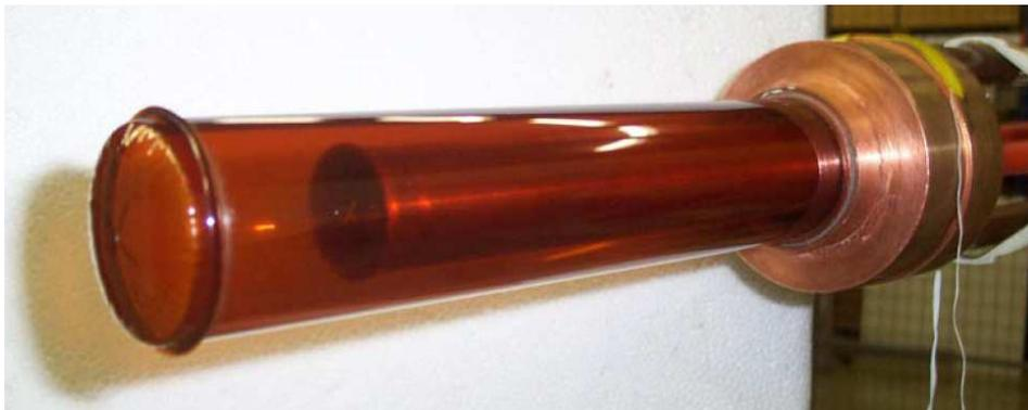
Figure 4.4: Liquid hydrogen target cell [80].
