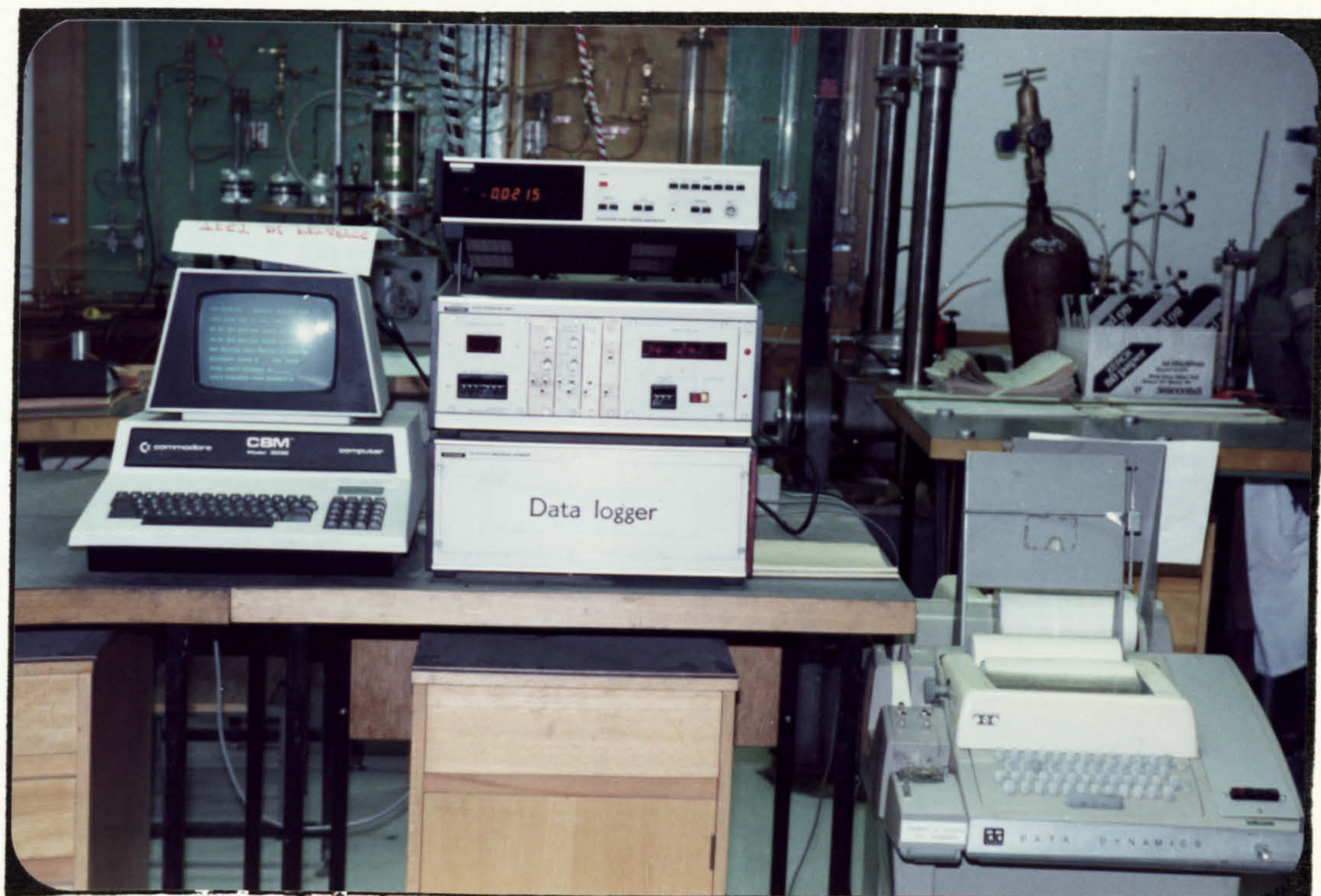
Fig.6.15: The data logging equipment used to collect all the data from the unsaturated soil tests.
