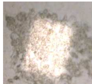
Figure 3-4: Light micrograph of acetone extract of Sitka spruce on Barium fluoride window
