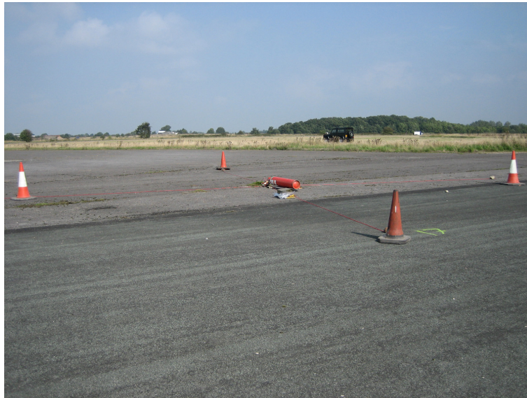
Figure 4.1: The cylinder and perforated pipes laid out to simulate a diffuse micro seepage.
