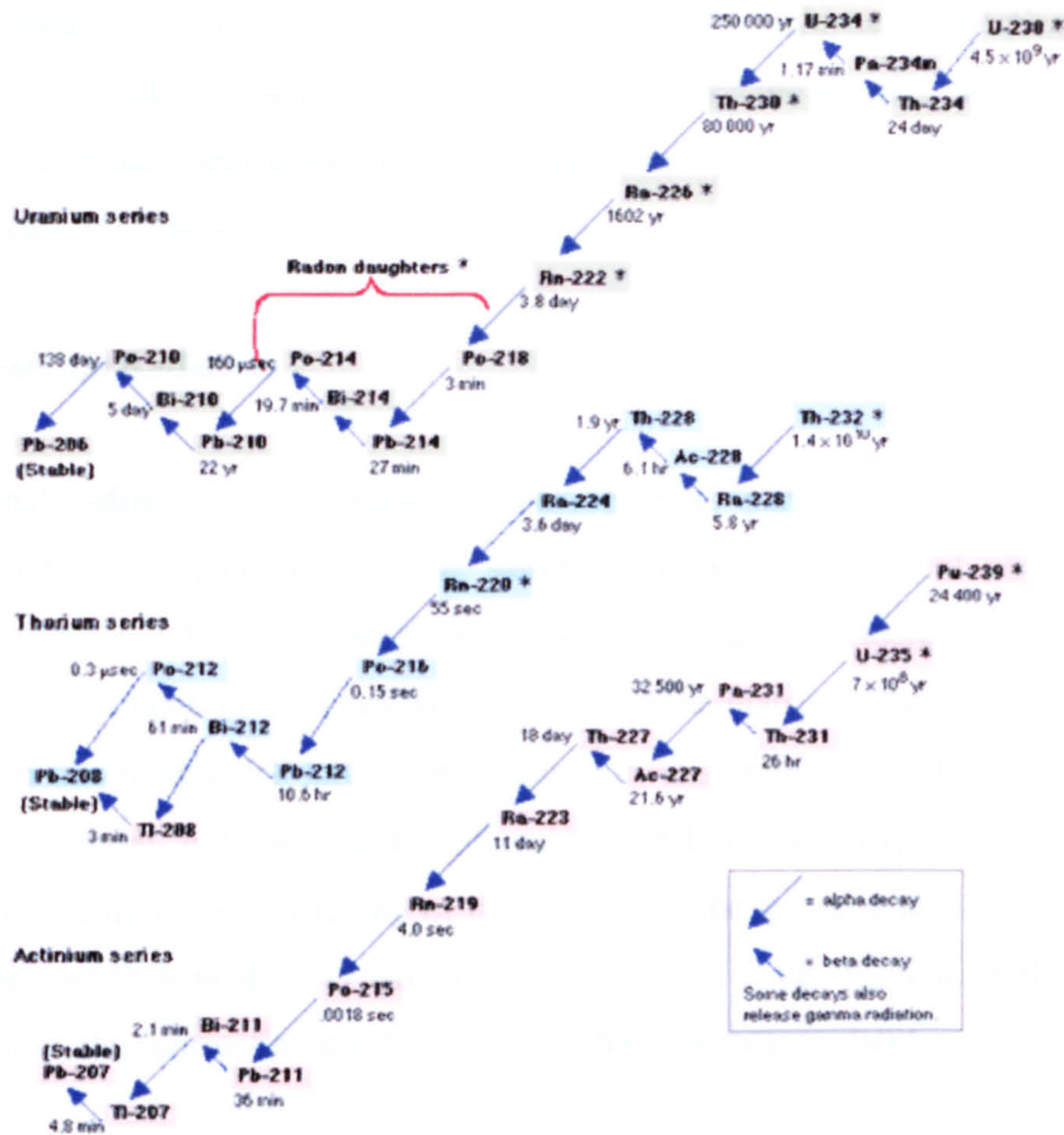
Fig 2. 11 Radioactive Decay series for U and Th (Hore- Lacy, 2003)
