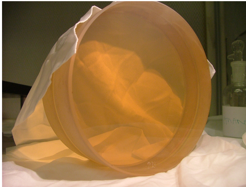
Figure B.13: Photograph of two bonded 12.3 cm diameter Zerodur discs.
