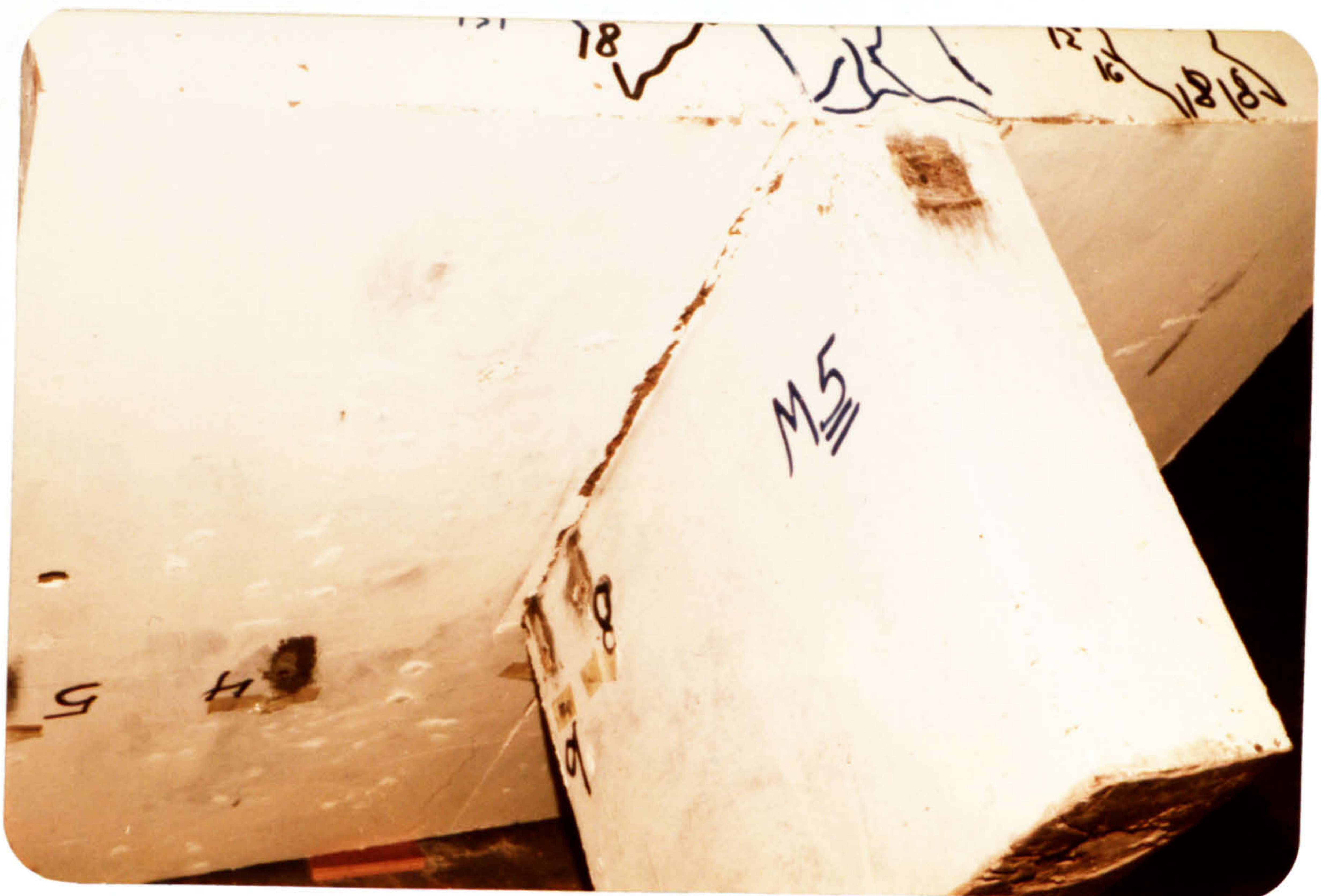
Figure (6.83) : Photograph showing failure of the connection at the bottom of the slab of model MT5 .
