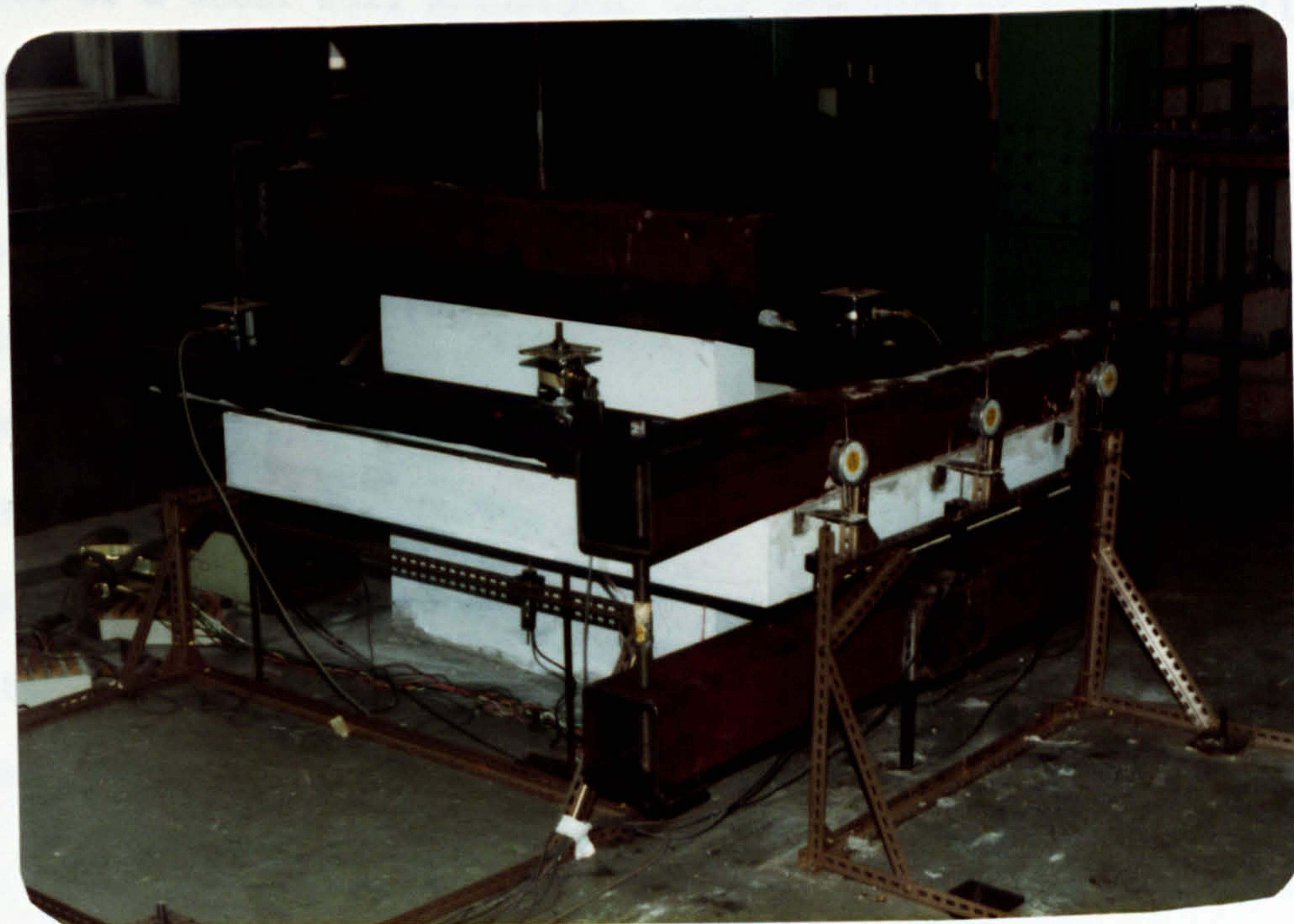
Figure (5.14) : Loading arrangement of a typical model.
