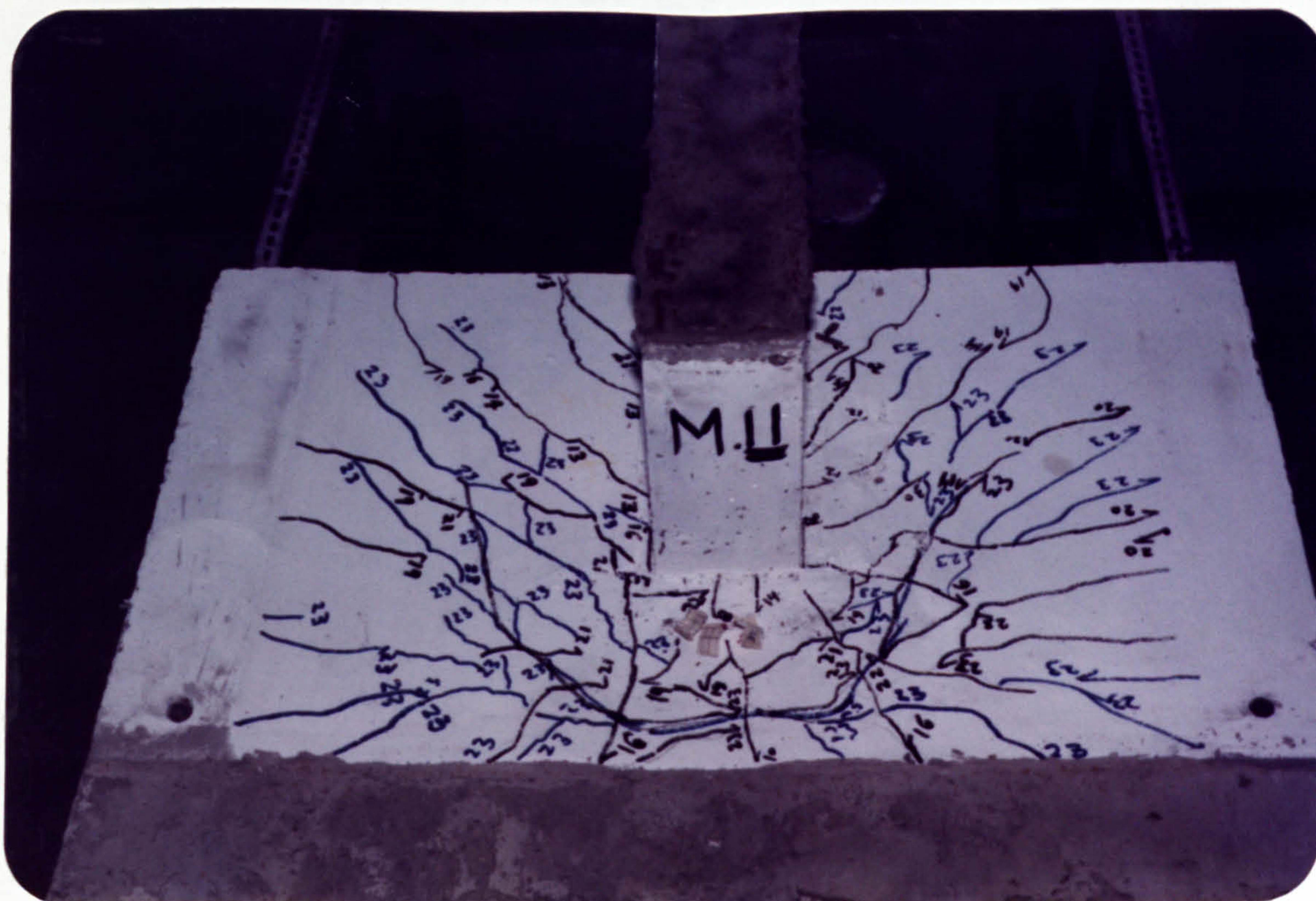
Figure (6.148) : Crack pattern after failure, of the slab of model MT11 .
