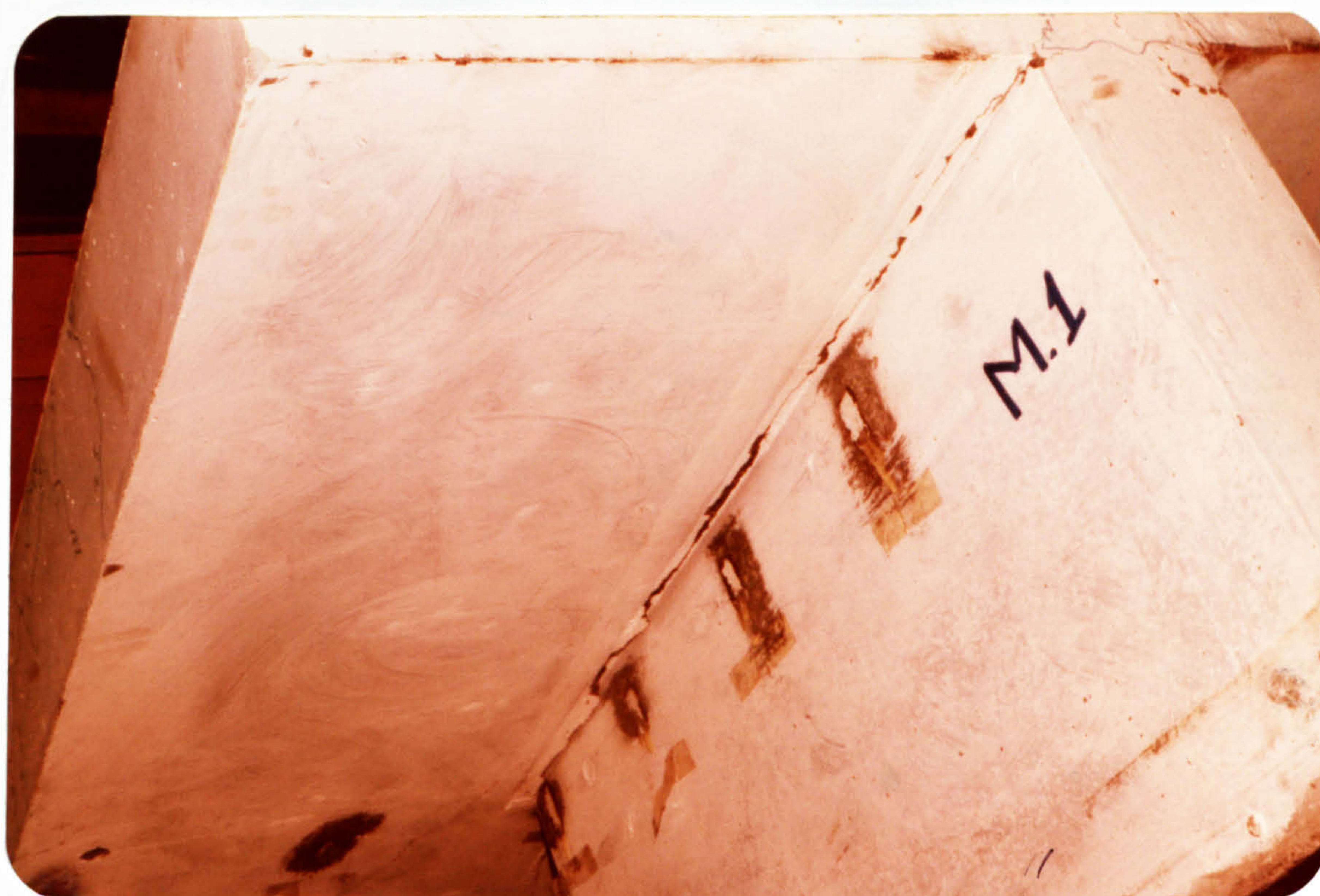
Figure (6.48) : showing the separation of slab from the wall at its bottom in model MT1 .
