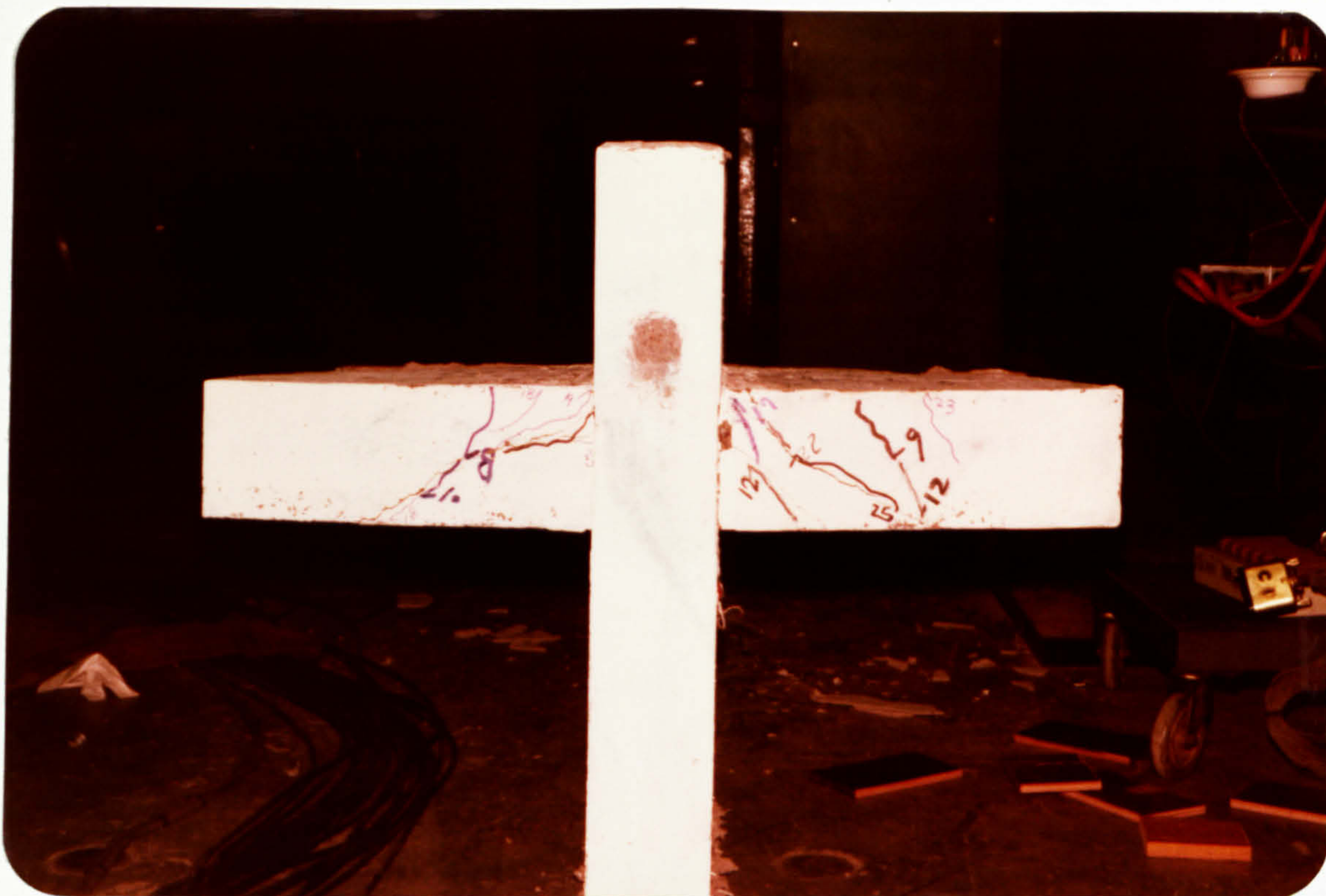
Figure (6.63) : Crack pattern of slab after failure at the back of MT3 .
