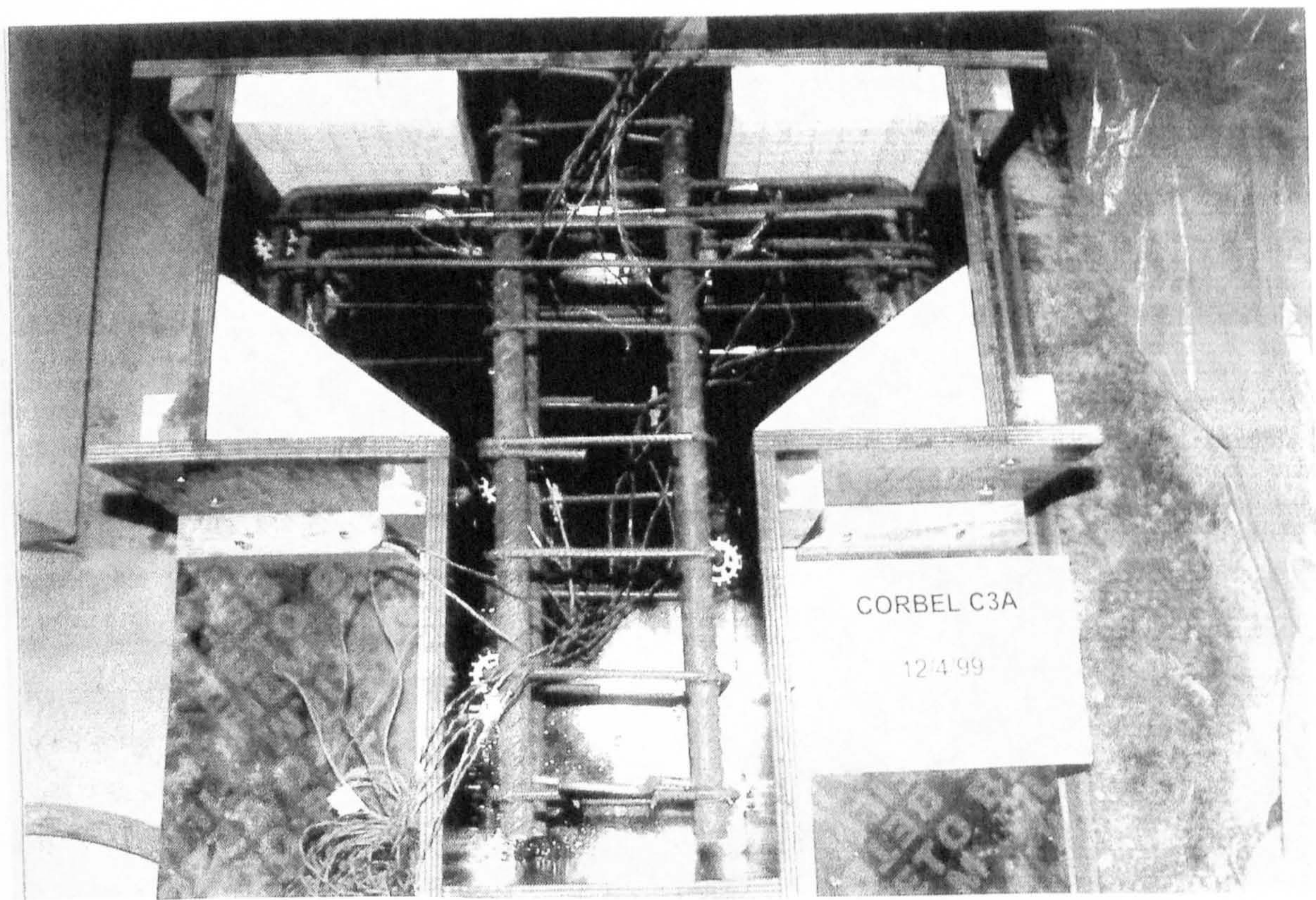
fig.8.4(b) Corbel C3A Reinforcement & Formwork
