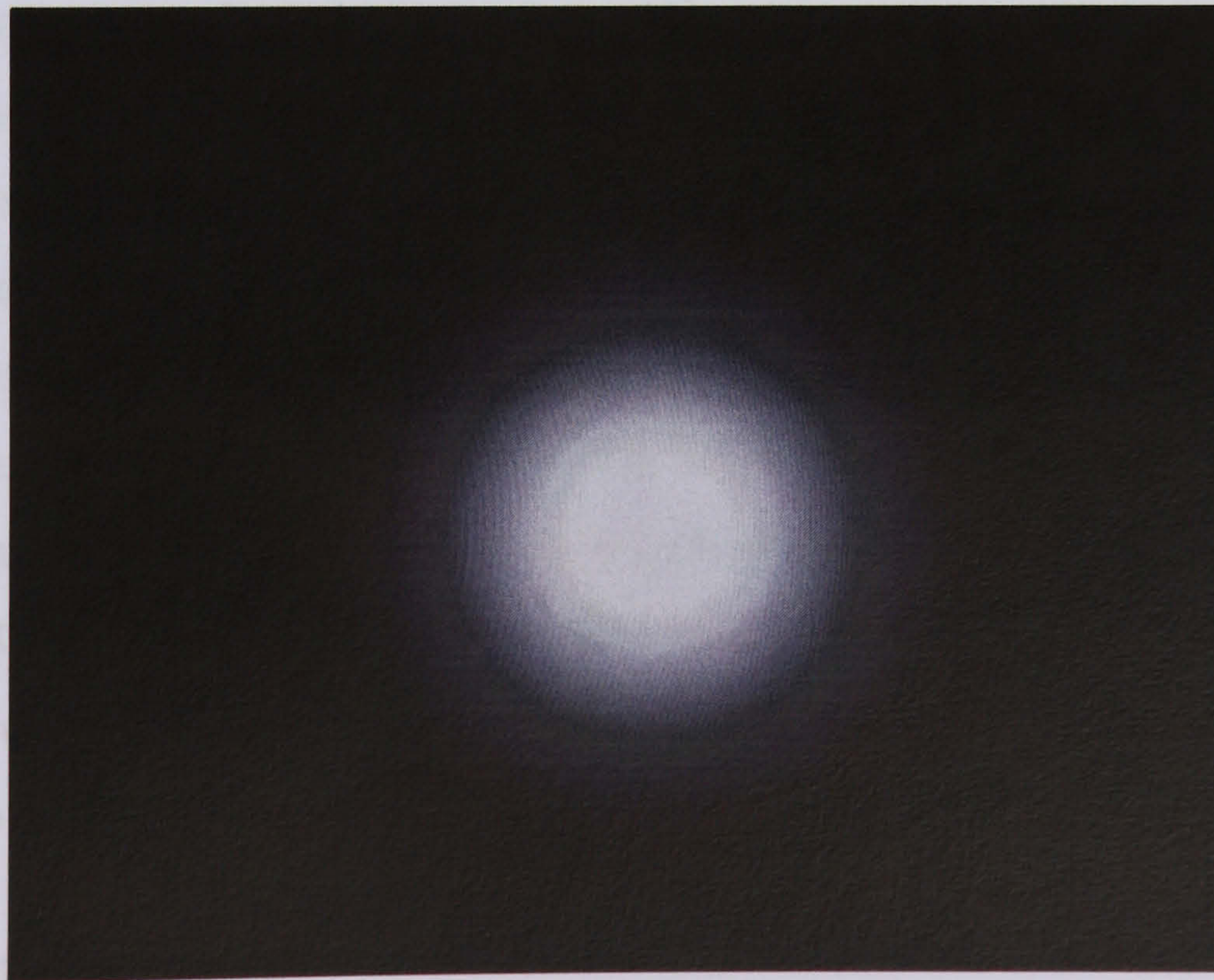
Figure 4.68: A beam spot image at a distance of 12 \text{ mm} from the end of a bare single-mode fibre.
