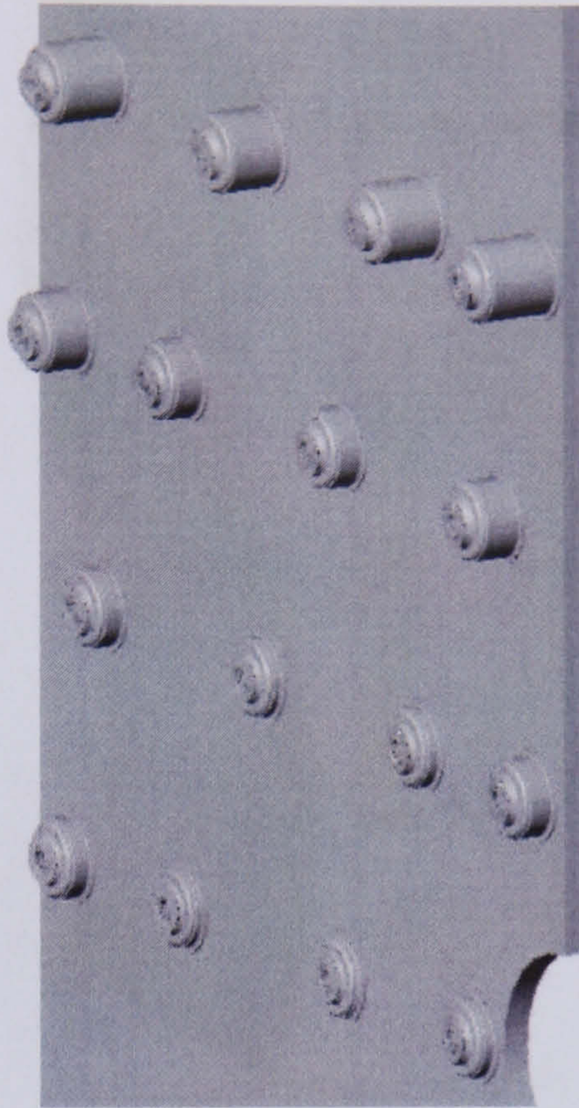
Figure 4.7: Mirror supports on sandwich panel [42].
