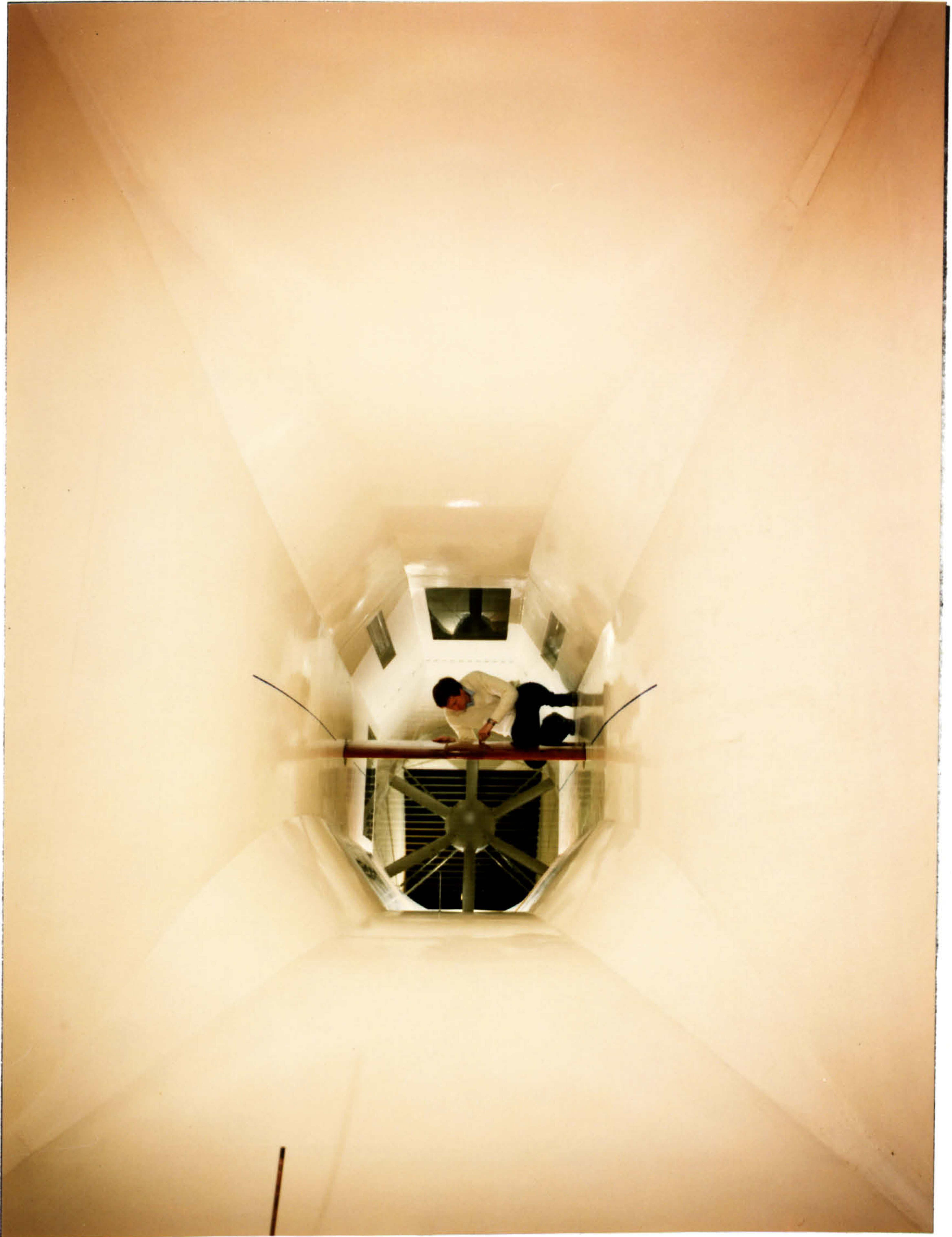
Figure 3.5 View of the aerofoil model in the wind tunnel.
