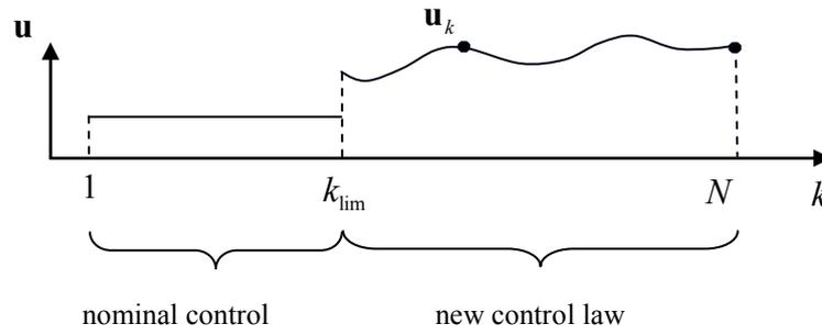
Figure 5.2: Control law schedule according to Jacobson's algorithm.
