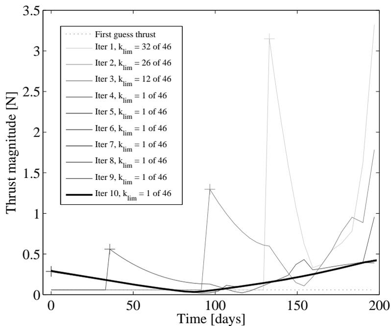
**Figure 5.4: Control law during the convergence process. Direct transfer Earth to Mars, with a time of flight of 200 days.**
