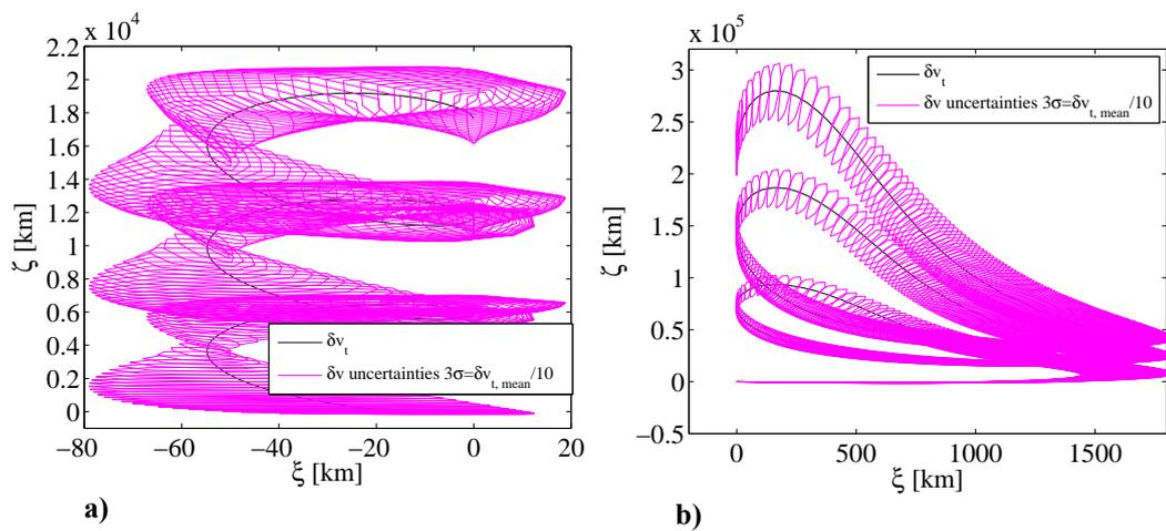
**Figure 2.22: Projection on the  $b$ -plane of the deviation.  $\delta v_{t, \text{mean}} = 0.07$  m/s applied along the tangent direction with  $3\sigma = \delta v_{t, \text{mean}}/10$  for a) asteroid 2000SG344 and b) asteroid 1979XB.**
