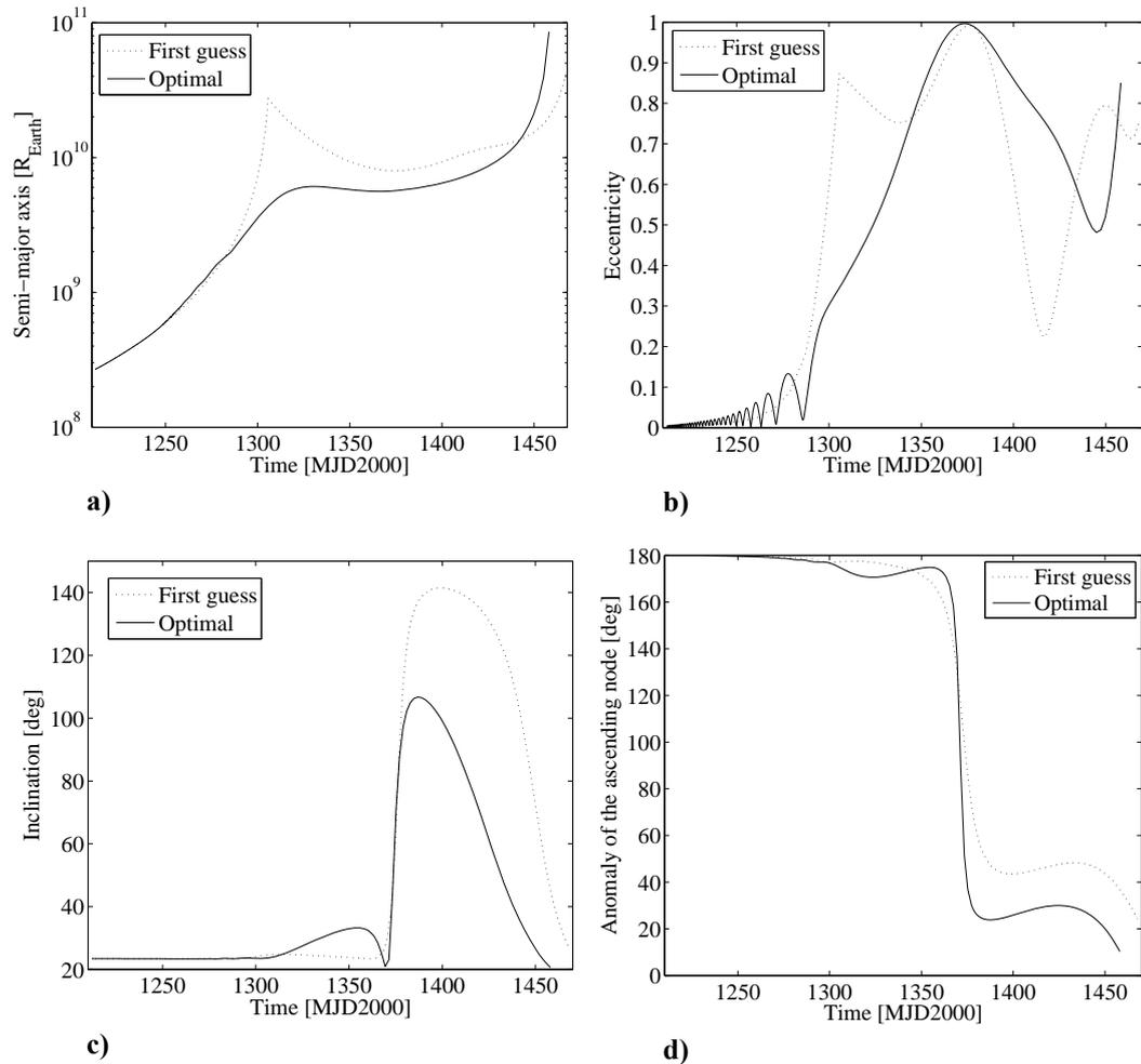
**Figure 5.35: Evolution of the Keplerian elements during the escape phase. The dashed line represents the first guess solution; the continuous line is the optimal profile. a) Semi-major axis, b) eccentricity, c) inclination, and d) anomaly of the ascending node.**
