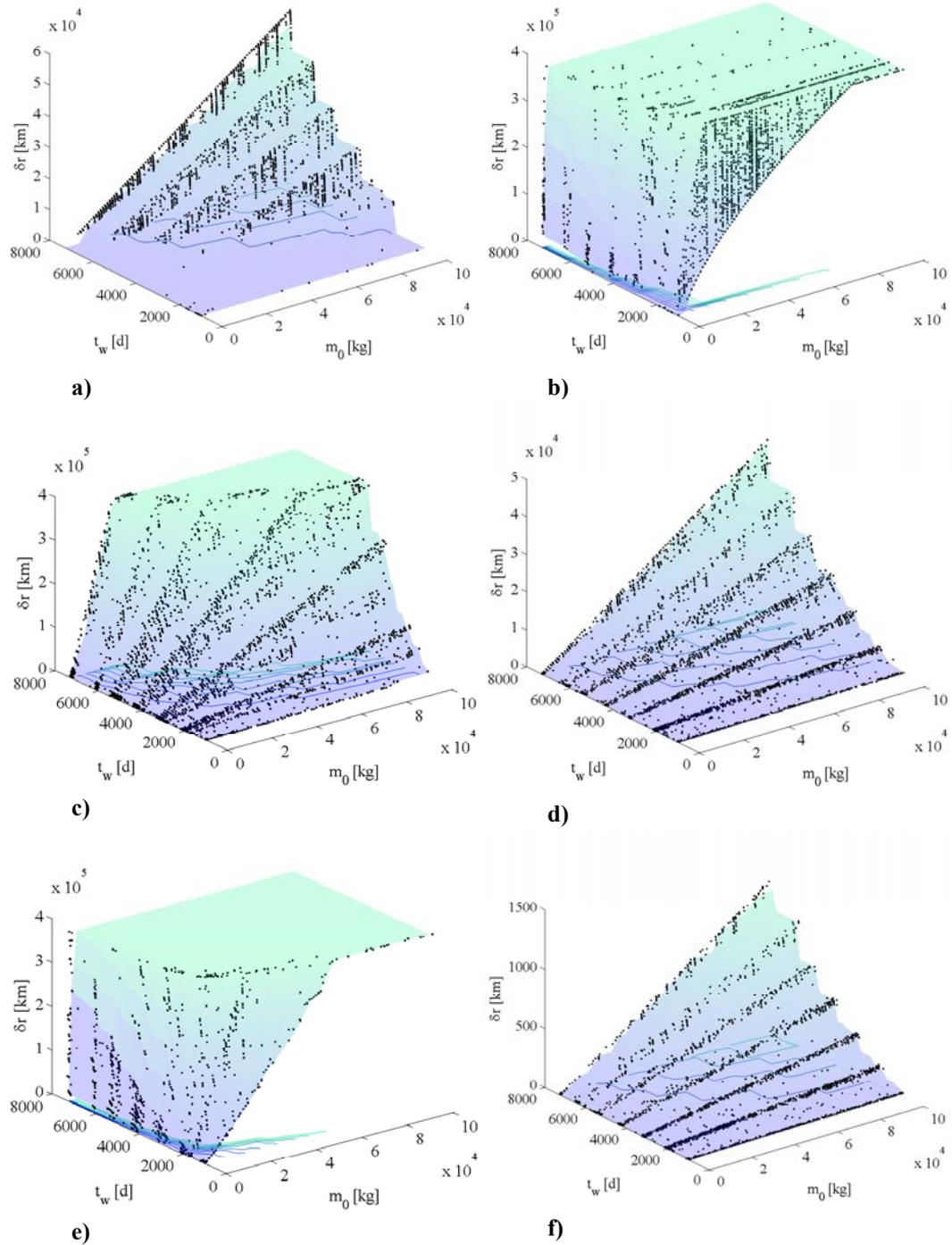
**Figure 4.3: Pareto front for the deviation of asteroid Itokawa through different strategies: a) kinetic impactor, b) nuclear interceptor, c) mass driver, d) attached spacecraft propulsion, e) solar collector, and e) gravity tractor.**
