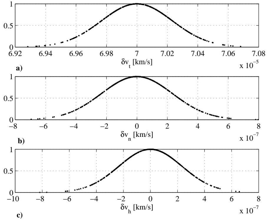
**Figure 2.19: Distribution of the components of  $\delta v$ , represented through the Gaussian membership function, with  $3\sigma = \delta v_{t, \text{mean}}/100$ . a) Tangential component, b) normal component, and c) component along the  $h$  direction.**
