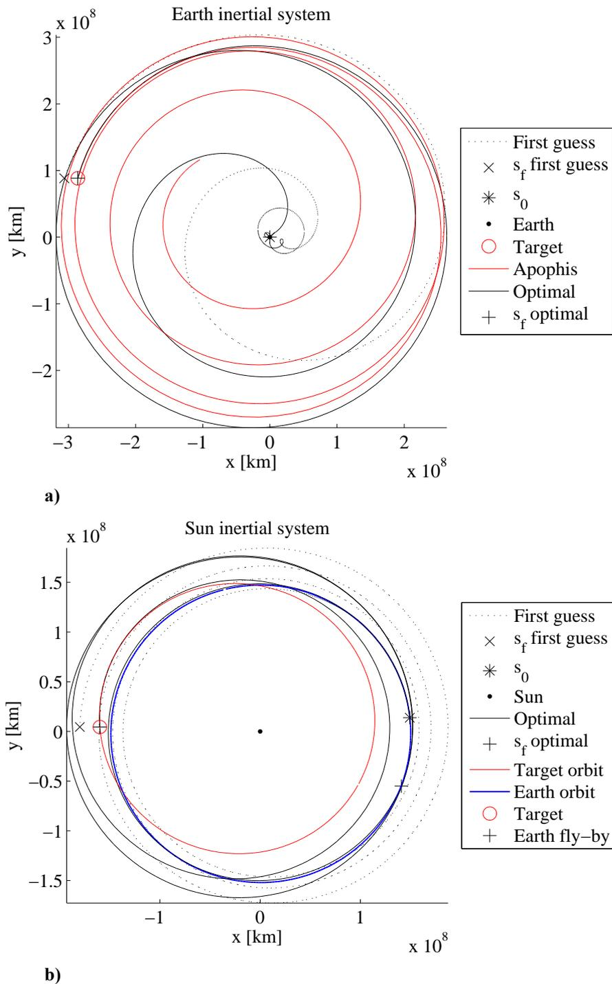
**b)** Figure 5.25: Trajectory to Apophis rendezvous. The dashed line represents the first guess transfer solution; the continuous line is the optimal trajectory. a) Transfer in the Earth inertial reference frame. The circle represents the target position, the cross is the final state of the optimal trajectory. b) Transfer in the Sun inertial reference frame. Apophis and Earth orbit are represented respectively in red and blue continuous lines.
