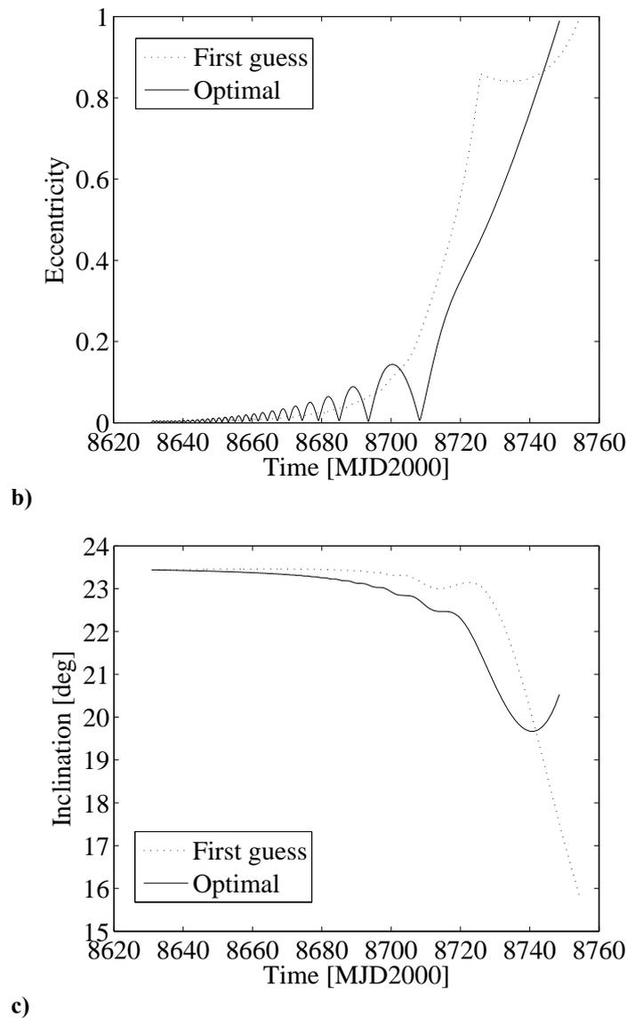
**Figure 5.16: Evolution of the Keplerian elements during the escape phase. The dashed line represents the first guess solution; the continuous line is the optimal profile. a) Semi-major axis expressed in Earth radii, b) eccentricity and c) inclination.**
