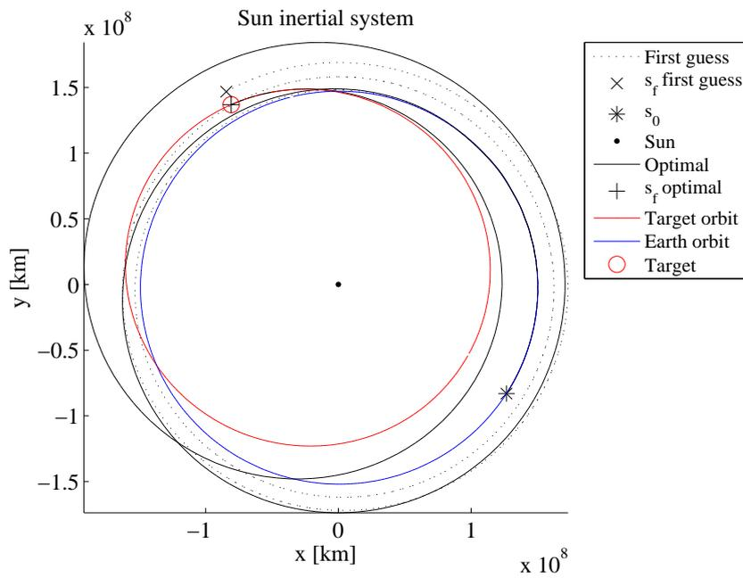
**Figure 5.15: Trajectory to Apophis rendezvous. Transfer in the Sun inertial reference frame. The dashed line represents the first guess transfer solution; the continuous line is the optimal trajectory. Apophis and Earth orbit are represented respectively in red and blue continuous lines.**
