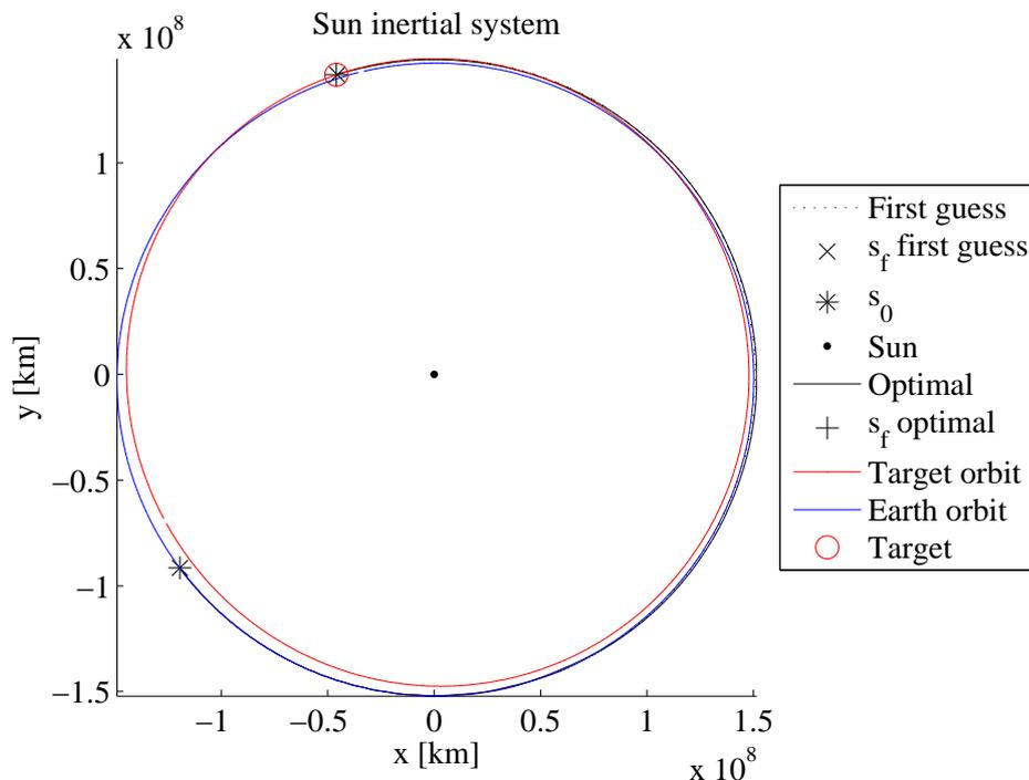
**Figure 5.30: Transfer trajectory to 2002 AA29 fly-by in the Sun inertial reference frame. The dashed line represents the first guess transfer solution; the continuous line is the optimal trajectory. 2002 AA29 and Earth orbit are represented respectively in red and blue continuous lines.**
