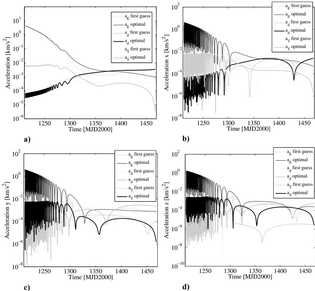
**Figure 5.38: Acceleration components.** The dashed line represents the first guess solution, the continuous line is the optimal solution. The black line indicates the acceleration due to the Earth's gravity field, the black bold line indicates the disturbing acceleration due to the Sun and the bold grey line indicates the thrust acceleration. a) Acceleration magnitude, b) x component of the acceleration, c) y component of the acceleration, and d) z component of the acceleration.
