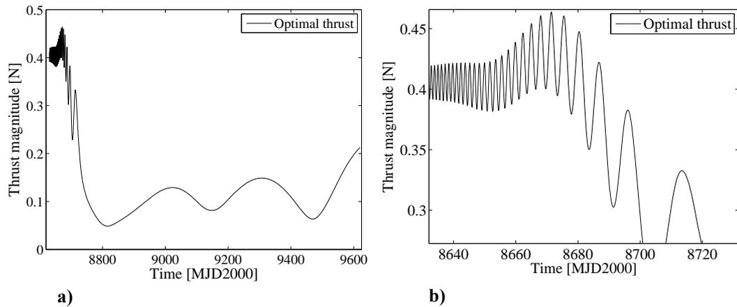
a) **Figure 5.18: Thrust magnitude for the mission with  $m_0 = 1350$  kg. The dashed line represents the first guess solution provided to the DDP algorithm, the continuous line is the optimal thrust profile. a) Entire trajectory and b) close-up on the escape phase.**
