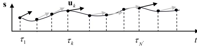
**Figure 5.6: Trajectory discretisation in the Static/Dynamic Control approach.**
