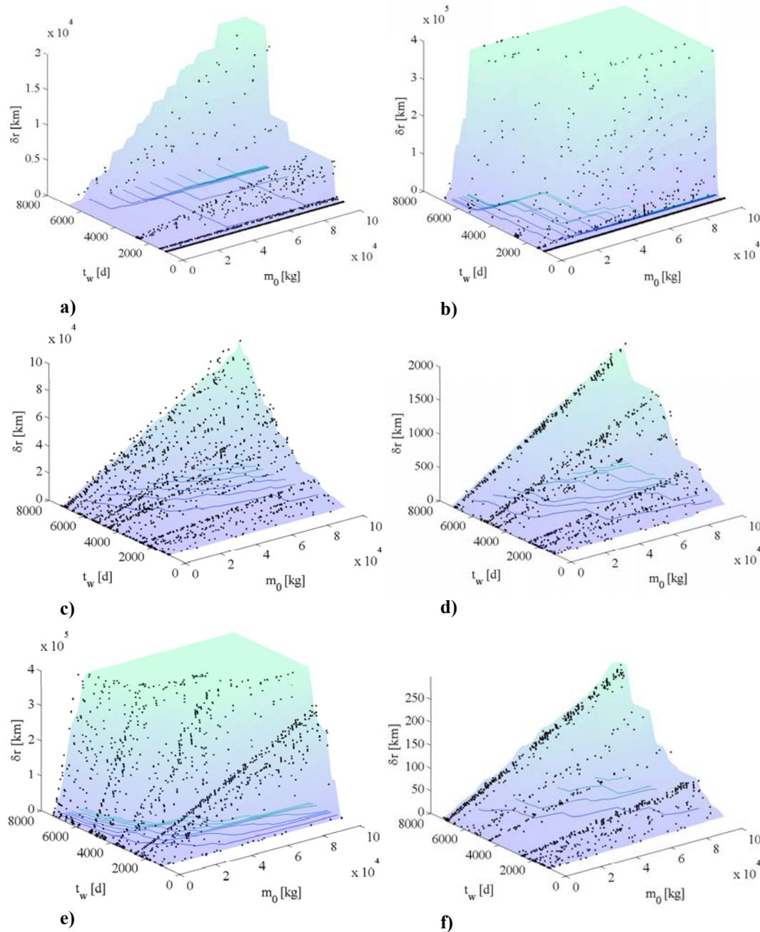
**Figure 4.5: Pareto front for the deviation of asteroid 1979XB through different strategies: a) kinetic impactor, b) nuclear interceptor, c) mass driver, d) attached spacecraft propulsion, e) solar collector, and e) gravity tractor.**
