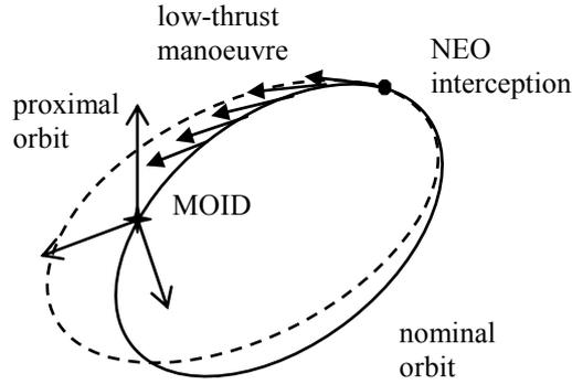
Figure 3.1: Low-thrust NEO deviation.
