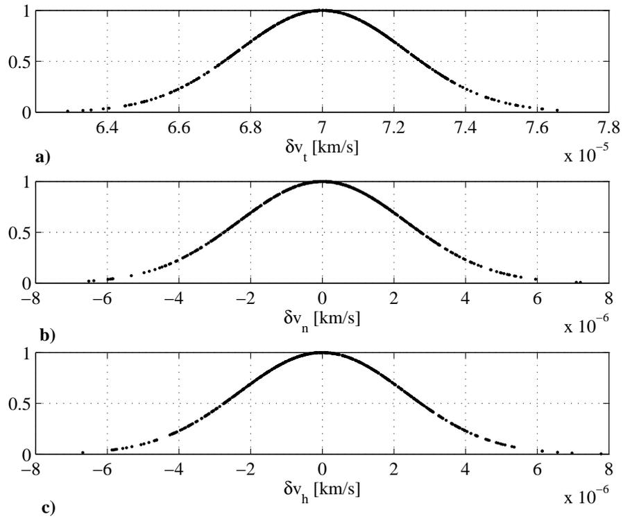
**Figure 2.21: Distribution of the components of  $\delta v$ , represented through the Gaussian membership function, with  $3\sigma = \delta v_{t, \text{mean}}/10$ . a) Tangential component, b) normal component, and c) component along the  $h$  direction.**
