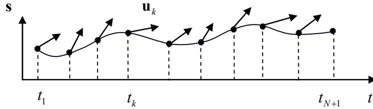
**Figure 5.5: Trajectory discretisation within the optimisation problem.**
