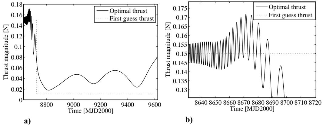
**Figure 5.11: Thrust magnitude.** The dashed line represents the first guess solution provided to the DDP algorithm, the continuous line is the optimal thrust profile. a) Entire trajectory and b) close-up on the escape phase.
