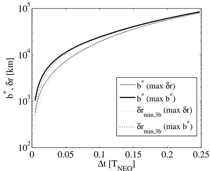
**Figure 2.13: Projection of the deviation (continuous line) on the  $b$ -plane calculated through the two-body problem and minimum deviation computed through the three-body problem (dashed line) for asteroid 1979XB. The bold lines represent the results of the maximum- $b^*$  strategy, the thin lines represent the result for the maximum-deviation strategy.**
