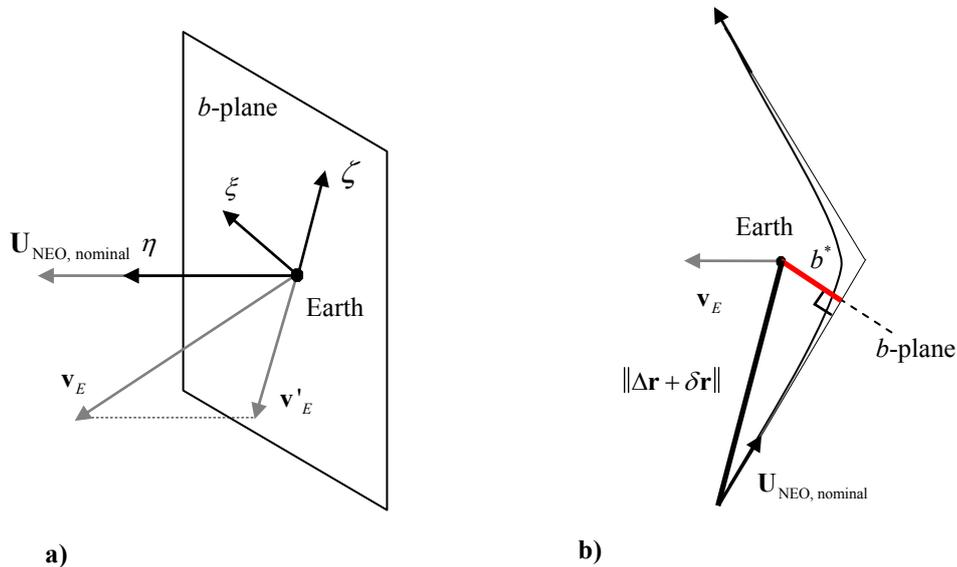
a) **Figure 2.8: Earth-centred local reference system: a)  $b$ -plane representation and b) geometry of hyperbolic passage.**
