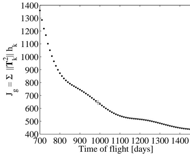
**Figure 5.17: Time of flight sensitivity.** The integral term of the cost function (normalised to the weight parameter  $w$ ) is represented on the y axis. Each point represents an optimised transfer (with final constraints satisfied) with a given time of flight. The cross shows the result corresponding to the solution fully presented in this section.
