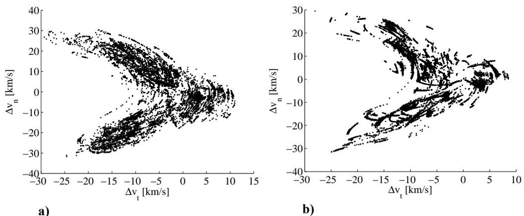
a) Figure 2.29: Optimal impact  $\Delta v$  distribution for direct impacts: a) results of the single-objective optimisation and b) results of the multi-objective optimisation.
