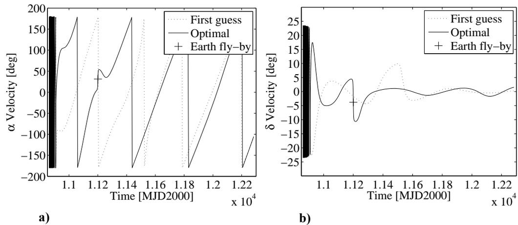
**Figure 5.28: Evolution of the angles of the velocity vector with respect to the Earth inertial reference frame, during the fly-by. The dashed line represents the first guess solution; the continuous line is the optimal profile. The cross symbol is in correspondence of the pericentre passage. a) In-plane angle of the velocity vector and b) out-of-plane angle of the velocity vector.**
