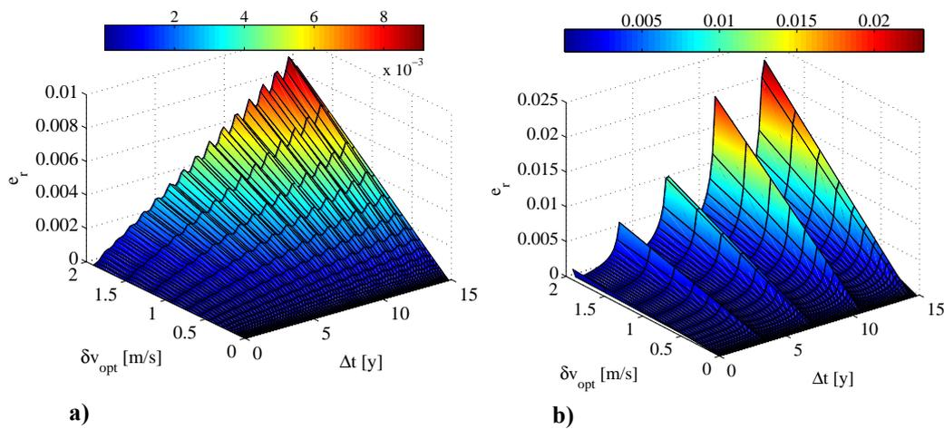
a) **Figure 2.5: Relative error for the deviation of a) asteroid 2000SG344 and b) asteroid 1979XB.**
