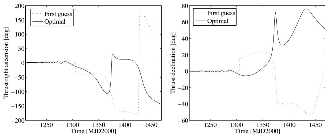
**a)** **Figure 5.37: Angles of the thrust vector.** The dashed line represents the first guess solution; the continuous line is the optimal profile. **a) Right ascension and b) declination.**
