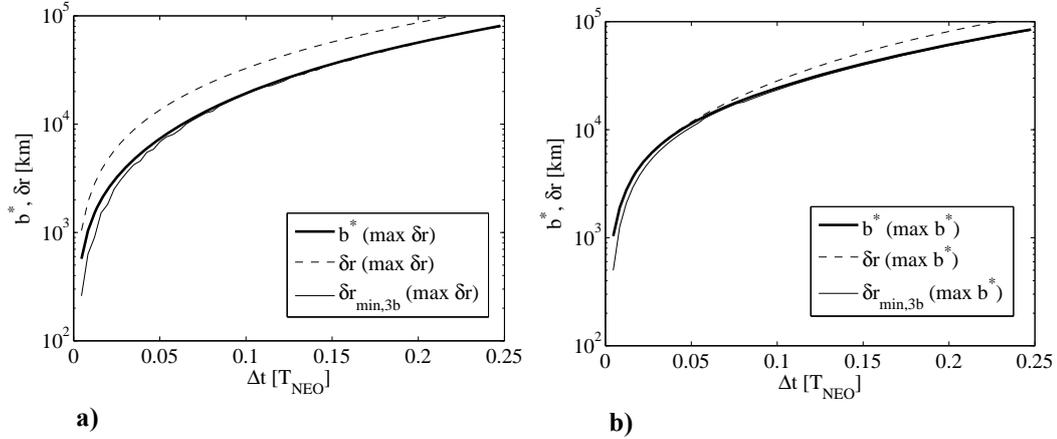
**Figure 2.12: Deviation (dashed line) and its projection (bold line) on the  $b$ -plane calculated through the two-body problem and minimum deviation computed through the three-body problem (continuous thin line): a) maximum deviation strategy for asteroid 1979XB and b) maximum  $b^*$ -parameter strategy for asteroid 1979XB.**
