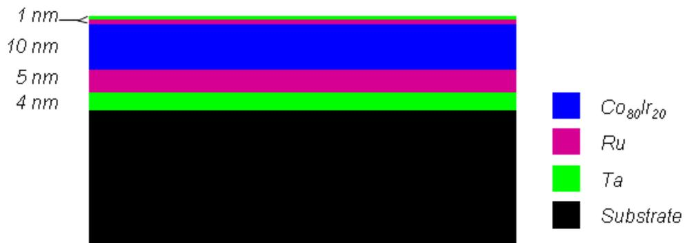
Figure 6.1: Cross-section stacks of the multilayer film system used in the research.
