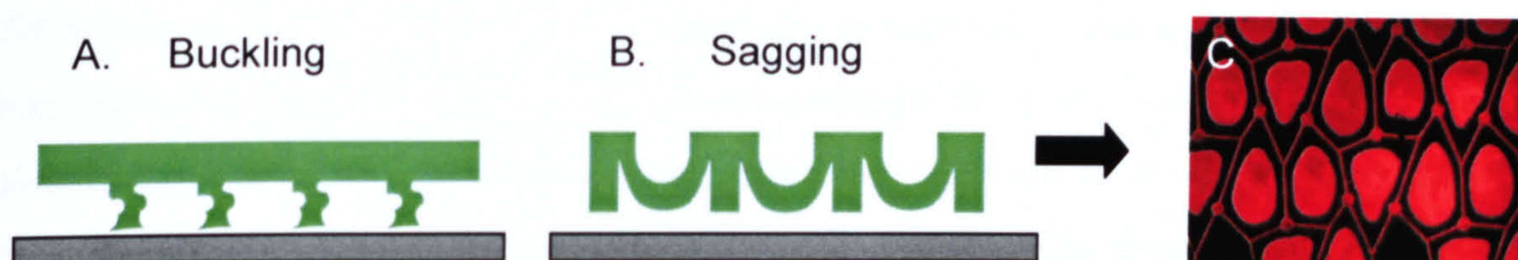
Figure 3.13. Schematic diagram showing the different types of stamp deformation that could potentially cause the result observed during the evaluation of pattern transfer experiment (A, B), and the corresponding fluorescent image illustrating this result (C).
