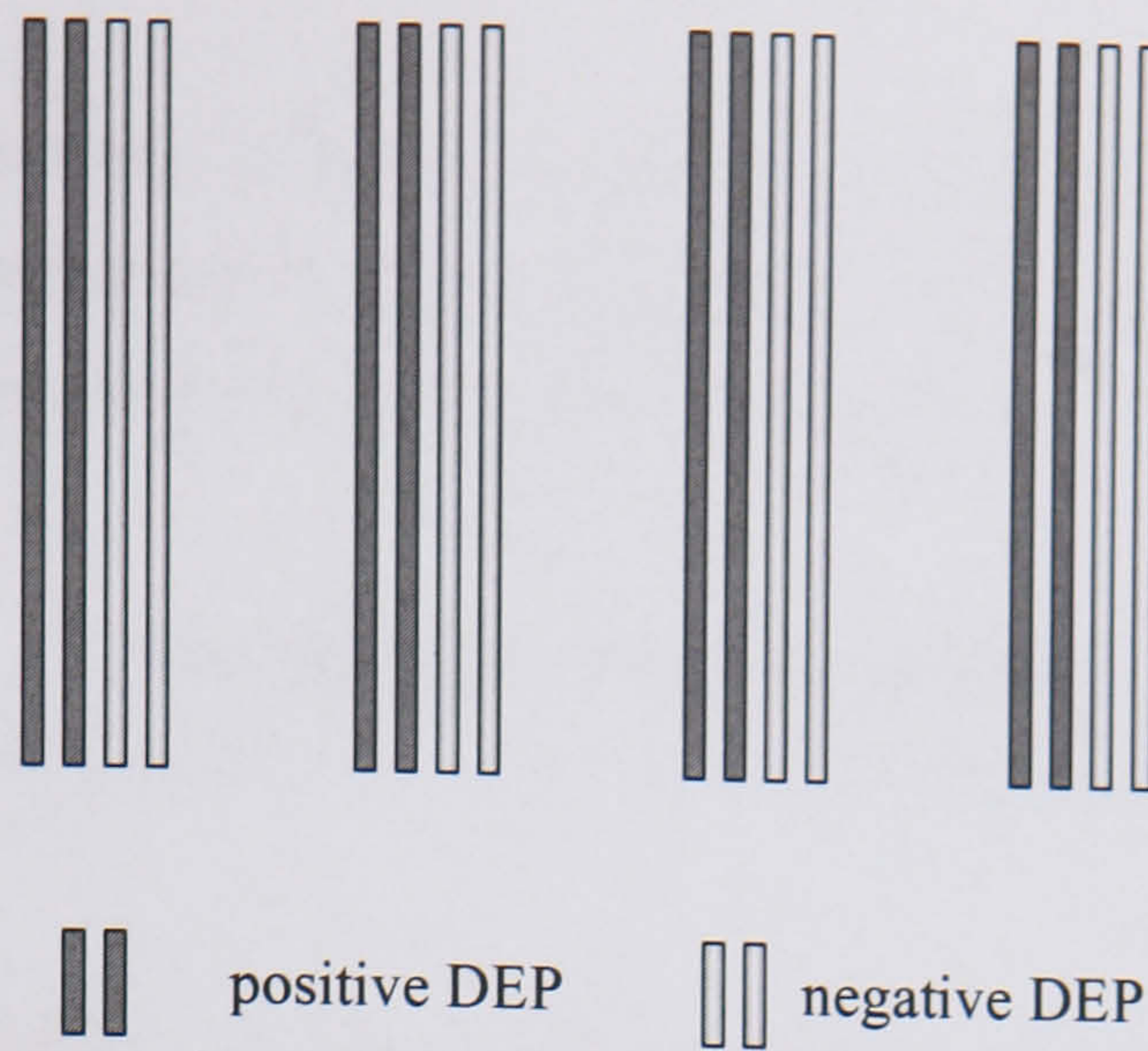
Figure 6-30 4 electrode interdigitated cluster design
