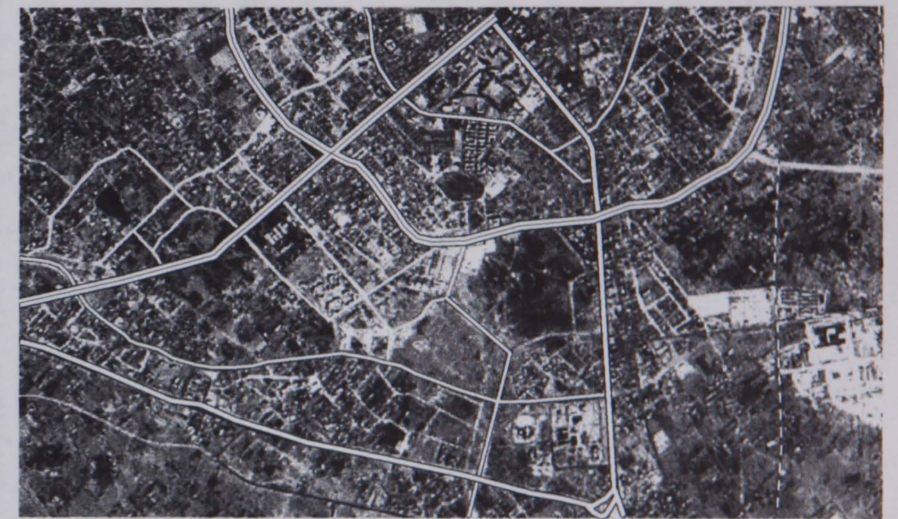
Figure 12-2d: The most appropriate line forms selected to represent the different classes of roads. (1:50,000 scale)
