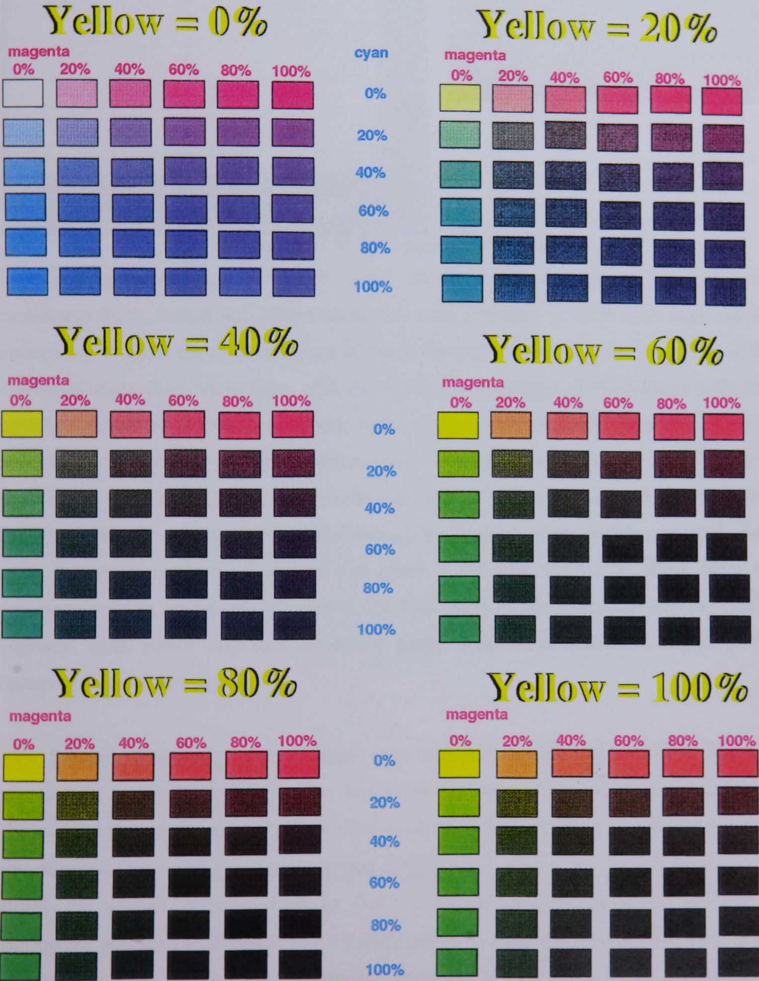
Figure 15-7: ACE process colour chart as printed by the Epson Stylus 1520 colour inkjet printer.
