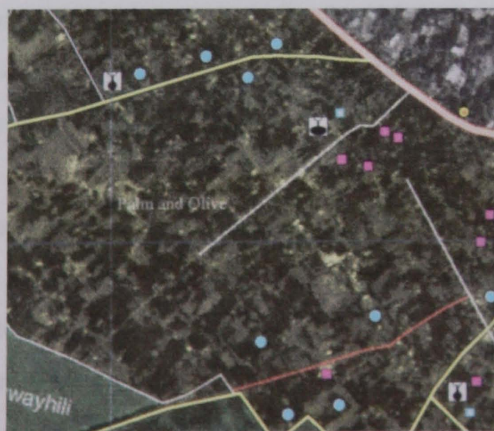
Figure 13-6a: This small window illustrates how over exaggeration of the point symbols (magenta-coloured squares) used to show isolated building may affect the balance and appearance of the map.
