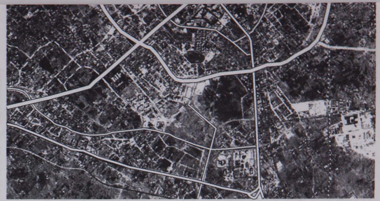
Figure 12-2b: The second line form alternative – single and double lines have been used. (1:50,000 scale)
