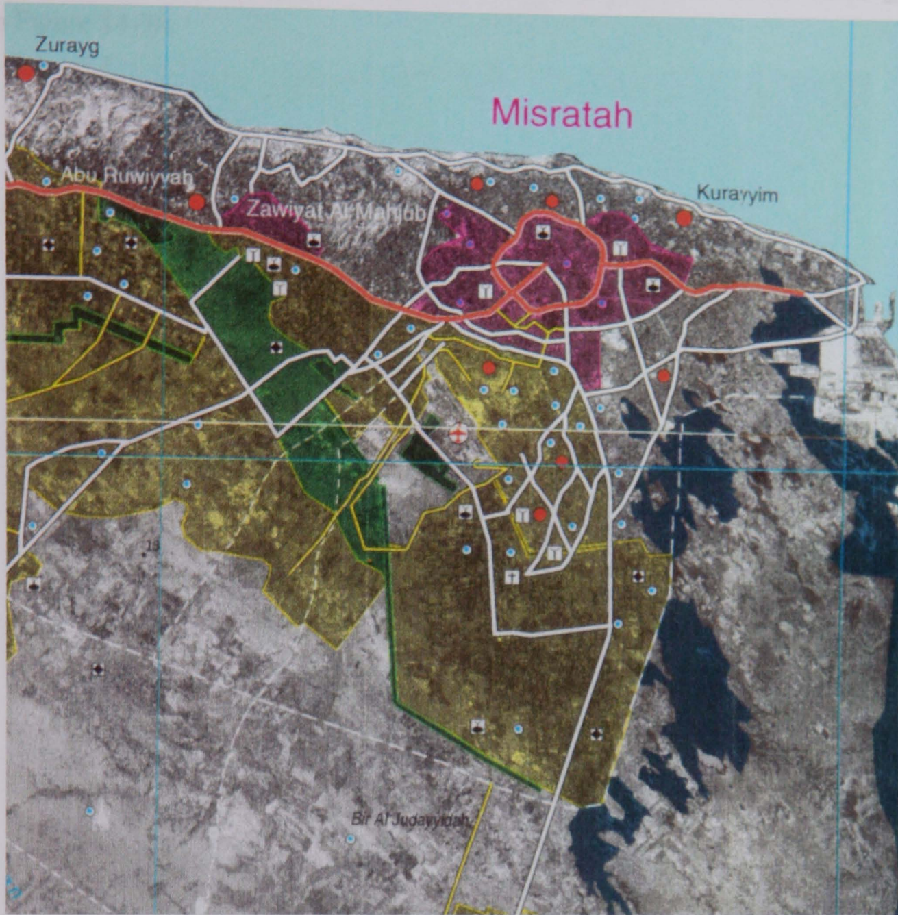
Figure 14-3a: A small window illustrates the representation of towns on the 1:250,000 scale map produced in the current project. As the size of this area feature gets smaller due to scale changes, the percentage of transparent magenta was increased to obtain sufficient visual contrast and clarity.
