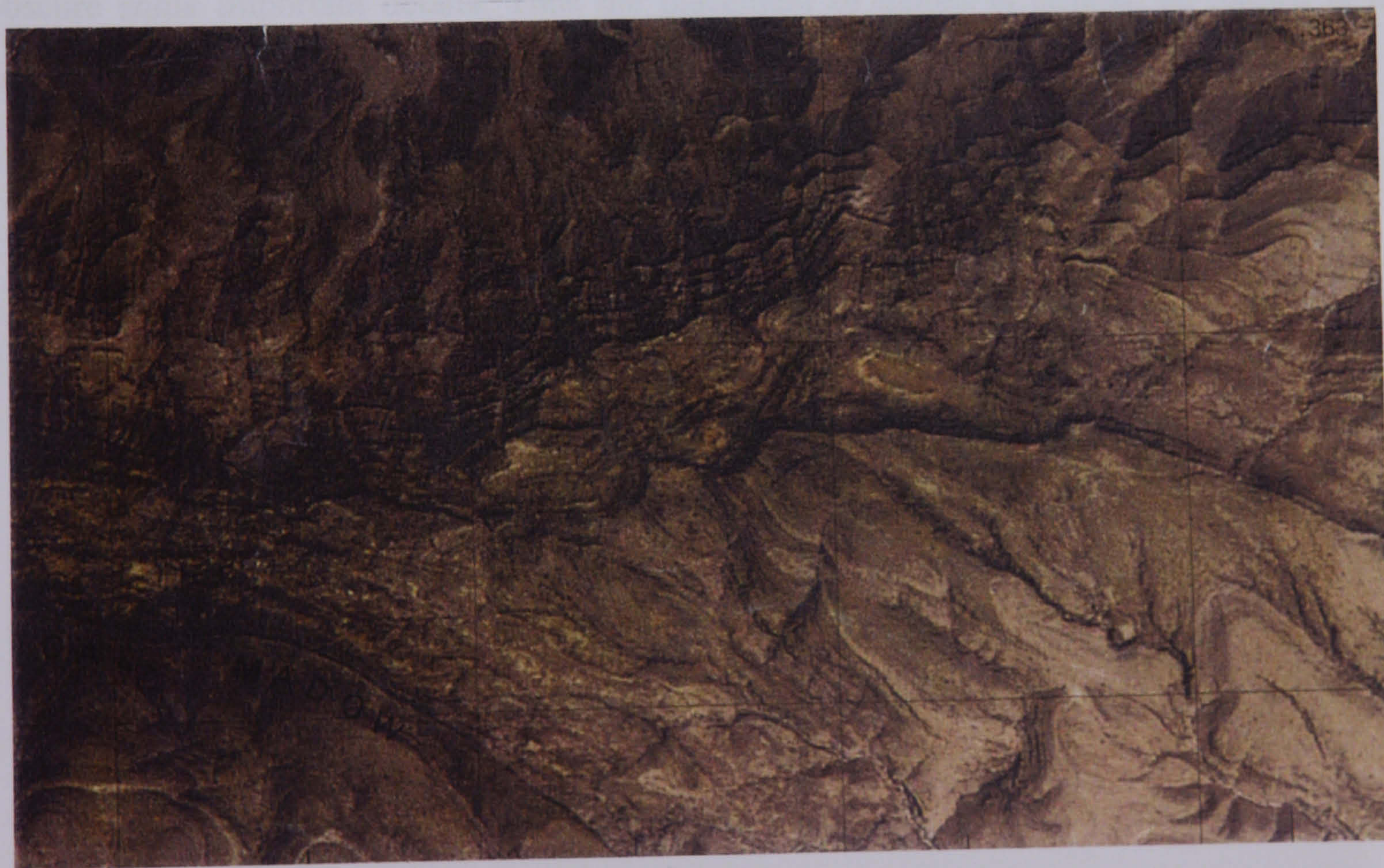
Figure 7-1: A small window from the Laag space image map in Somalia at 1:50,000 scale showing the problem of insufficient contrast (tonal variation) caused by shadow in this hilly area. The map fragment illustrated is virtually indecipherable. Note also that the black grid is almost invisible. (Map 29 in Chapter 6)
