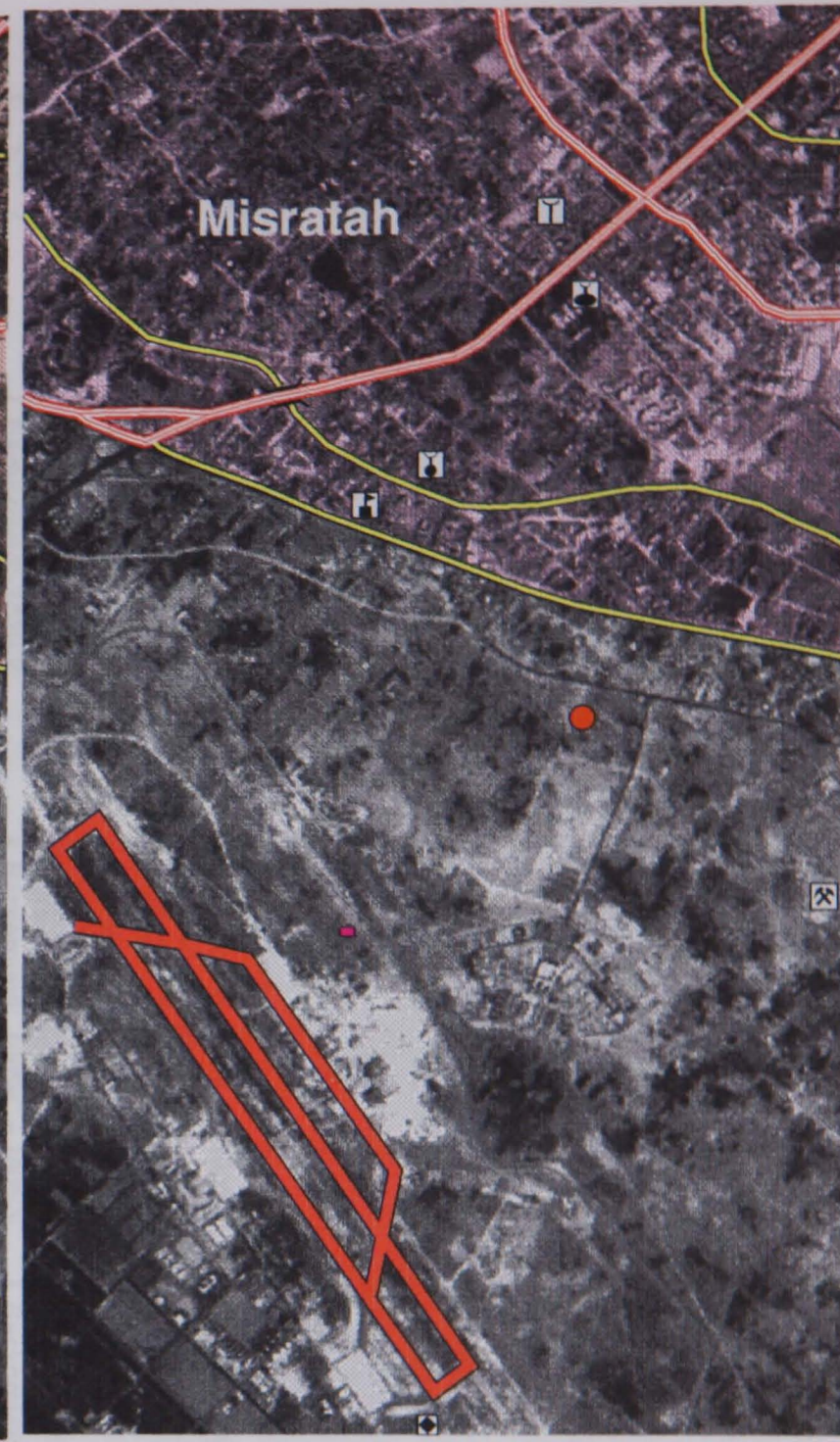
Figure 12-5i: The selected colours for the various classes of cultural features. (1:50,000 scale)
