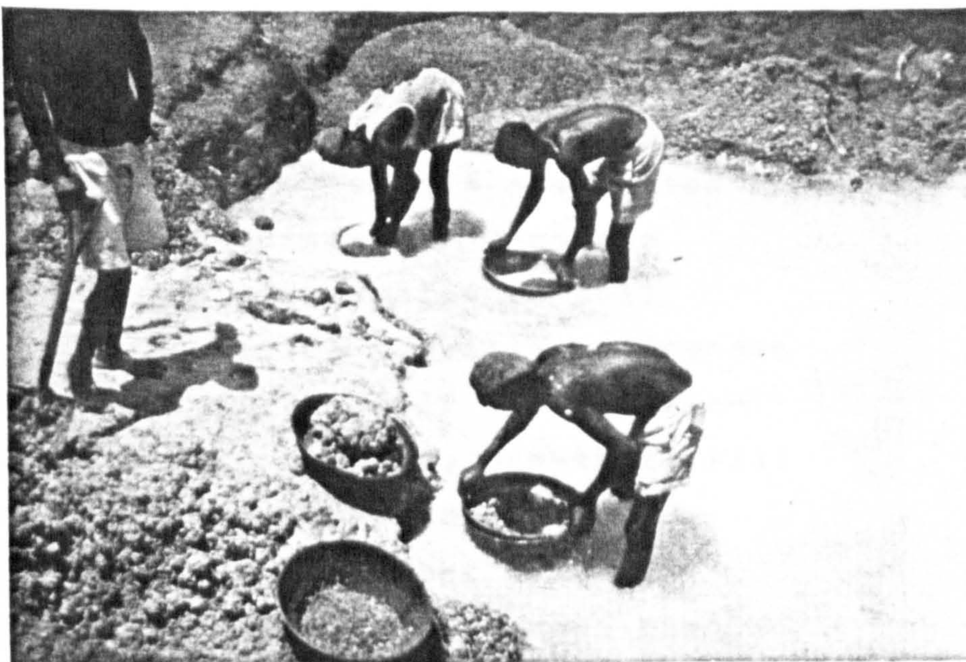
Illustration 21: The back-breaking task of washing gravel by the long-standing method of panning, typical of alluvial mining booms everywhere, is closely supervised by the gangmaster (standing). The diamond bearing gravel before washing is in the right-hand pan and the concentrate in the left-hand one in the foreground of the picture: Yomandu, Sando Chiefdom, Kono District (October 1968).
