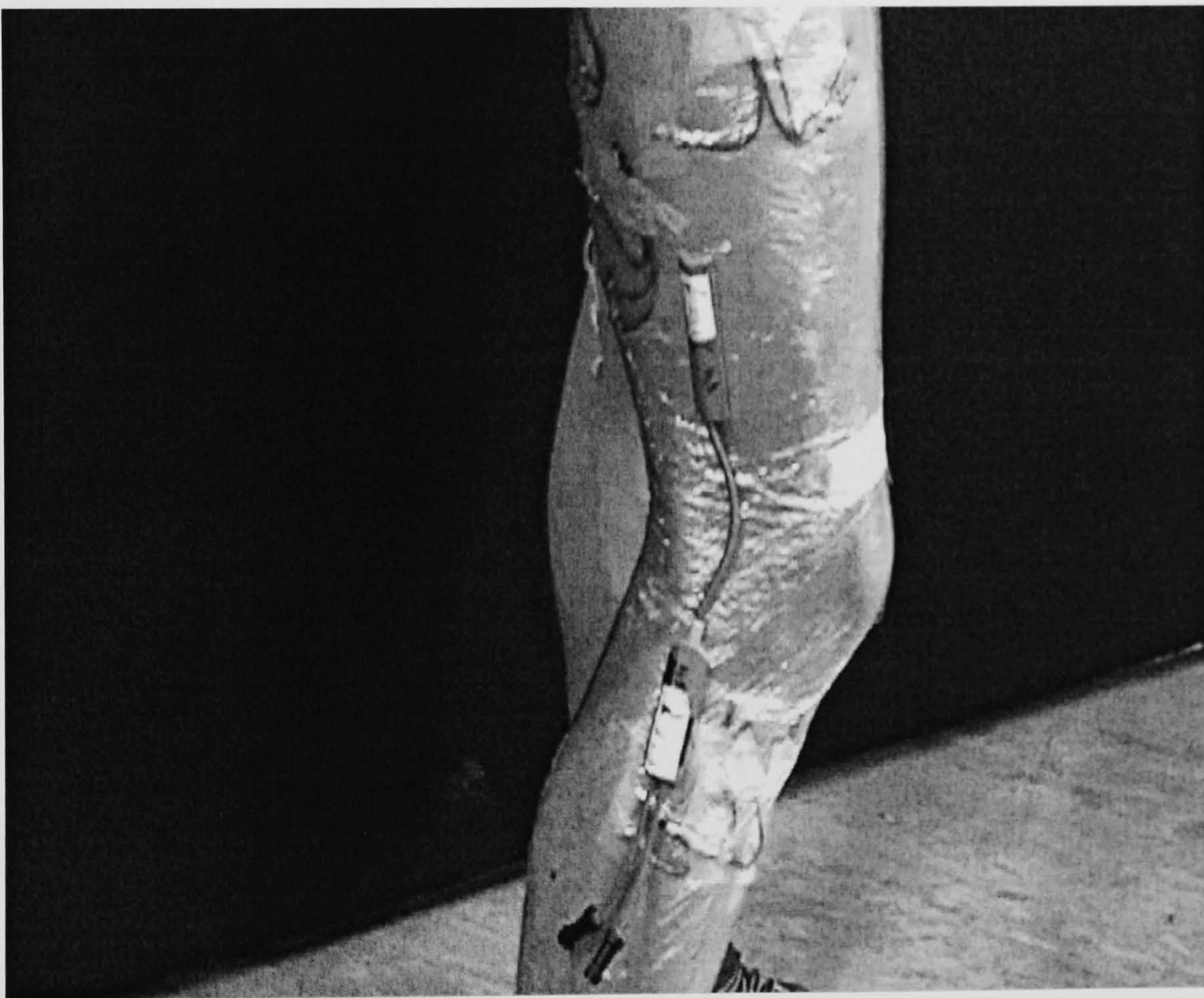
Figure 2.3. The figure shows the electrogoniometer fixed on the lateral aspect of the knee joint.
