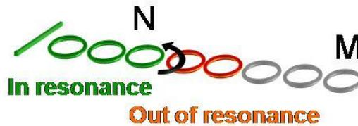
(c) Schematic representation of the ring on resonance (green) and off resonance (red).
