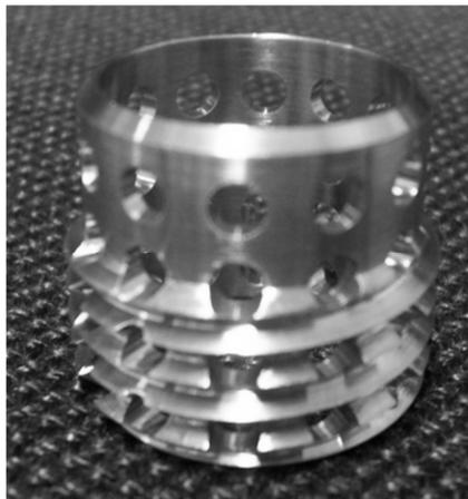
**Figure 14: Photograph of a Kerf Cut Cylinder.**
