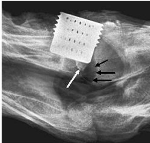
**Figure 26: Post testing latero-lateral radiograph of the C4-C5 articulation from group 1. Left is cranial, top is ventral. Black arrows indicate the caudal end of the fracture line; white arrow shows the fracture fragment from the cranial body of C5.**
