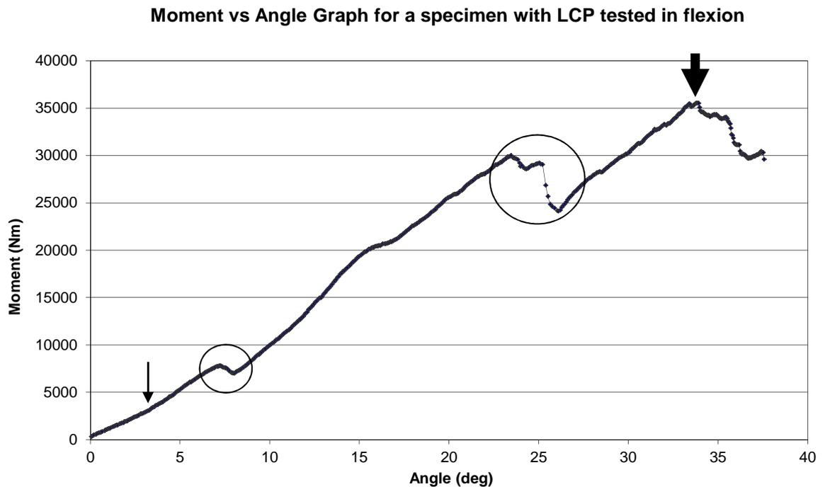
**Figure 41: Moment vs. angle graph from a specimen in the LCP group in flexion demonstrating the alterations in stiffness. Nm = Newton meter, deg = degree. The changes in stiffness at 8° and 25° (circled) corresponded with screw slippage from the construct. The change from the “toe-region” to the construct stiffness is highlighted by the thin arrow. The failure point is highlighted by the thick arrow.**
