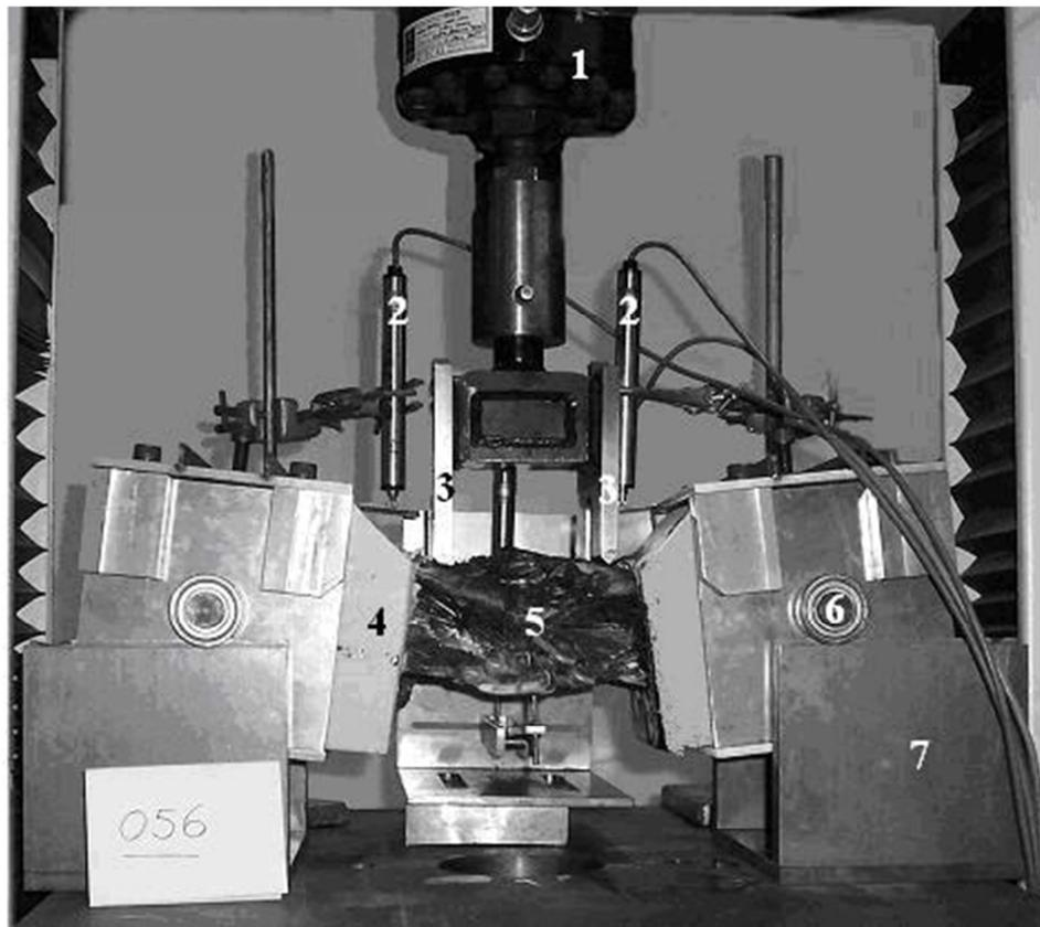
**Figure 30: Cervical vertebrae secure in the load cell before testing (Left = cranial, Top = ventral). 1: Load cell; 2: LVDT; 3: Inner Support Points; 4: Resin Block; 5: Specimen; 6: Pivot Wheel / Outer Support; 7: Support.**
