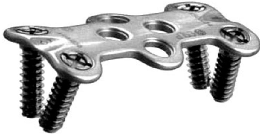
**Figure 3: A “Synthes” cervical locking plate using fixed angle screws, locked to the plate with secondary inner set screws.**
