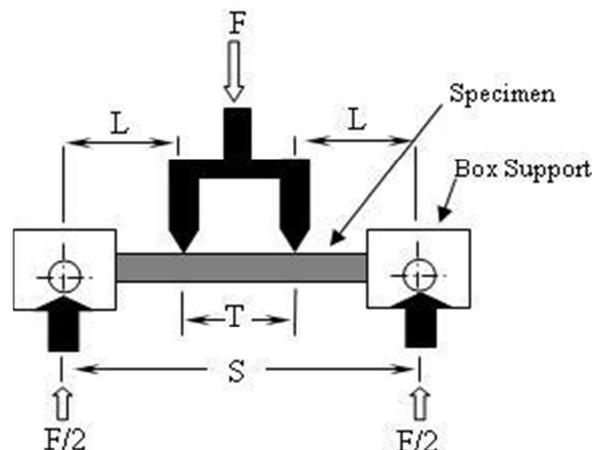
**Figure 31: Diagram representing the forces applied through the test apparatus:  $F$ = force (yield load or failure load) applied to the specimen;  $L$  = distance from the outer to the inner support;  $S$  is the distance between the outer supports;  $T$  is the distance between the inner supports.**
