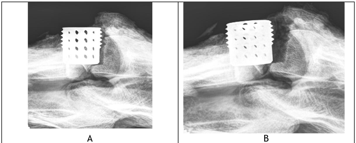
**Figure 42: Radiographs post mechanical testing. A=in neutral position; B=with specimen in stressed position, highlighting the fracture site.**
