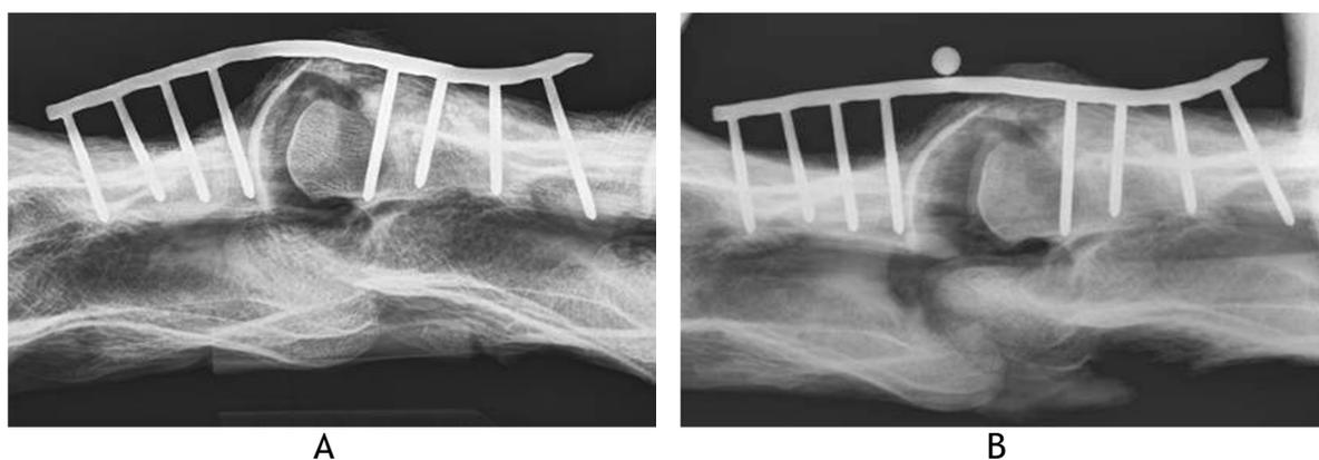
**Figure 28: Radiographs before (A) and after (B) testing of a 3.5mm Locking Compression Plate demonstrating plate deformation.**
