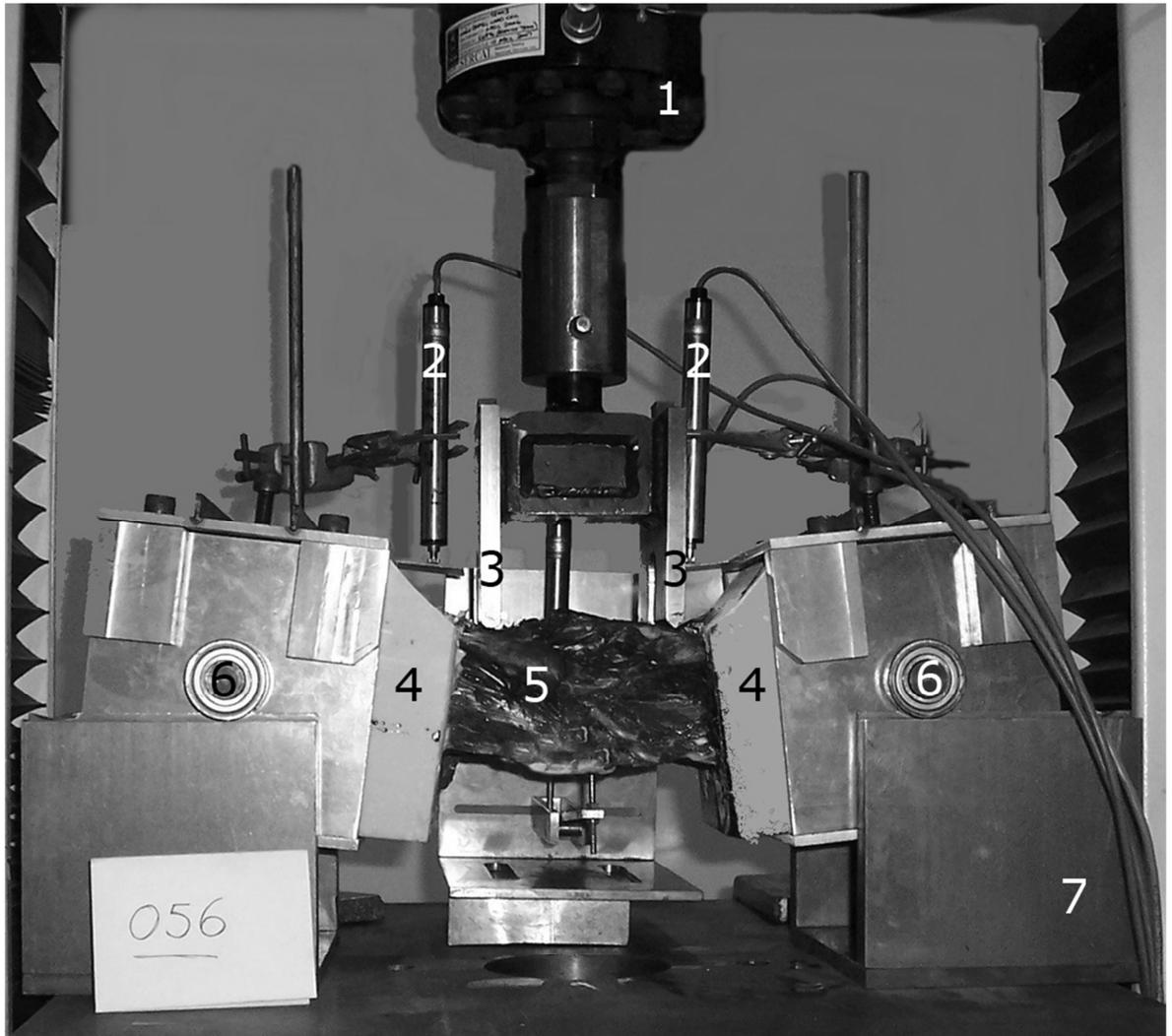
**Figure 18: A spine secure in the load cell prior to testing. 1: Load cell; 2: LVDT; 3: Inner Support Points; 4: Resin Block; 5: Specimen; 6: Pivot Wheel / Outer Support; 7: Support.**
