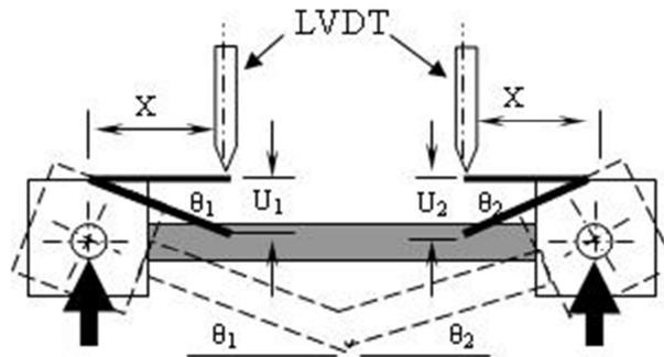
**Figure 32: Diagram representing the angular displacement of the specimen.  $U_1$  and  $U_2$  represent the displacement of the LVDT's,  $X$  is the distance of the LVDT from the pivot point of the outer support and  $\theta_1$  and  $\theta_2$  represent the rotations at each support.**
