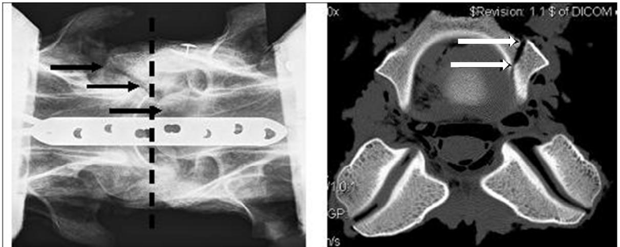
**Figure 39: Post testing DV radiograph (Left of image = cranial) and CT (Top of image = ventral) scan of specimen from the LCP group that failed during lateral flexion. Black and white arrows highlight the fracture line on the compression side, extending from the left lateral caudal articular surface at the intercentral articulation to the left lateral vertebral body just caudal to the lateral process. The dashed line represents the level of the CT slice (right hand image).**
