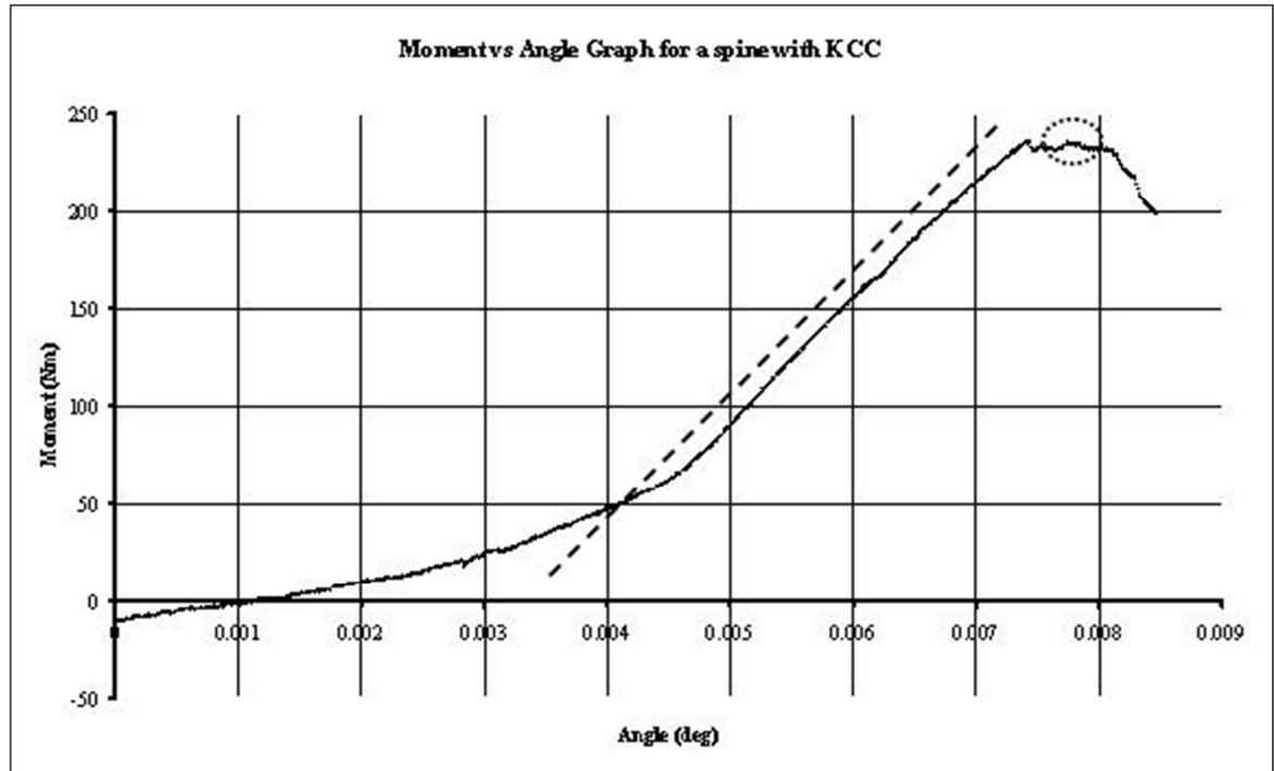
**Figure 23: Moment vs. angle graph from Group 1 demonstrating initial shallow incline followed by steeper incline. Dashed line represents the stiffness of the construct; dotted circle represents the failure point. Nm = Newton meter, deg = degree.**
