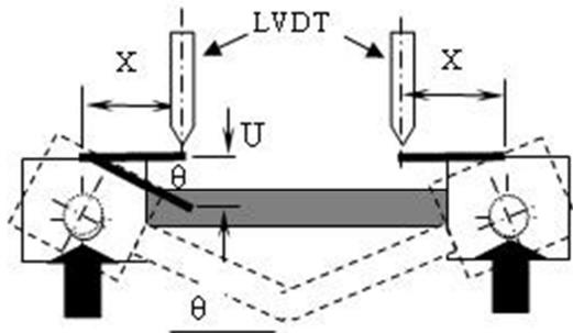
**Figure 20: Diagram representing the angular displacement of the specimen. LVDT = linear variable differential transformer;  $\theta$  = angular displacement; U = displacement of the LVDT and X = offset of the LVDT from the pivot support,  $\theta_T$  = total rotational displacement of the joint and  $\theta_1$  and  $\theta_2$  = rotations at each support.**
