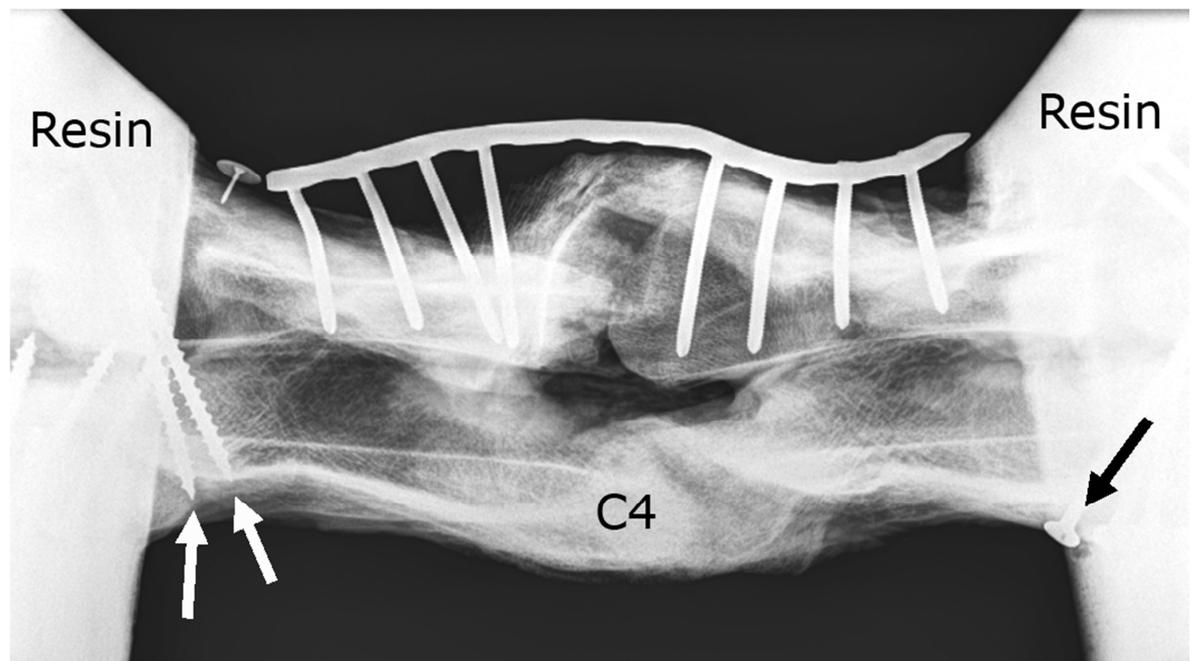
**Figure 17:** A spine fixed in resin post testing. White arrows point to the tips of the two 100mm screws extending from cranioventral to caudodorsal across the C3-C4 intervertebral disc. The black arrow points at one of the fixation screws extending from craniomedial to caudolateral across the centre of one of the articular process joints between C5 and C6.
