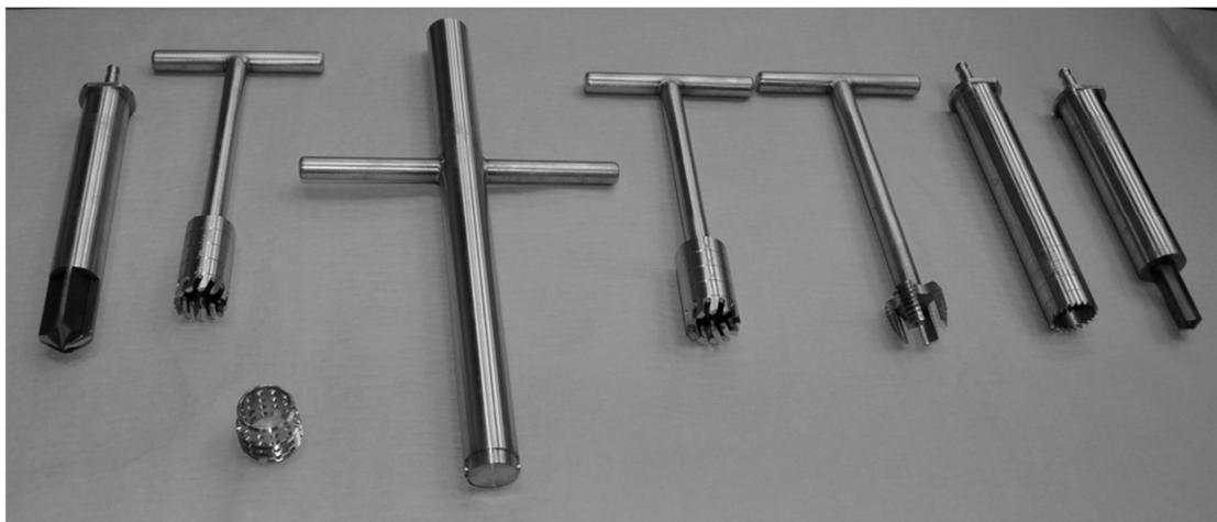
Figure 16: Equipment required for Kerf cut cylinder placement.
