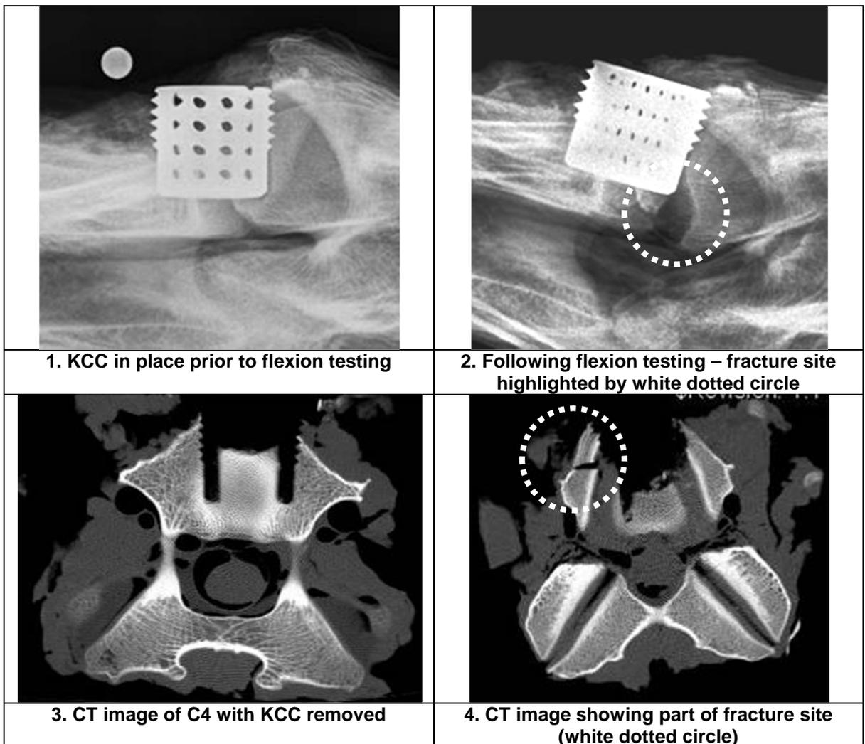
Figure 36: Radiographs and CT images demonstrating some of the Kerf Cut Cylinder failure modes.
