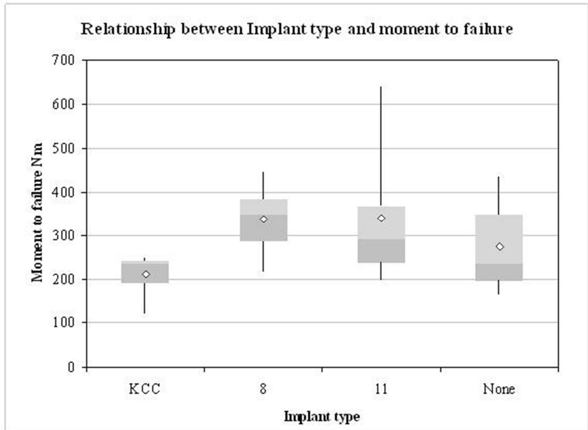
**Figure 24: Relation of group with respect to moment to failure. Centre line is the median; interquartile ranges and total ranges are represented by the box and whiskers respectively. White diamonds represent the mean.**
