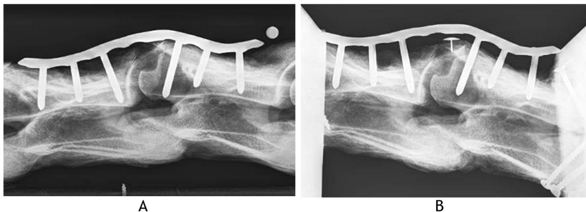
**Figure 27: Radiographs before (A) and after (B) testing of a 4.5mm Locking Compression Plate demonstrating screw pull out.**
