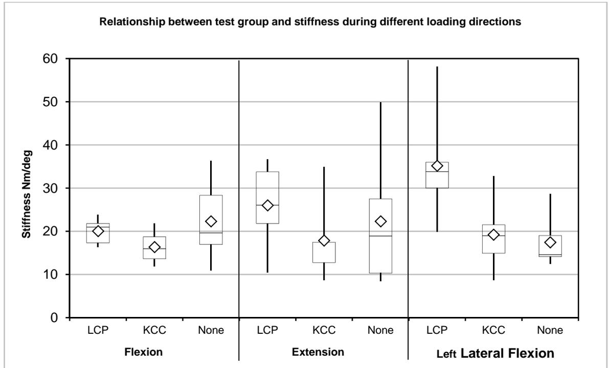
**Figure 34: Relation of group and loading direction with respect to stiffness. Centre line is the median; interquartile ranges and total ranges are represented by the box and whiskers respectively. White diamonds represent the mean. KCC = Kerf Cut Cylinder; LCP = Locking Compression Plate; Nm = Newton meter; deg = degree.**
