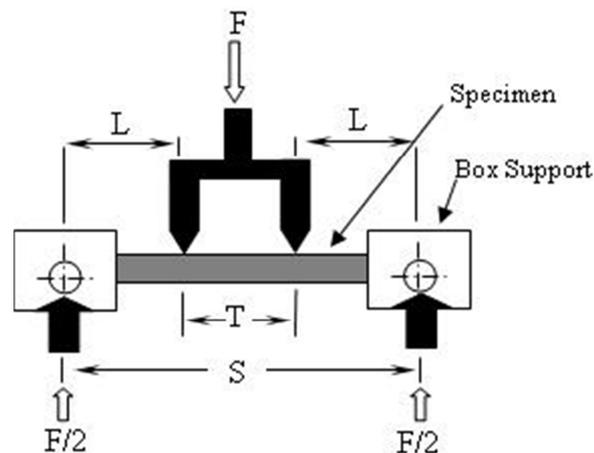
**Figure 19: Diagram representing the forces applied through the test apparatus.  $F$  = force (yield load or failure load) applied to the specimen;  $L = (S-T)/2$ ;  $S$  = distance between the outer supports and  $T$  = distance between the loading edges.**
