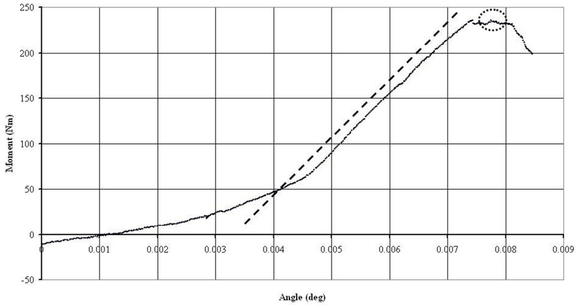
**Figure 33: Moment vs. angle graph from Group 1 demonstrating “toe-region” followed by steeper incline. Dashed line represents the stiffness of the construct; dotted circle represents the failure point. Nm = Newton meter, deg = degree.**
