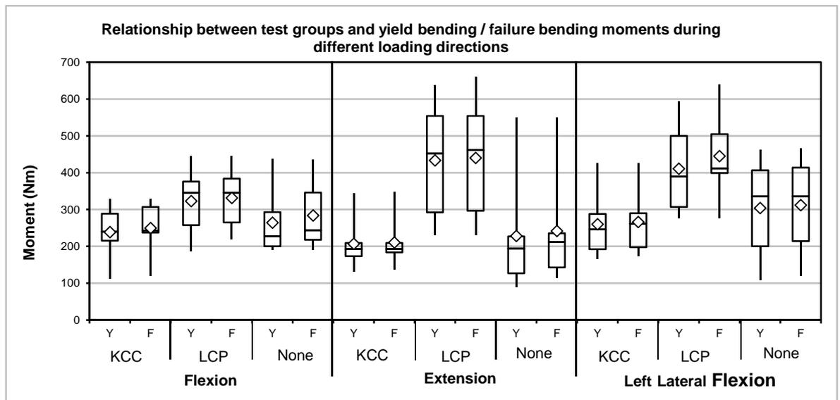
**Figure 35: Relation of group and loading direction with respect to yield bending and failure bending moments. Centre line is the median; interquartile ranges and total ranges are represented by the box and whiskers respectively. White diamonds represent the mean. Y = Yield bending moment; F = Failure bending moment; KCC = Kerf Cut Cylinder; LCP = Locking Compression Plate; Nm = Newton meter.**
