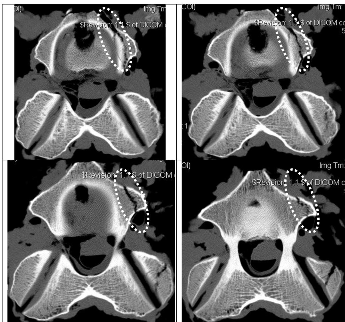
**Figure 37: Sequential CT images demonstrating the fracture site following testing of a specimen with a LCP implant. The fracture occurred in a sagittal plane along the caudal inter-central articulation of C4. Images run sequentially from left to right in a cranial to caudal progression. Fracture highlighted by a white dotted ellipse.**
