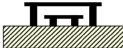
i) Lift-off the photoresists and etch the Ti/Au seed layer
