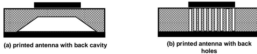
**Figure 2 - 18 :** Techniques used to synthesize a low dielectric constant by etching the substrate.
