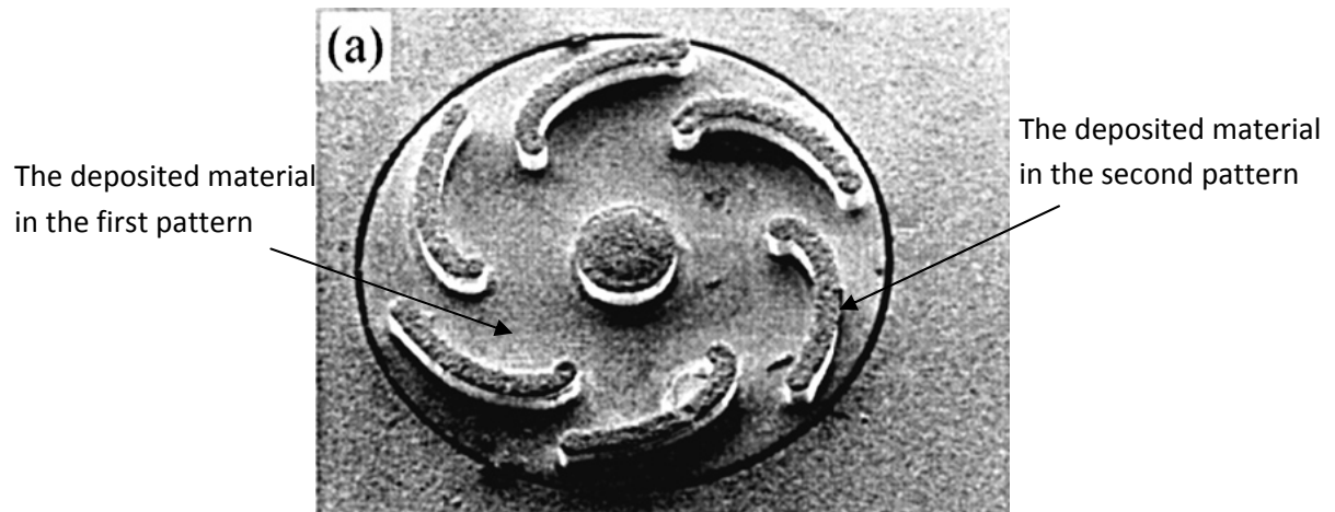
Figure 36 a turbine which was produced with six levels [98]
