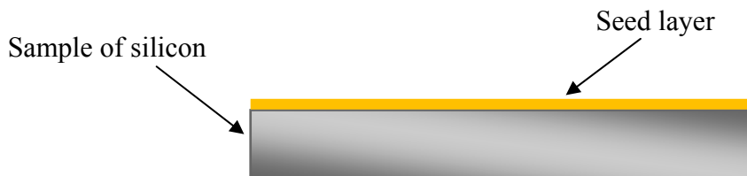
Figure 48 depositing a seed layer
