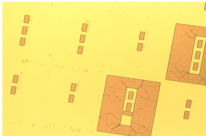
Figure 73 removing of the SU 8
