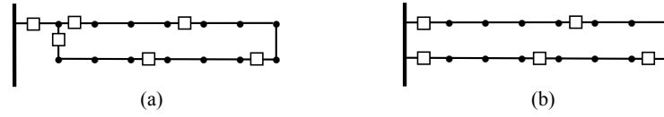
Figure 6.3: Illustration of device redundancy of collection string switchgear configuration.
