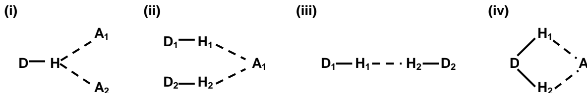
Figure 1-2 Examples of BHBs (i) One donor, one H atom and two acceptor atoms (DHAA), (also referred to as three- centred in the literature) (ii) Two donors, two H atoms and one acceptor atom (DDHHA) (iii) Two donors, with two H atoms between and no acceptor atoms (DHHD) (iv) One donor, two H atoms and one acceptor atom (DHHA).
