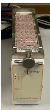
Figure 2-12 The ReactArray Microvate, a device designed to allow temperature programmable crystallisation regimes
