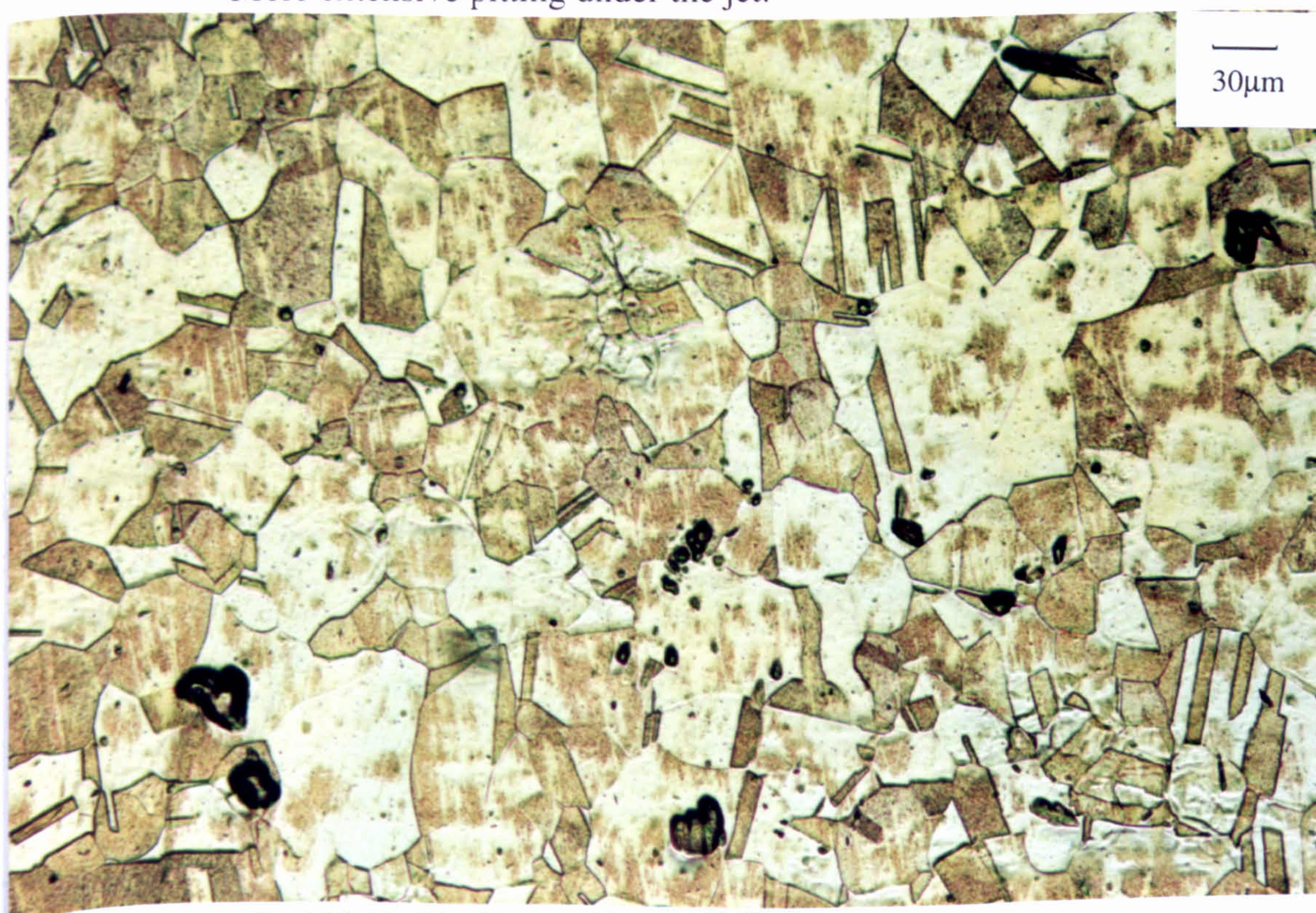
Figure 6.48. Cu-10%Ni, V=86\text{m/s} , 8 hours, T.W.L. The grain structure with a few pits even at the outer regions.
