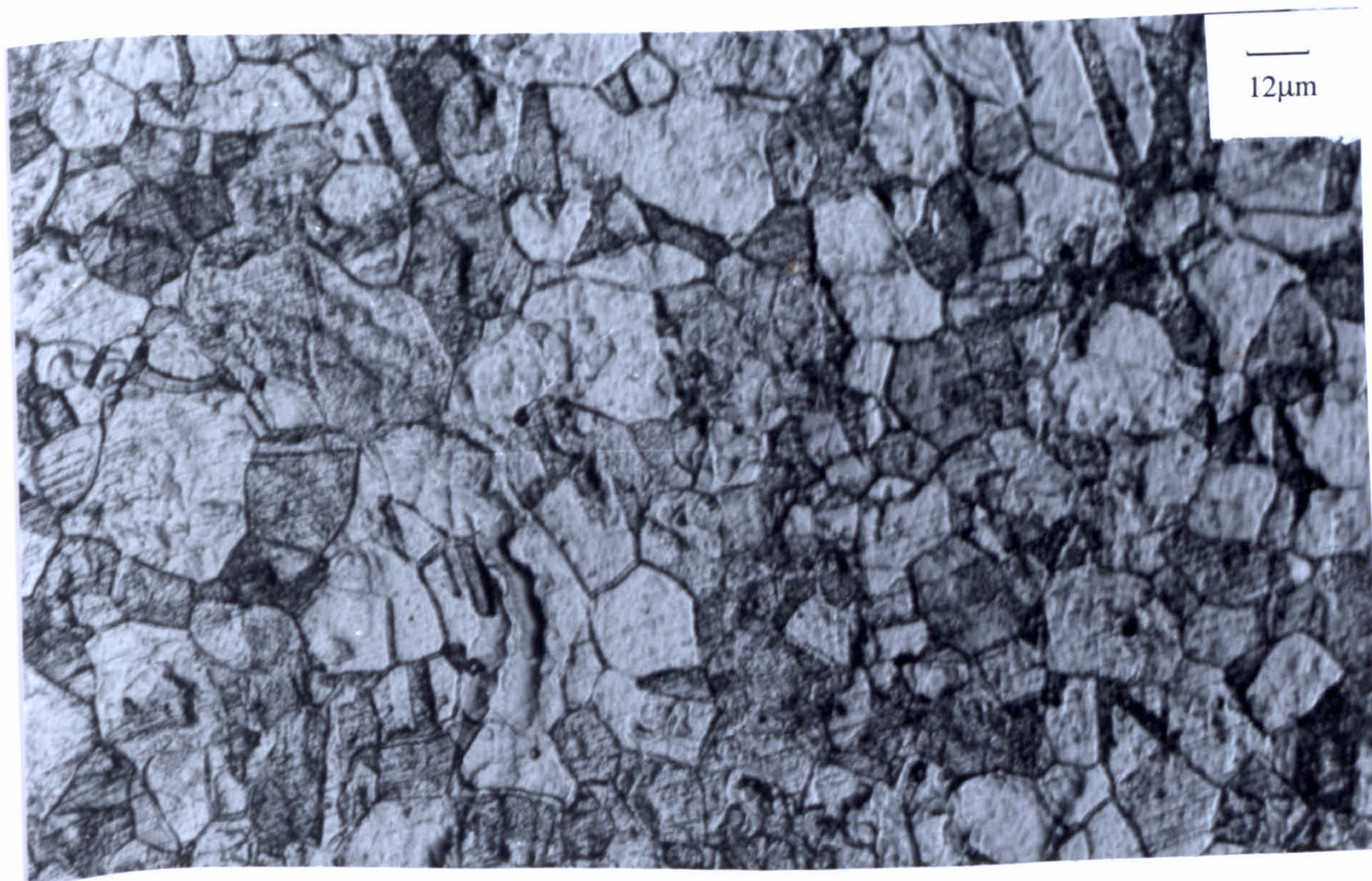
Figure 6.40. Cu-10%Ni, V=17\text{m/s} , 48 hours, T.W.L. The etched appearance was obvious for the whole surface.
