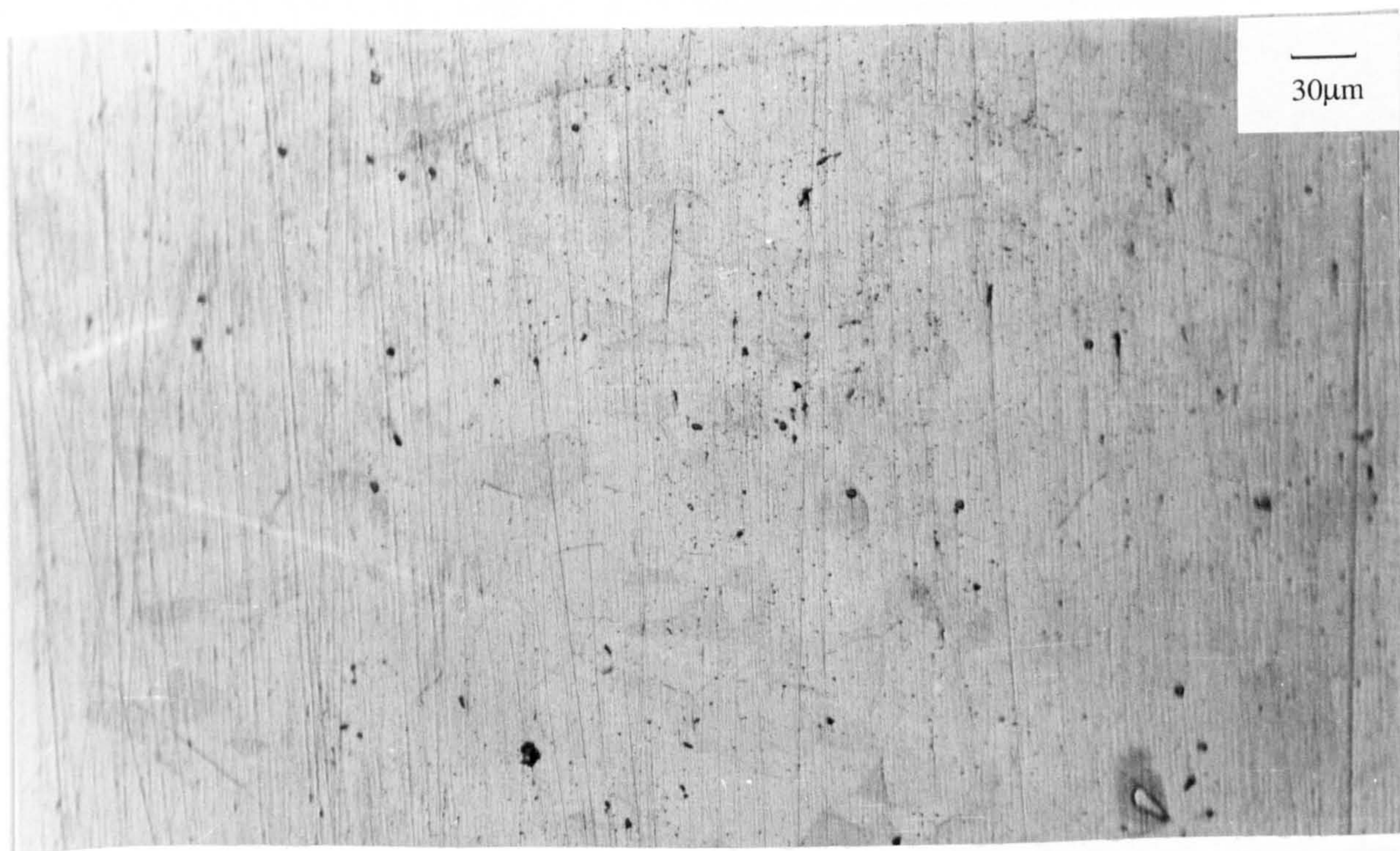
Figure 6.30. Cu-10%Ni, V=4.5\text{m/s} – 1mm nozzle, 4 hours, T.W.L. Numerous shallow pits appeared just under the jet.
