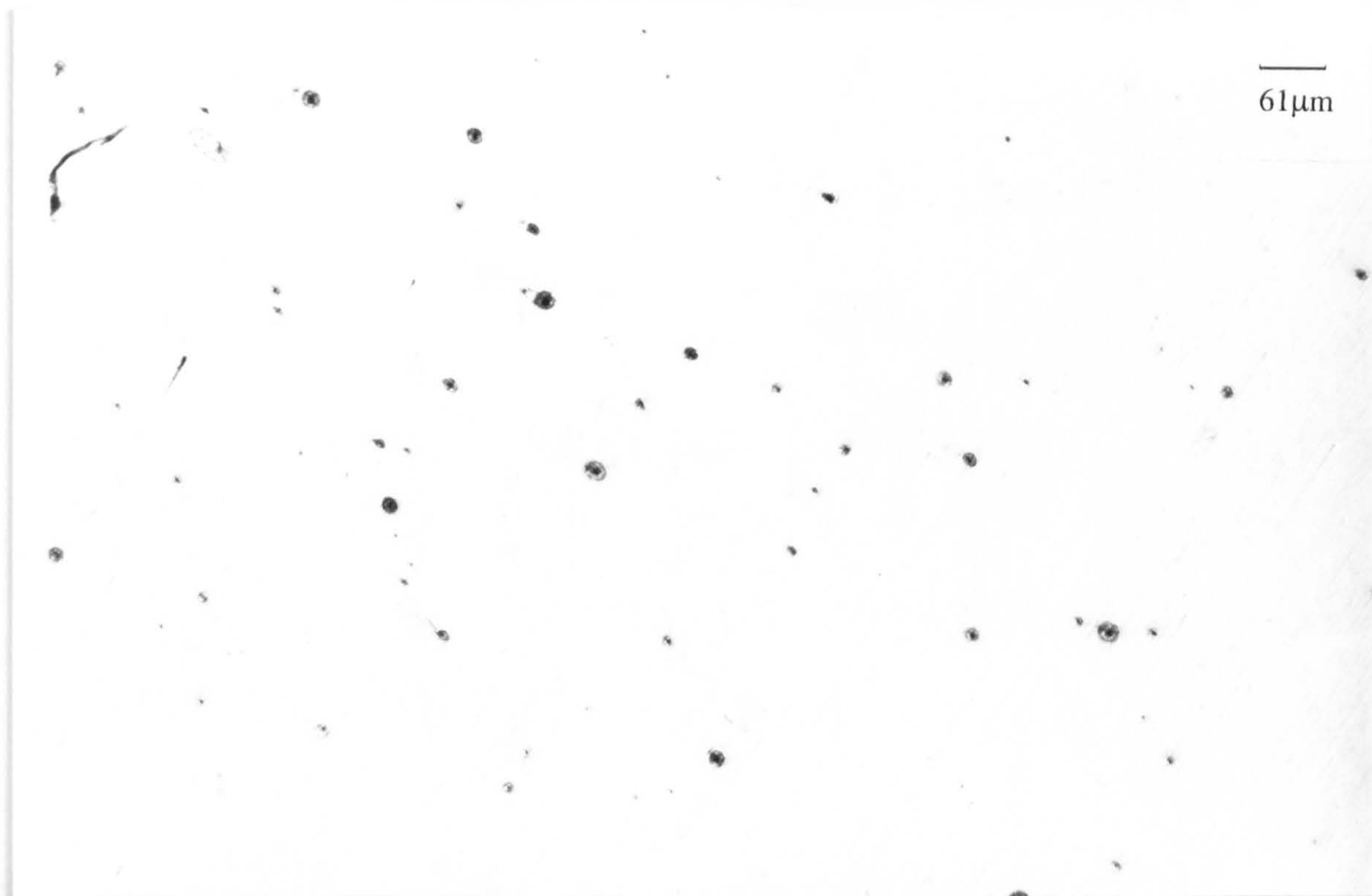
Figure 6.87. Marinel, V=17\text{m/s} , 8 hours, C.P. The area outside the directly impinged zone with some pits and comets.
