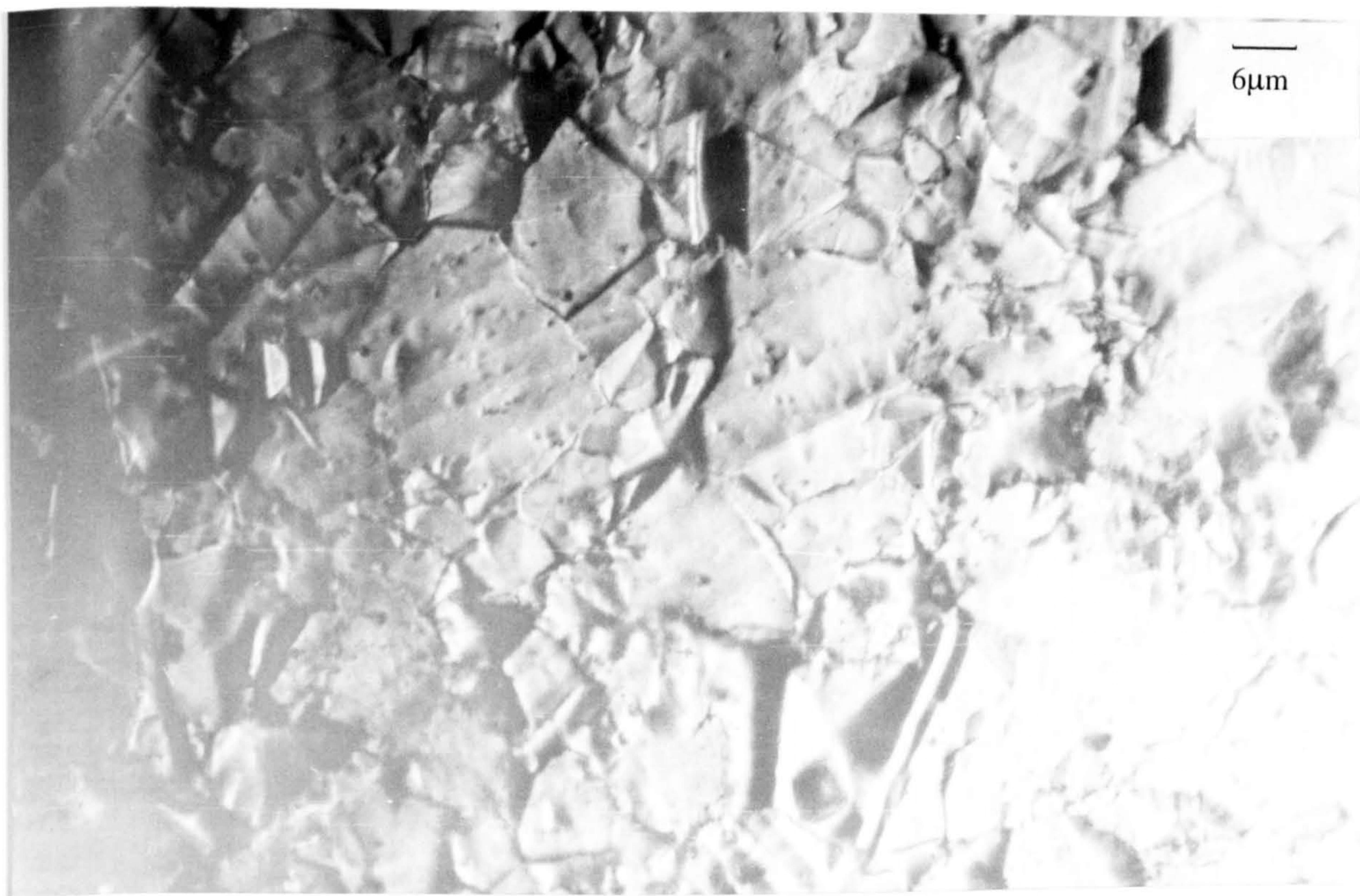
Figure 6.116. Marinel, V=17\text{m/s} , 1 hours, A.R. The etched structure with some pits were evident everywhere.
