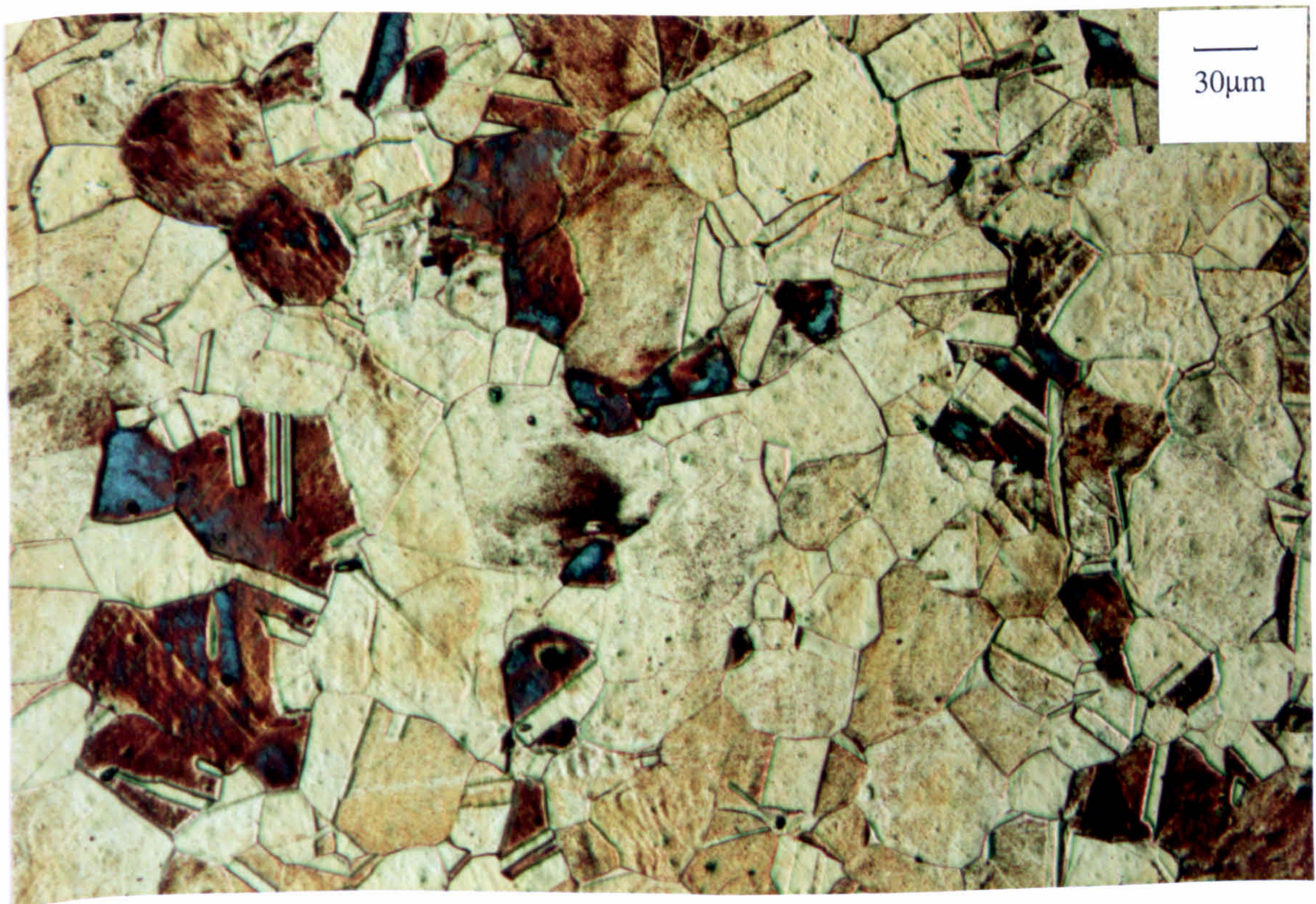
Figure 6.54. Cu-10%Ni, V=86\text{m/s} , 8 hours, A.P. The etched structure at the outer regions of the specimen.
