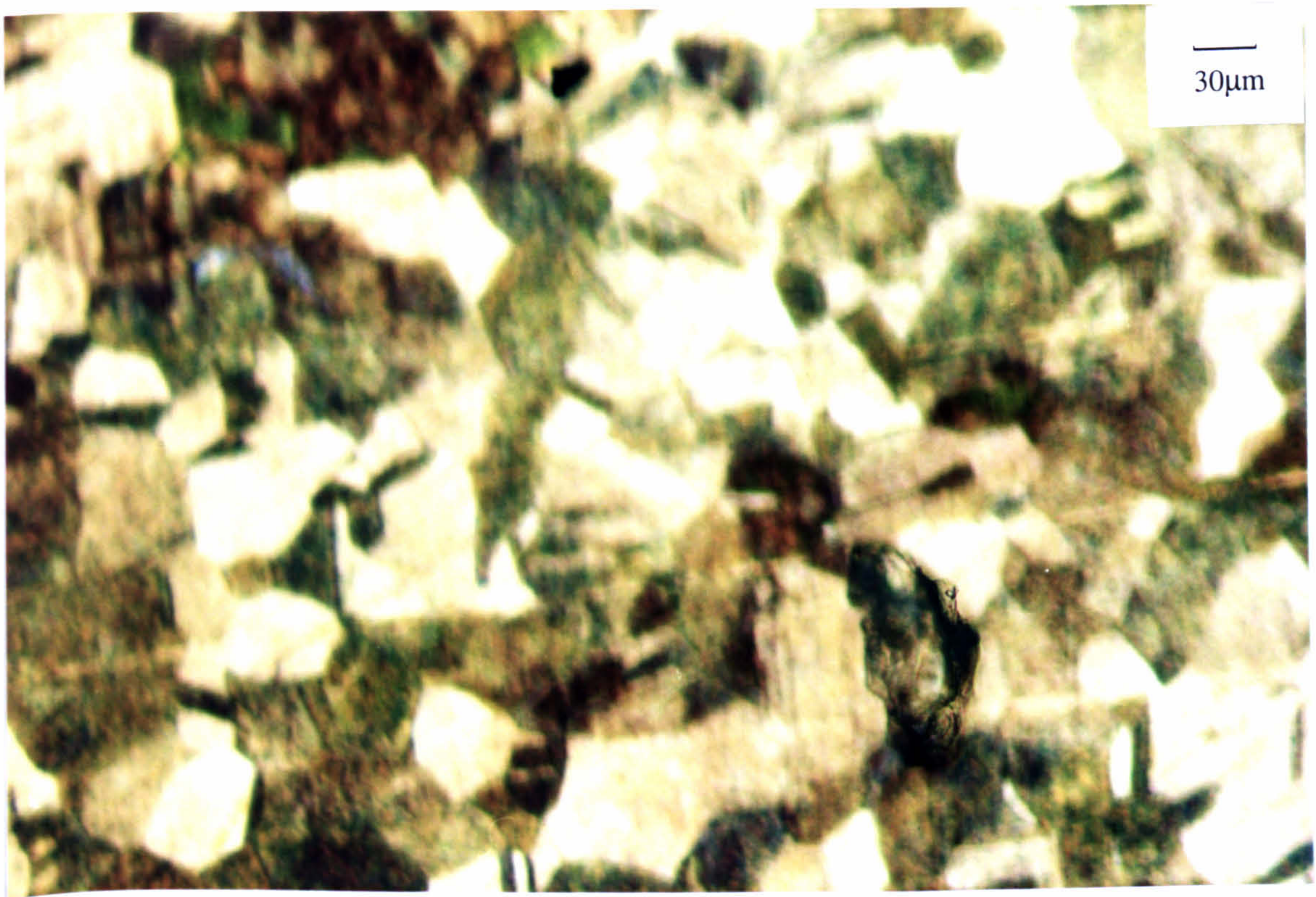
Figure 6.43. Cu-10%Ni, V=86\text{m/s} , 4 hours, T.W.L. The grain structure with a few pits at the outer regions.
