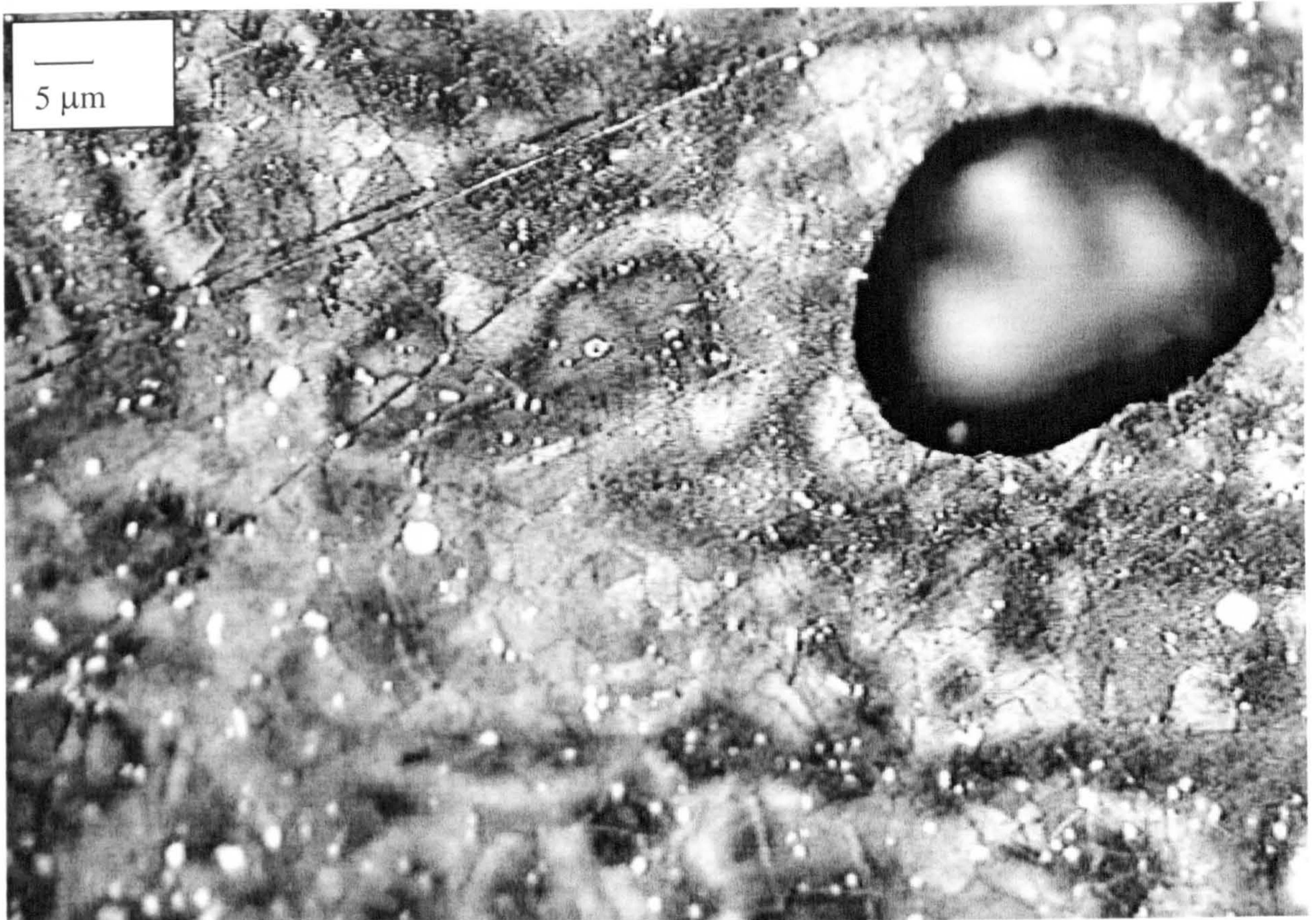
Figure 6.94. Marinel, V=17\text{m/s} , 48 hours, A.P. Some pits at the outside with a deep one out of focus.
