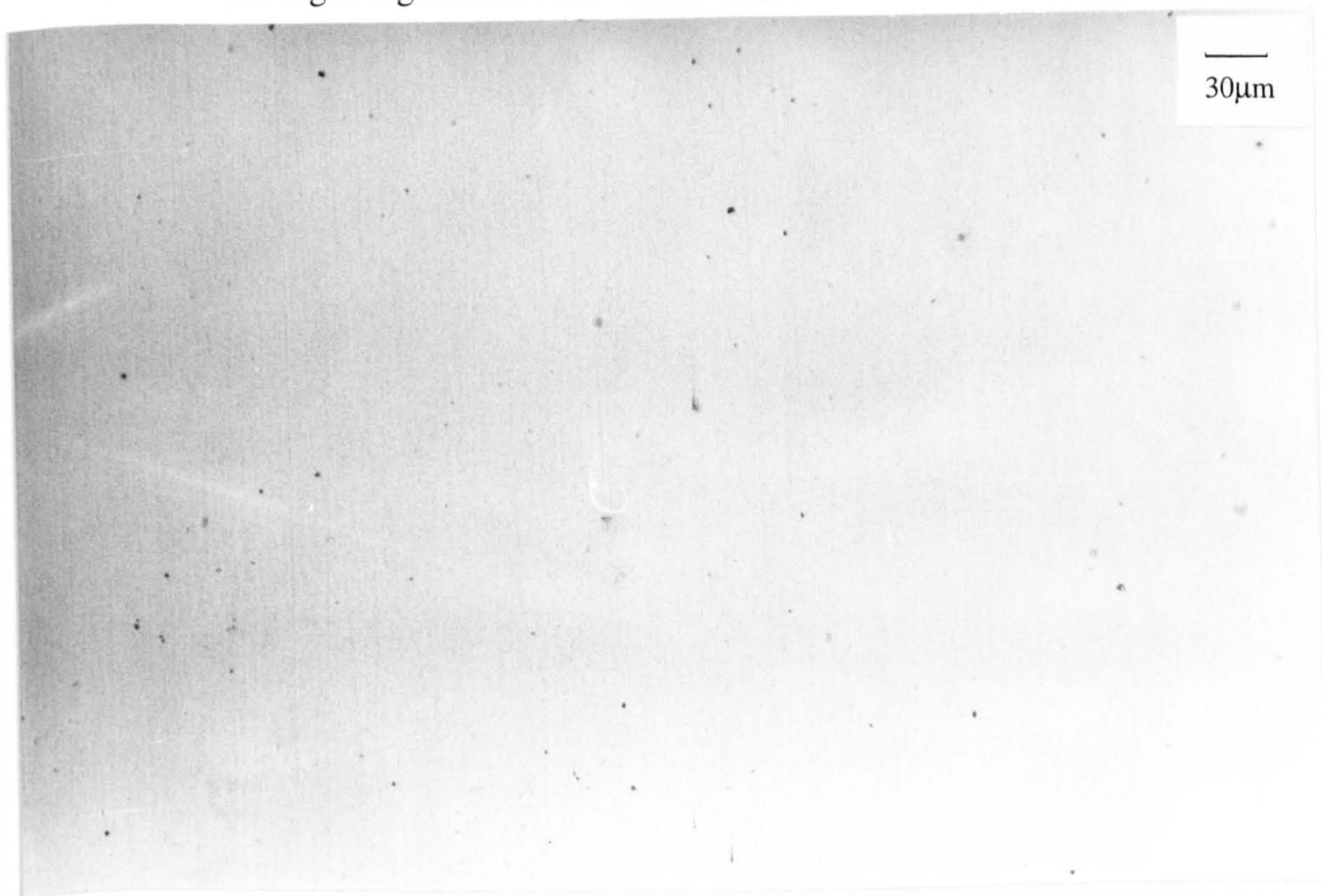
Figure 6.71. Marinel, V=4.5\text{m/s} – 4mm nozzle, 4 hours, C.P. Negligible attack on the surface of the specimen.
