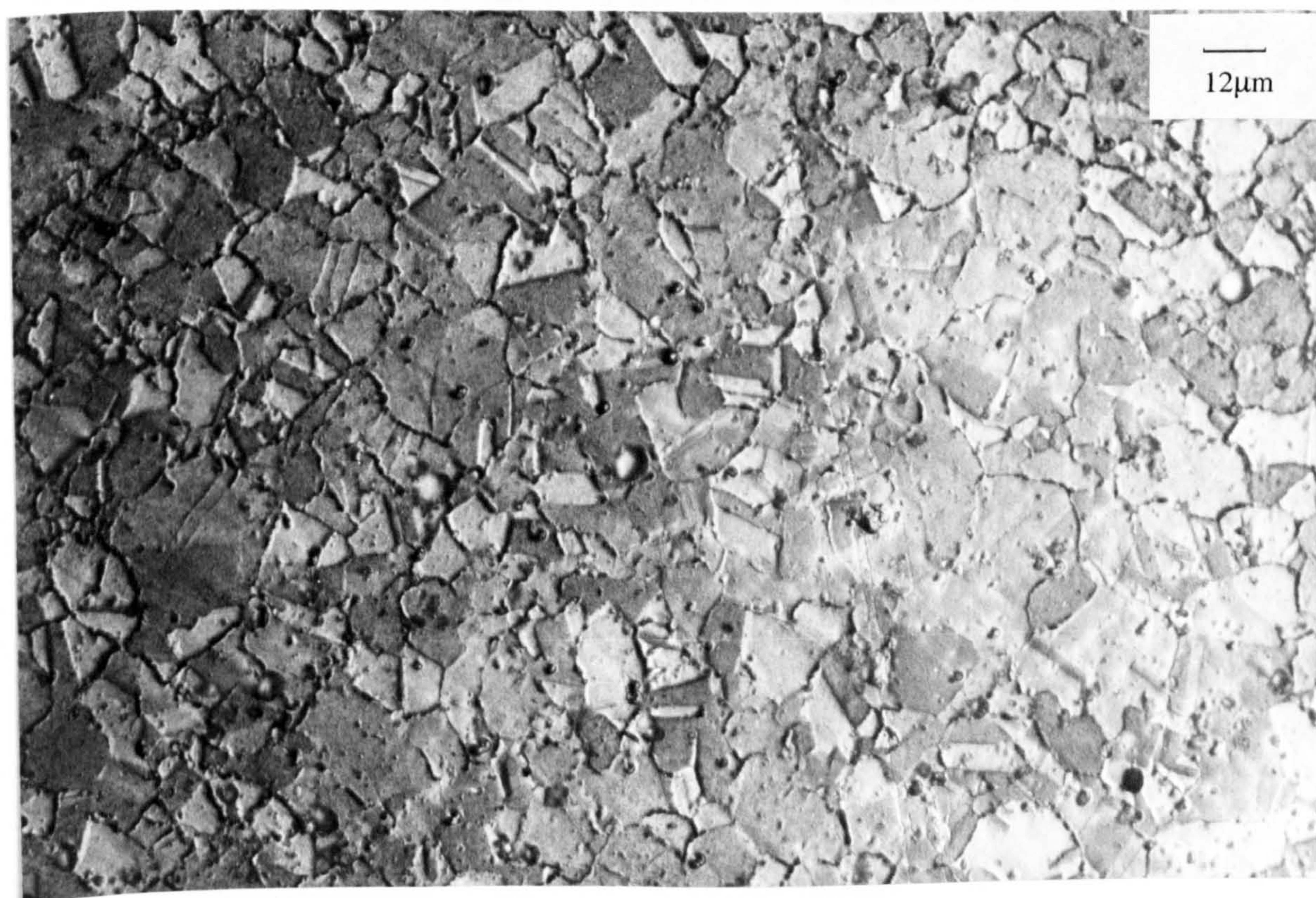
Figure 6.105. Marinel, V=86\text{m/s} , 8 hours, T.W.L. Intense pitting attack underneath the thick film outside the central zone.
