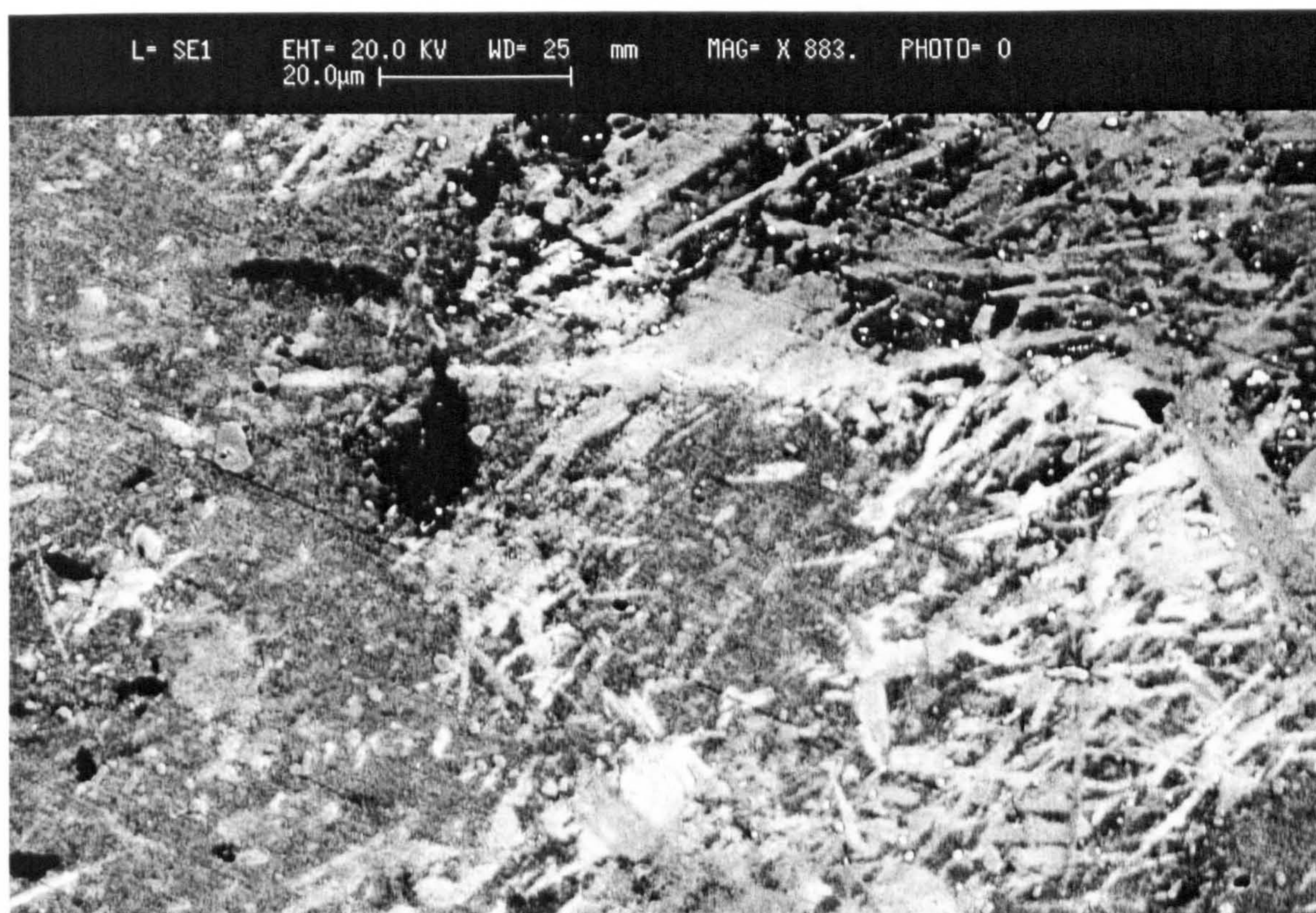
Figure 6.76. Marinel, V=17m/s, 4 hours, T.W.L. At the centre some white acicular features, which represent another film.
