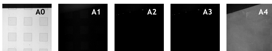
Figure 5.3(a) Fluorescence images of the SU-8 pattern on Si/SiO 2 substrate taken by optical microscope with FITC filter. (A0) Bright field image of SU-8 pattern (square) on the SiO 2 substrate, (A1) O 2 plasma and H 2 SO 4 ; (A2) O 2 plasma, H 2 SO 4 and APTES 99%; (A3) O 2 plasma, H 2 SO 4 , APTES 99% and NHS-biotin incubation; (A4) O 2 plasma, H 2 SO 4 , APTES 99%, NHS-biotin and streptavidin-FITC incubation.
