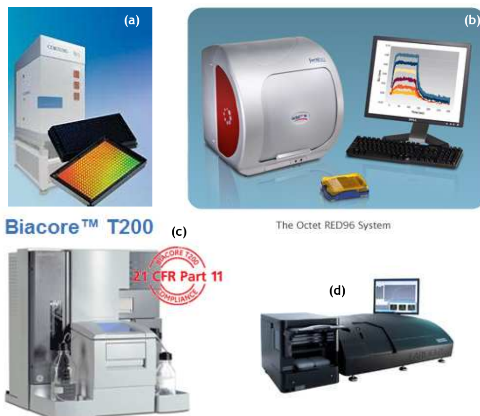
Figure 1.2: Commercial optical biosensors with different type of sensing method. (a) Epic® (Corning Inc, USA), the operating principle is based on refractive index waveguide surface to measure response the cellular signal of transduction (genetics) process; (b) Octet RED96® (ForteBio Inc, USA); (c) Biacore T200 (GE Healthcare, USA) measuring kinetic and affinity system using the SPR method and (d) AnaLight® System (Farfield Group Ltd, UK) analysing lipid and protein interaction using a planar waveguide platform.
