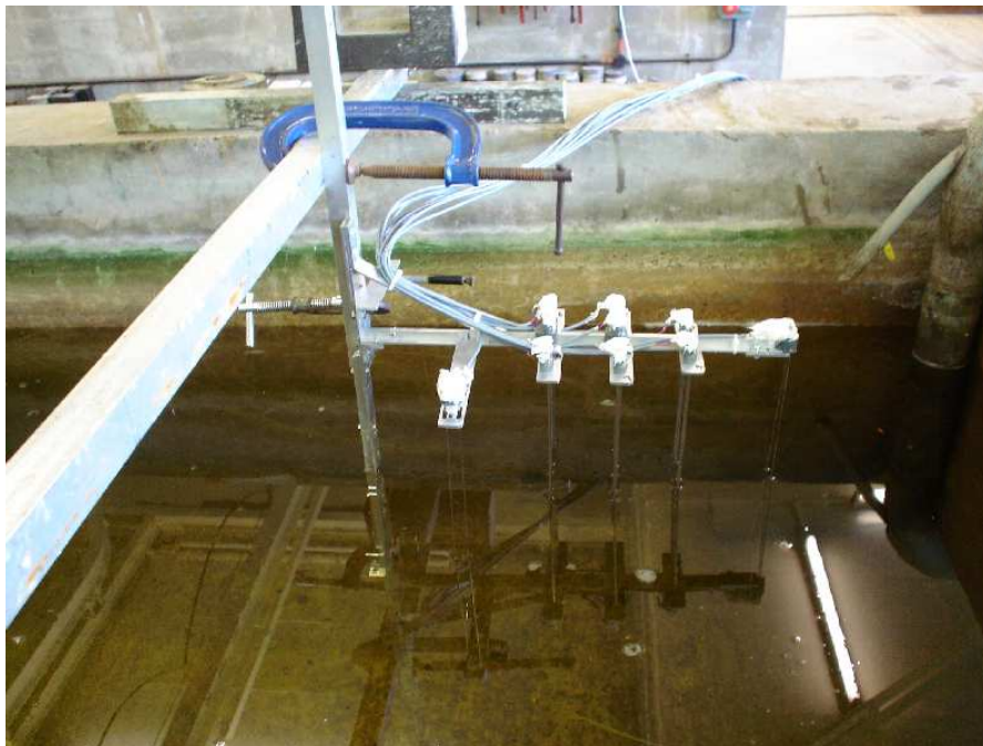
Figure 4.7.2 Calibration of wave probes that were fitted to bow section.
