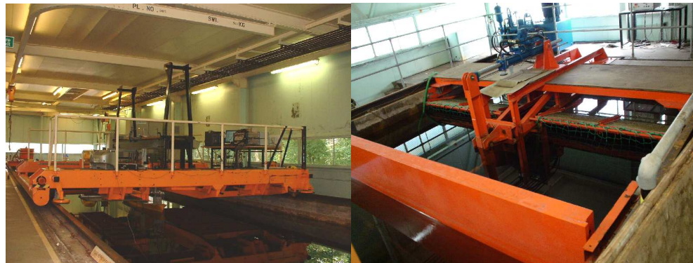
Figure 4.3.2 Snapshots of towing tank with the mobile carriage and hinged flap wave maker.
