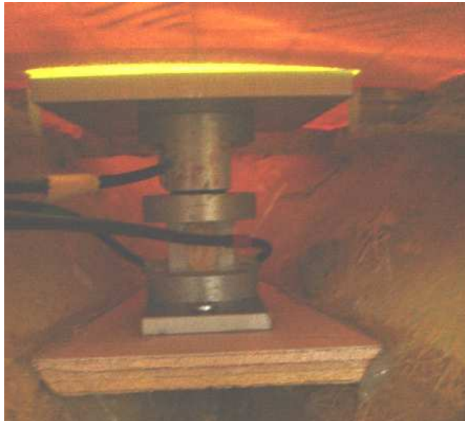
Figure 4.5.7 Deck load cell unit located under forecastle deck.
