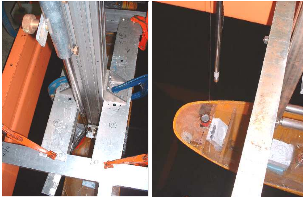
Figure 4.5.2 LVDT's to measure ship motions, one at LCG (left) and another at aft perpendicular (right).
