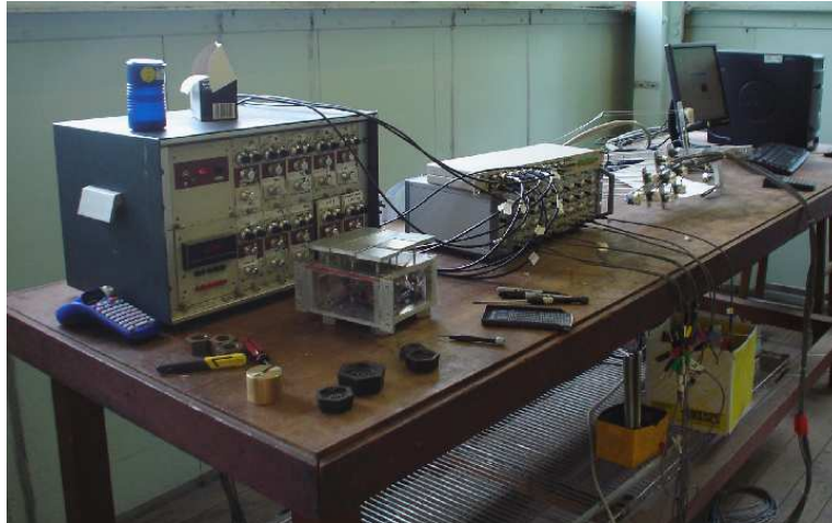
Figure 4.7.3 Calibration of vertical load cells.
