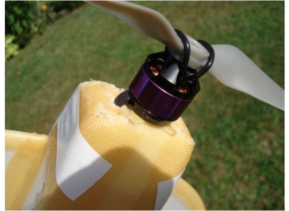
Figure 55 - Front fuselage detail with Kevlar reinforcement
