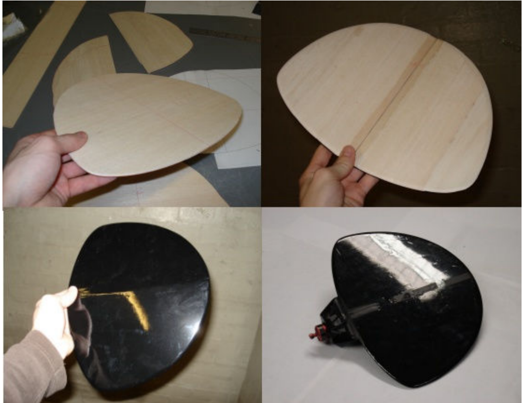
Figure 18 - Wind tunnel test model manufacturing
