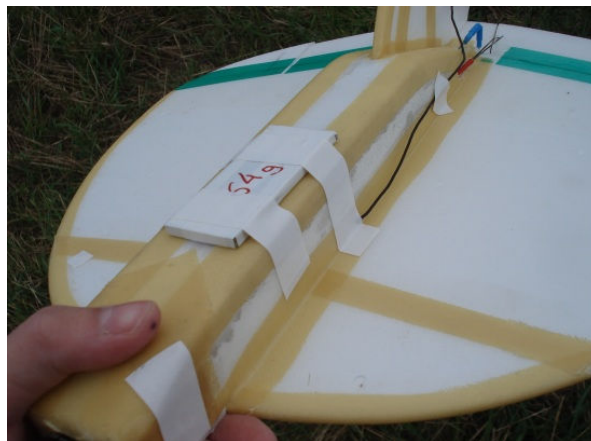
Figure 60 - Ballast (half equipment weight) attached to the MAV's belly.
