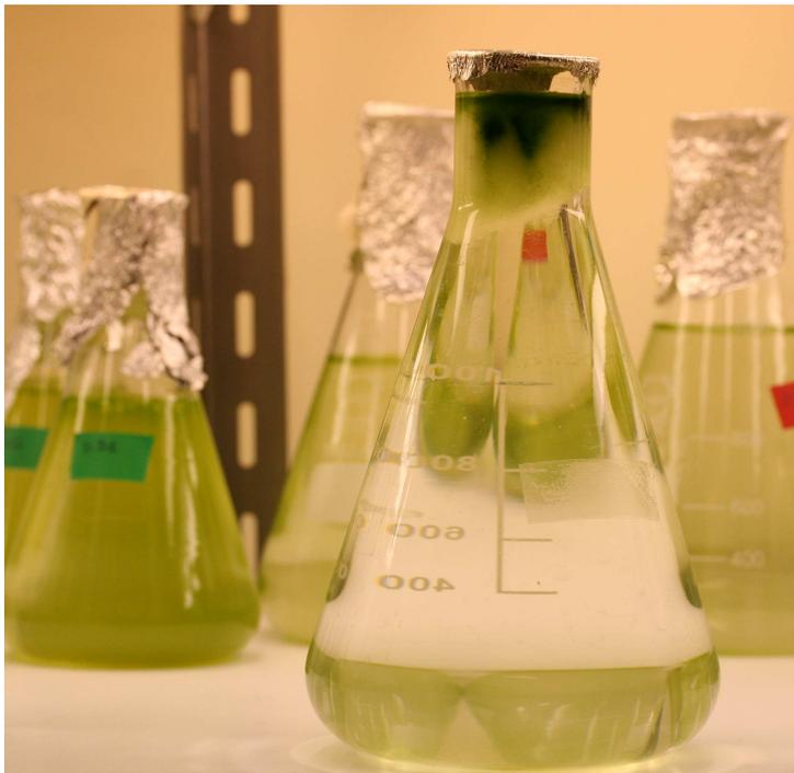
(b) Final stage of cells concentration procedure as the same conical flask after 4 days shows millions of cells trapped in cotton wool bung which turns green.
