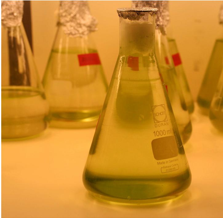
(a) Initial stage of cells concentration procedure as initially no cells accumulation in white cotton wool bung held at the top of long neck of conical flask.
