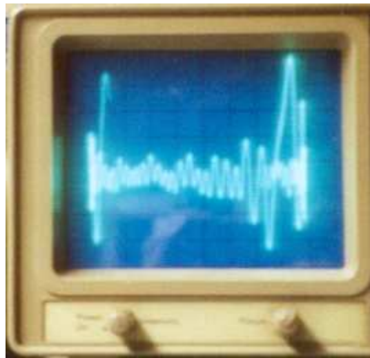
Figure 8.6. Interferometric fringes on the oscilloscope display.
