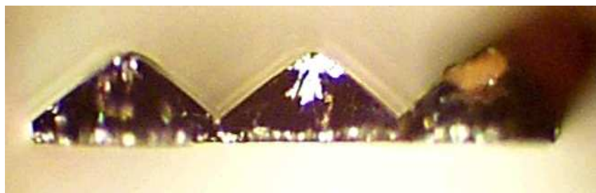
Figure 7.10. Profile of etched cleavage pits in a test sample as seen in an optical microscope.
